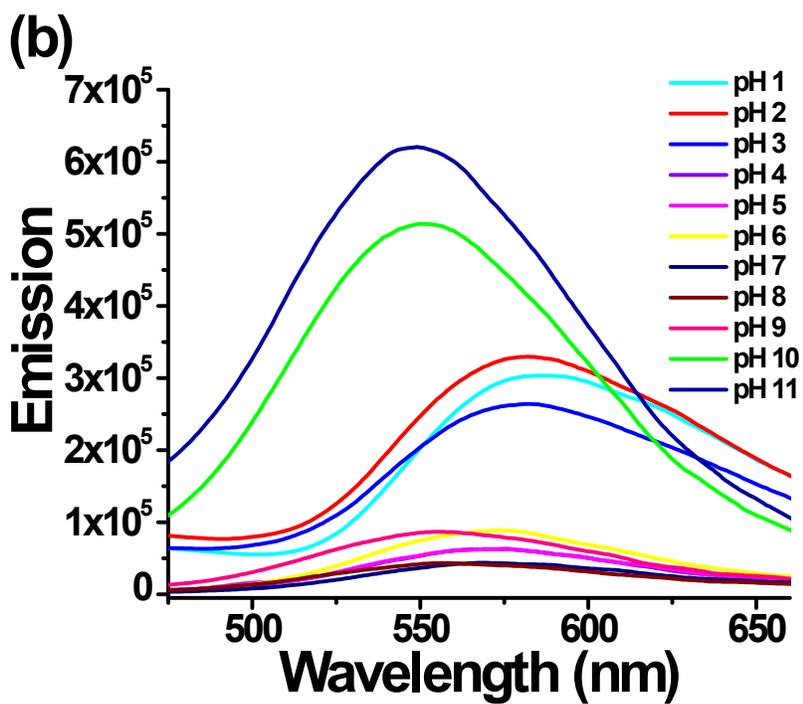
Figure S18. Absorbance (a) and emission (b) of probe 2 in different aqueous pH solutions at room temperature. Excitation at 450 nm.
