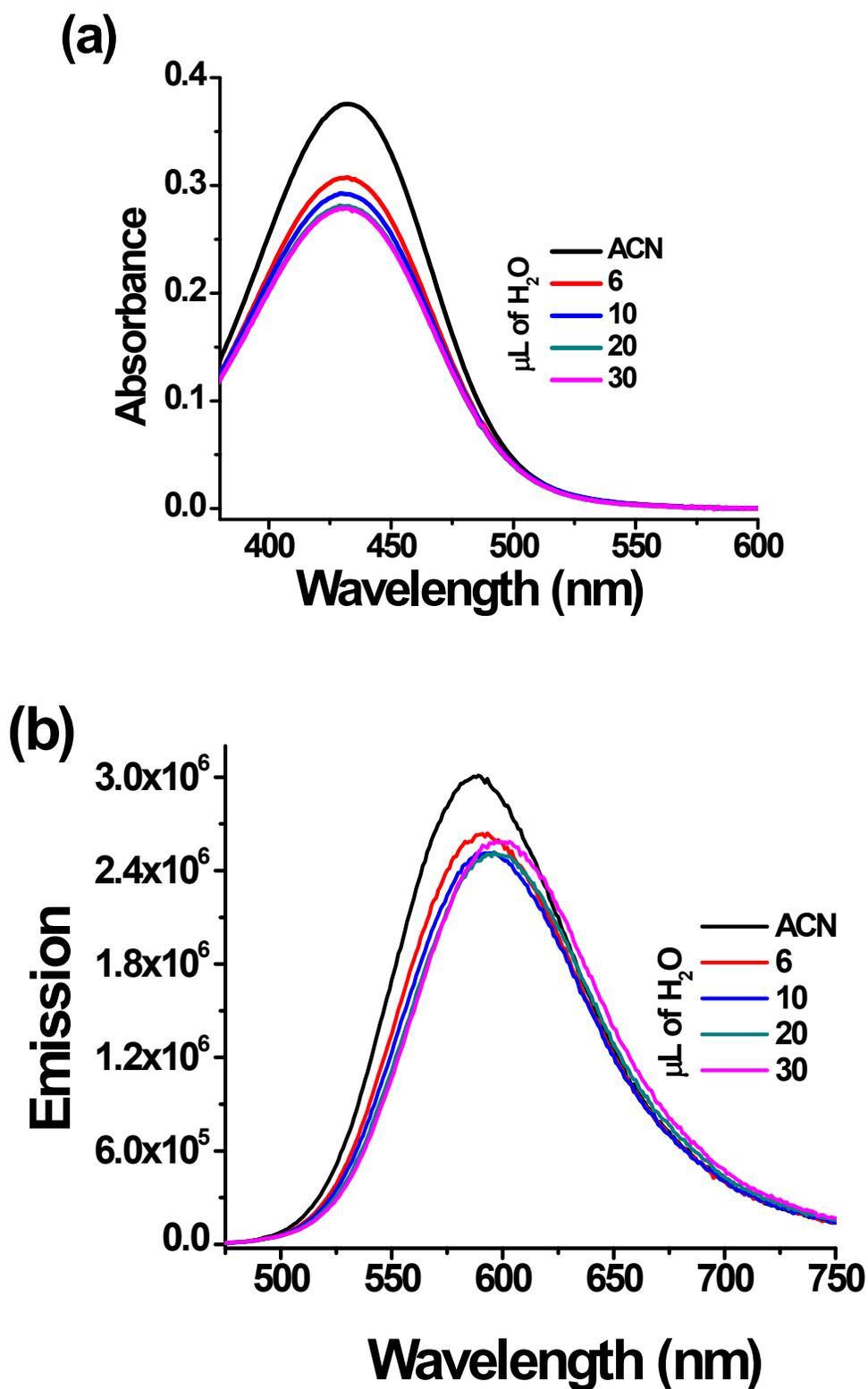
**Figure S14.** Absorbance (a) fluorescence (b) spectra obtained for probe 2 ( $1 \times 10^{-5}$  M) in acetonitrile at room temperature upon addition of different amounts of water. Probe 2 was excited at 430 nm to obtain the emission spectra.
