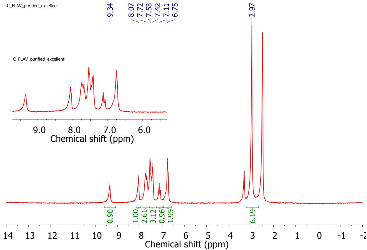
**Figure S1.1**  $^1\text{H}$  NMR spectra of **2** in DMSO- $d_6$  (300 MHz). The response signals at 2.5 ppm and 3.3 ppm attributed to DMSO and water respectively.
