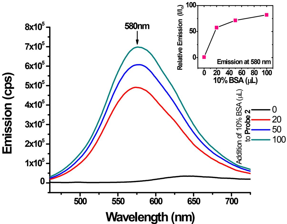
**Figure S13.** Fluorescence emission spectra obtained for probe 2 ( $1 \times 10^{-5}$  M in water) upon addition of different amounts of 10% (w/v) BSA in water. Probe 2 was excited at 435 nm to obtain the emission spectra
