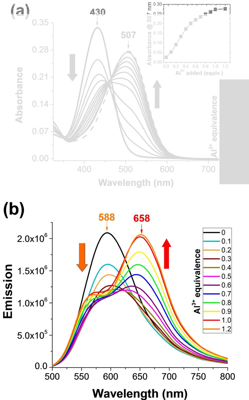
**Figure S5.** Absorption (a) and emission (b) recorded for probe 2 ( $1 \times 10^{-5}$  M) in acetonitrile upon spectrometric titration with  $\text{Al}^{3+}$  (1 mM in water) at room temperature. Sample was excited at 465 nm to obtain emission spectra.
