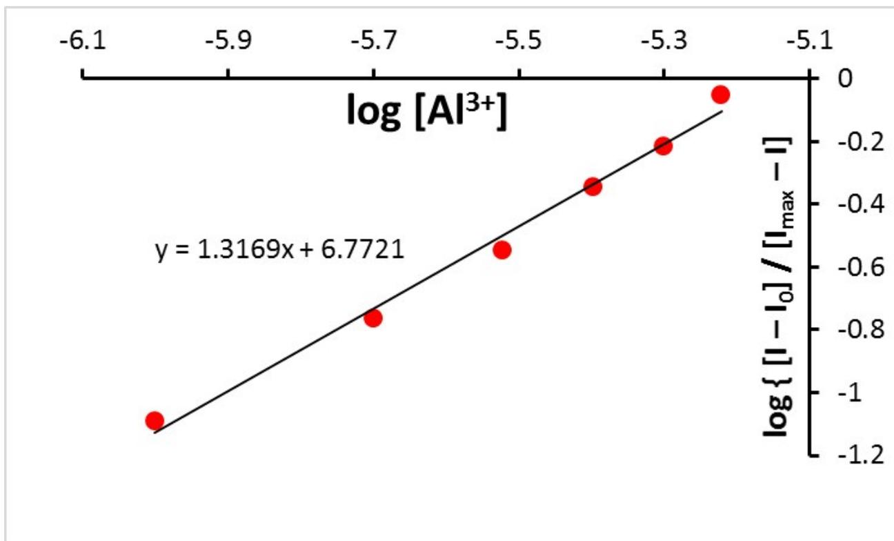
**Figure S9.** Determination of the binding constant ( $\log K$ ) for **2-Al** complex by using emission data obtained during spectrometric titration of probe **2** with  $Al^{3+}$ .
