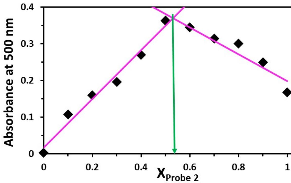
Figure S8. Determination of the probe 2: Al<sup>3+</sup> binding stoichiometry by Job's method.
