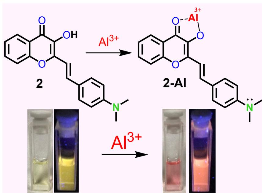
**Figure S10.** Visible and UV illuminated color observed for probe 2 before (left) and after (right) the addition of  $\text{Al}^{3+}$  (1.0 equiv.) in acetonitrile at room temperature.
