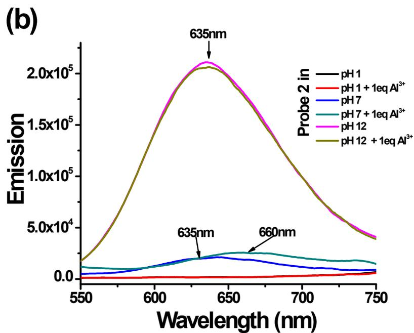
**Figure S20.** Absorbance (a) and emission (b) of probe **2** and probe **2+Al** complex in different aqueous pH solutions at room temperature.
