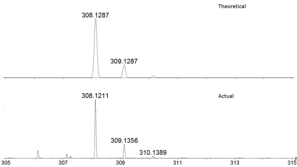
**Figure S2.** High resolution mass spectra (ESI) of [2-H]<sup>+</sup>. (Error < 3ppm)
