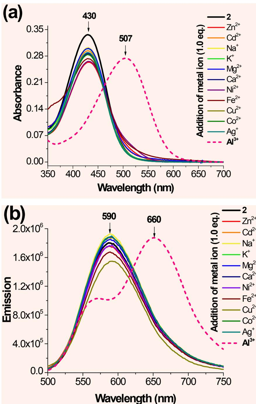
**Figure S11.** Absorption (a) and emission (b) recorded for probe **2** ( $1 \times 10^{-5}$  M) in acetonitrile upon addition of 1 eq. of cationic species (1 mM in water) at room temperature. Only **2-Al** complex was excited at 465 nm and all other samples were excited at 430 nm.
