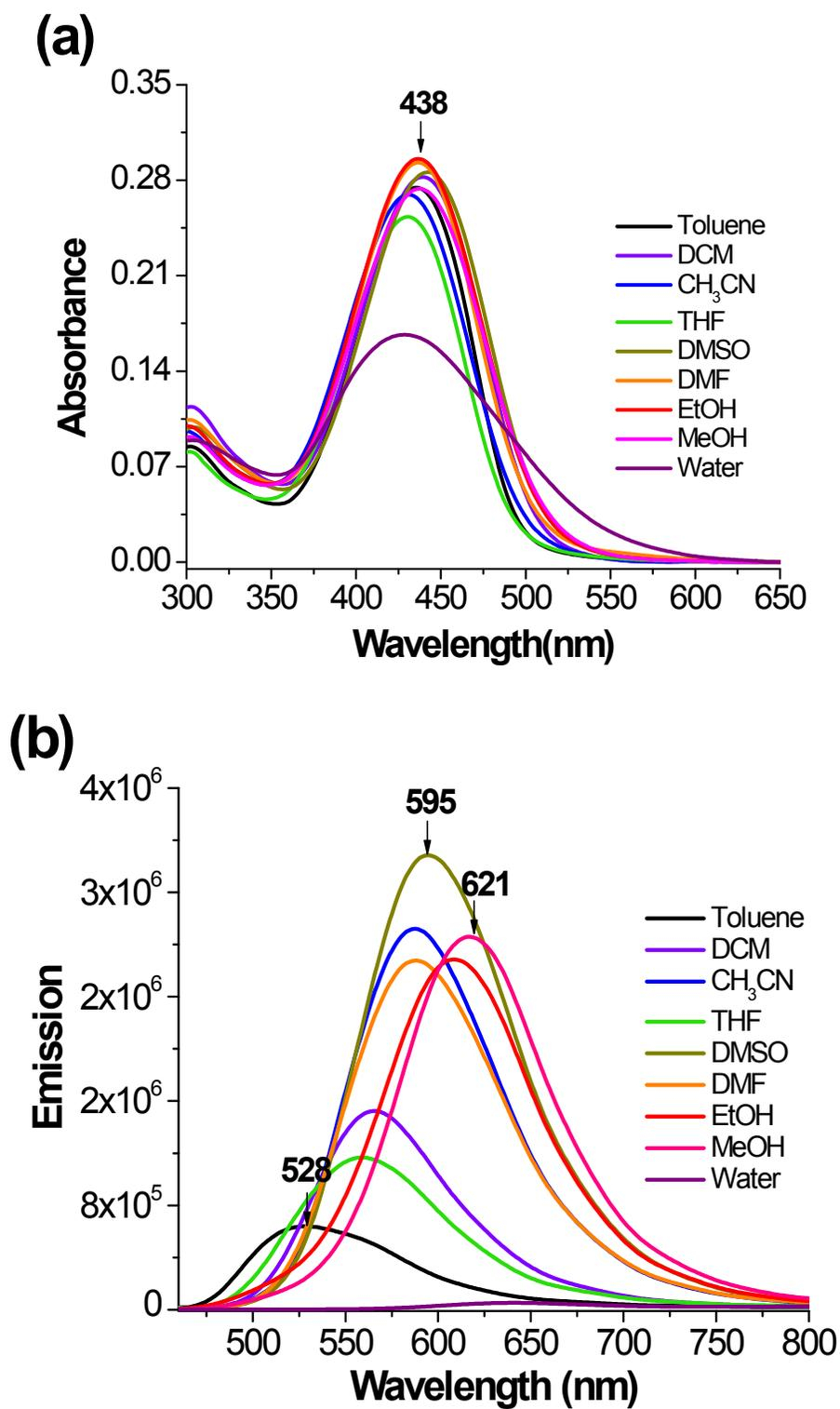
**Figure S3.** Absorption (a) and emission (b) of probe **2** ( $1 \times 10^{-5}$  M) in different solvents at room temperature.
