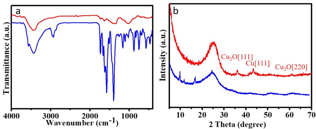
**Figure S19.** The (a)IR spectra and (b) XRD patterns of CuBDC@CF before (blue) and after (red) catalytic test.
