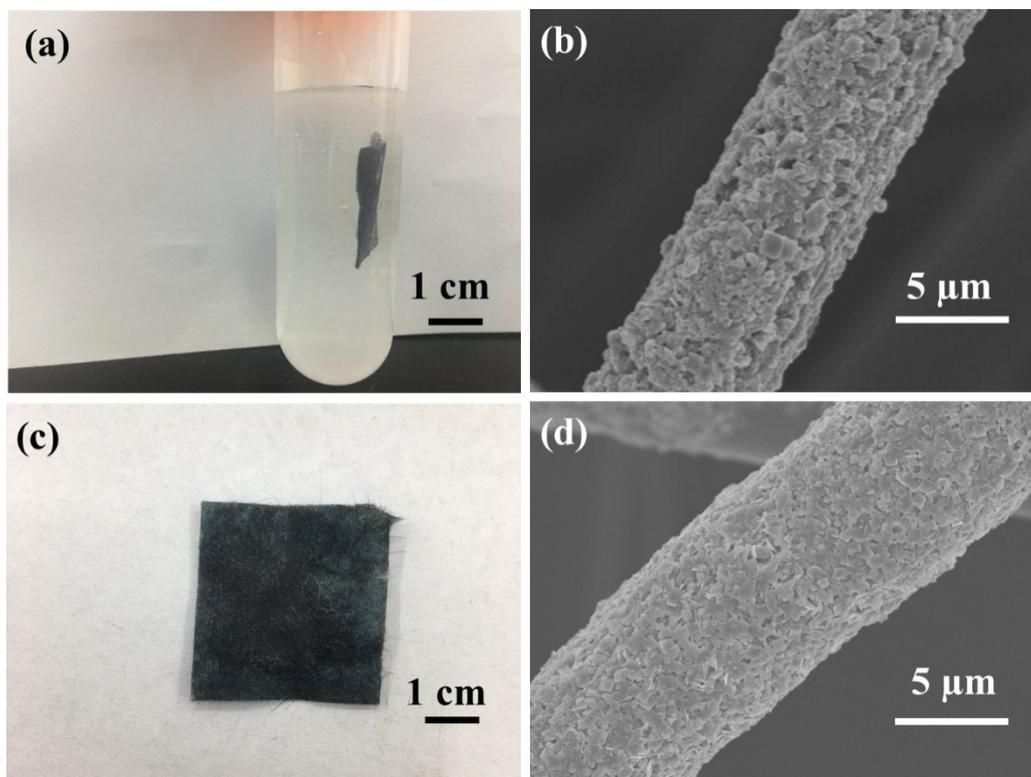
**Figure S4.** The photographs of CuBDC@CF after (a) shaking in DMF and (c) rubbing; the SEM images of CuBDC@CF after (b) shaking in DMF and (d) rubbing.
