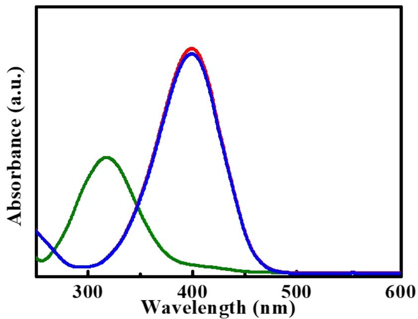
**Figure S14.** The UV-Vis absorption spectra of 4-NP without NaBH<sub>4</sub> (green), reaction mixture (red), reaction mixture for 10 h (blue).
