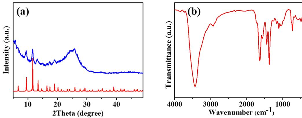
**Figure S12.** The (a) simulated XRD pattern of HKUST (red), XRD pattern of HKUST@CF (blue) and (b) IR spectrum of HKUST@CF.
