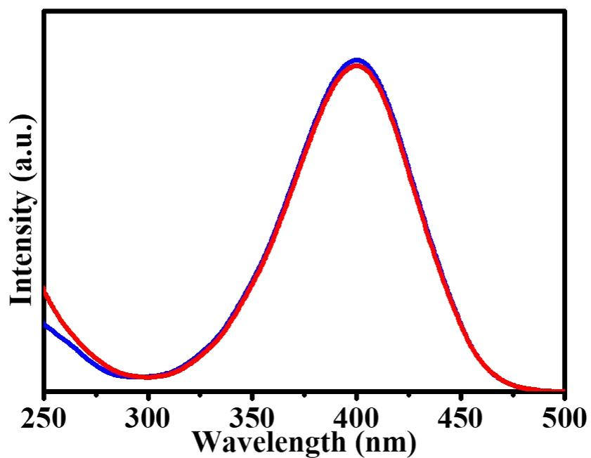
**Figure S21.** UV-Vis absorption spectra of the reaction mixture (blue), effluent collected through CFs (red).
