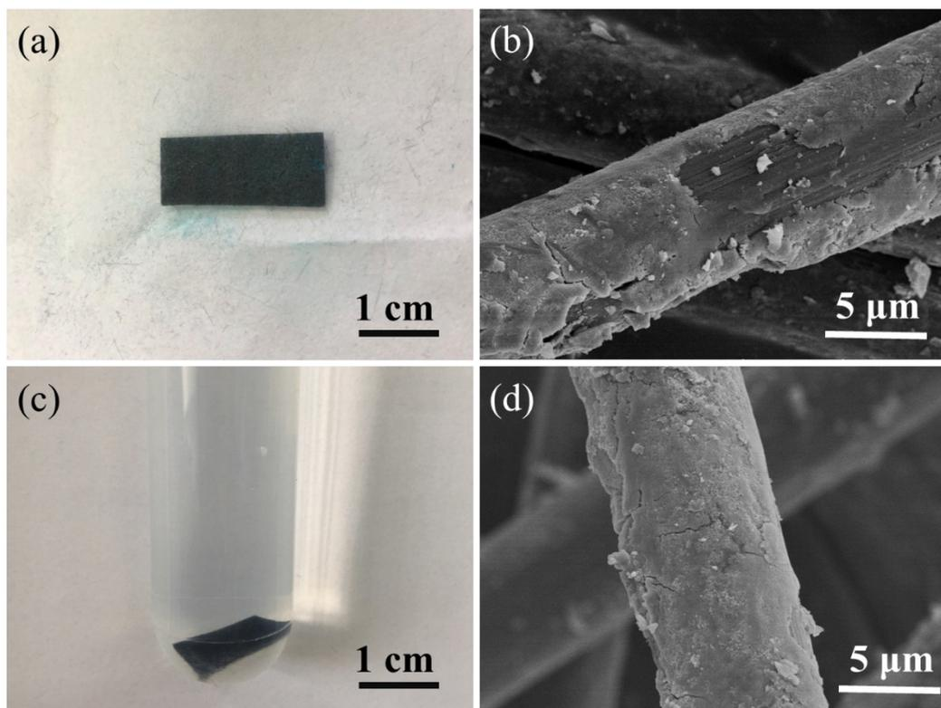
**Figure S13.** The photographs of HKUST@CF after (a) rubbing and (c) shaking in DMF; the SEM images of HKUST@CF after (b) rubbing and (d) shaking in DMF.
