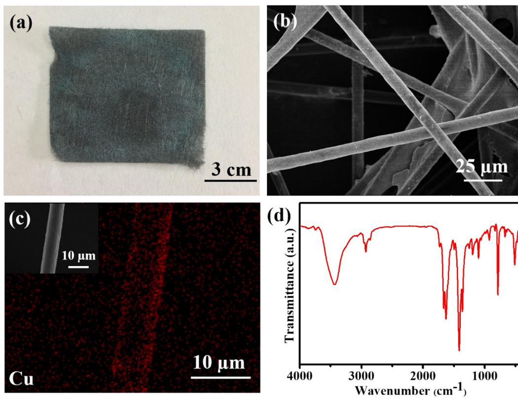
**Figure S9.** The (a) photograph, (b) SEM image, (c) EDS elemental mapping image and corresponding SEM image (insert), (d) FT-IR spectrum of Cu(2,6-NDC)@CF.
