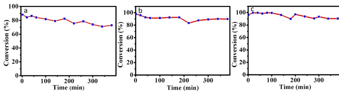
**Figure S22.** The conversion rate of 4-NP reduction by (a) Cu(1,4-NDC)@CF, (b) Cu(2,6-NDC)@CF and (c) Cu(2-atp)@CF.
