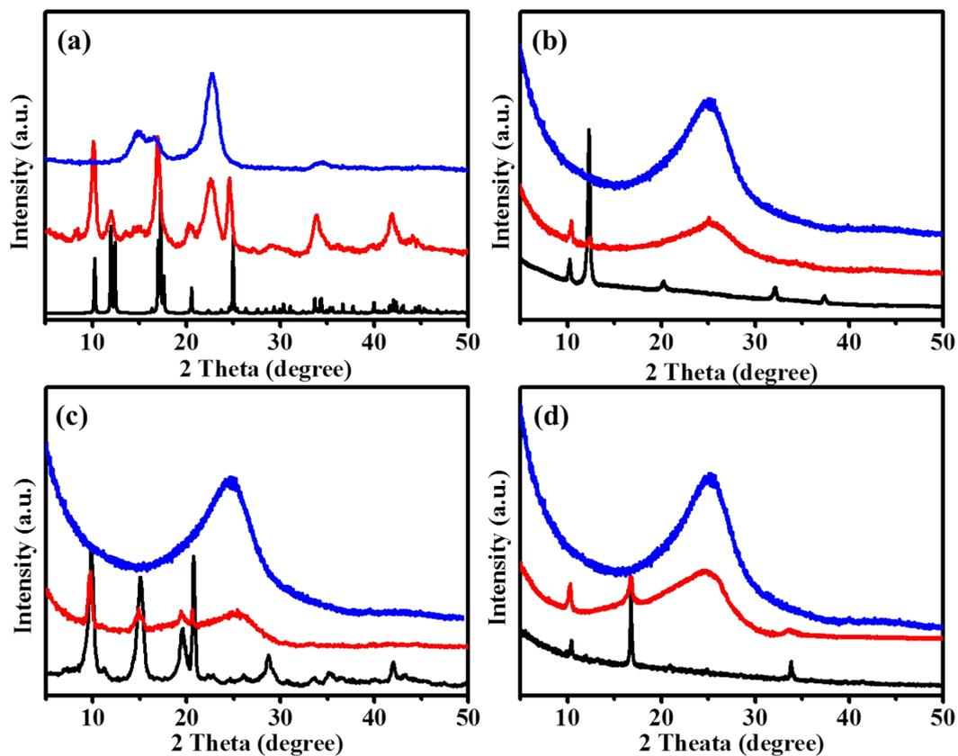
**Figure S7.** The XRD patterns of (a) CuBDC (black), CuBDC@cotton fiber (red) and cotton fibers (blue); (b) Cu(1,4-NDC) (black), Cu(1,4-NDC)@CF (red) and CFs (blue); (c) Cu(2,6-NDC) (black), Cu(2,6-NDC)@CF (red) and CFs (blue); (d) Cu(2-atp) (black), Cu(2-atp)@CF (red) and CFs (blue).
