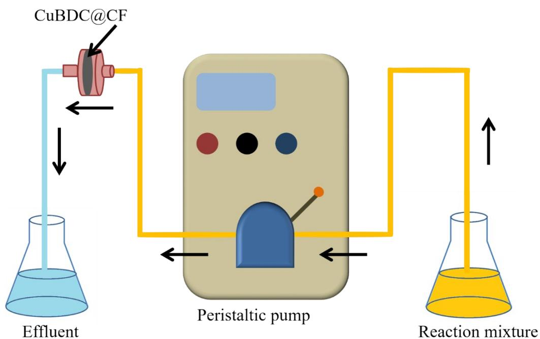
**Figure S20.** The schematic diagram of filtration system.
