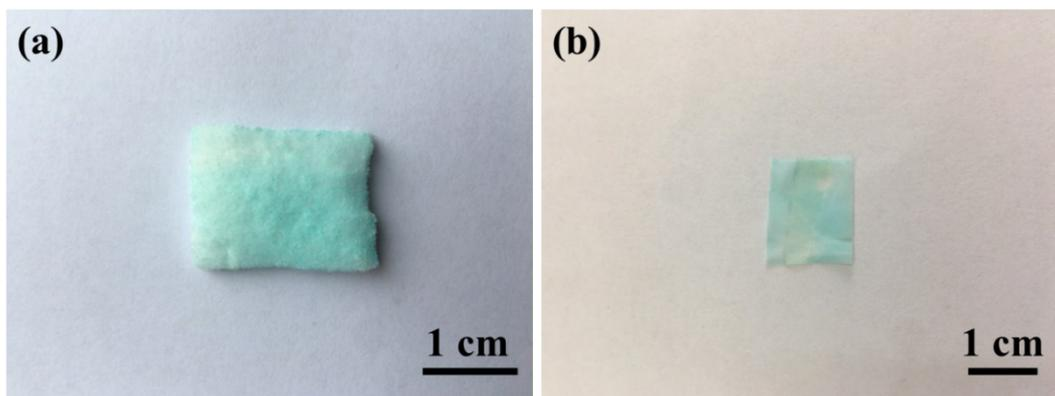
**Figure S5.** The photographs of (a) CuBDC@cotton fiber and (b) CuBDC@nylon fiber.
