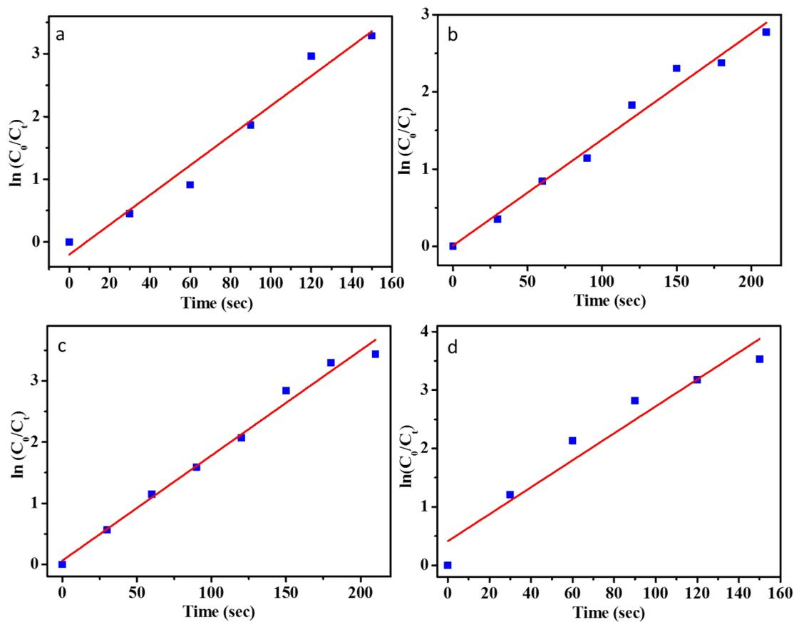
**Figure S17.** Plots of  $\ln(c_0/c_t)$  versus reaction time for the 4-NP reduction with (a) CuBDC@CF, (b) Cu(1,4-NDC)@CF, (c) Cu(2,6-NDC)@CF and (d) Cu(2-atp)@CF.
