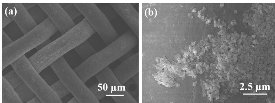
**Figure S6.** The SEM images of CuBDC@nylon fiber.
