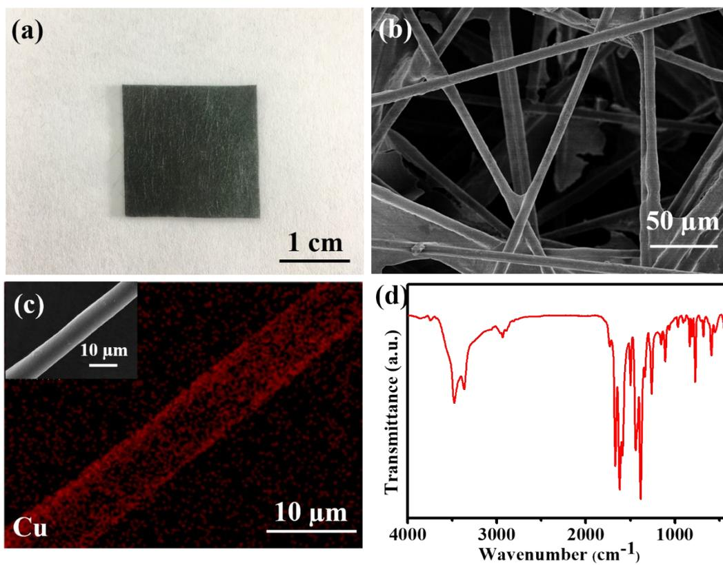
**Figure S10.** The (a) photograph, (b) SEM image, (c) EDS elemental mapping image and corresponding SEM image (insert), (d) FT-IR spectrum of Cu(2-atp)@CF.
