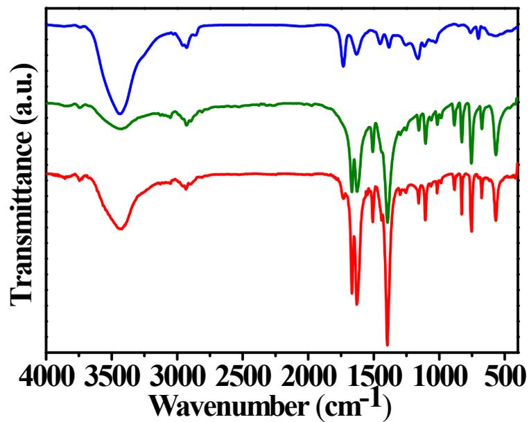
**Figure S3.** FT-IR spectra of CFs (blue), CuBDC@CF (red) and CuBDC (green) with larger wavenumber region.
