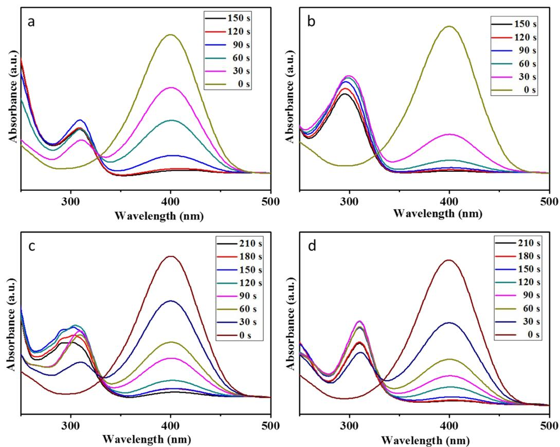
**Figure S16.** UV-Vis absorption spectra of the 4-NP reduction versus reaction time under the catalysis of (a) CuBDC@CF, (b) Cu(1,4-NDC)@CF, (c) Cu(2,6-NDC)@CF and (d) Cu(2-atp)@CF.
