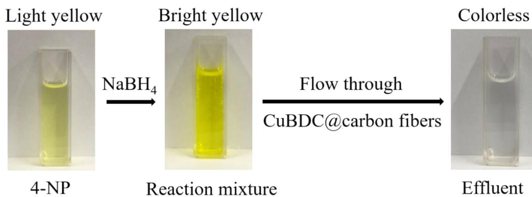
**Figure S15.** The photographs of 4-NP solution, reaction mixture solution and effluent solution (4-AP).
