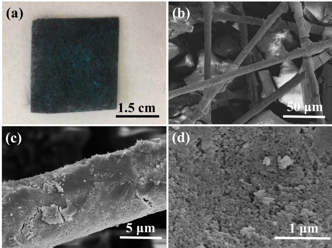
**Figure S11.** The (a) photograph and (b-d) SEM images of HKUST@CF prepared by spraying technique.
