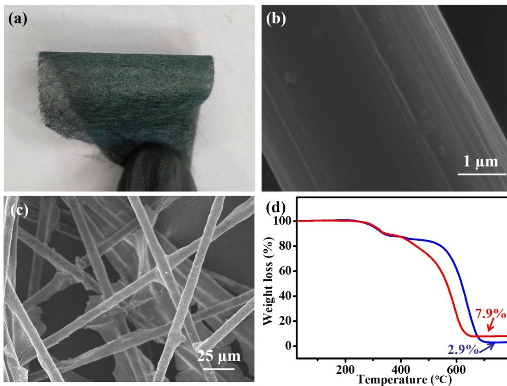
**Figure S1.** (a) The photograph of CuBDC@CF, the SEM images of (b) CFs and (c) CuBDC@CF, (d) the TGA curves of CFs (blue) and CuBDC@CF (red).
