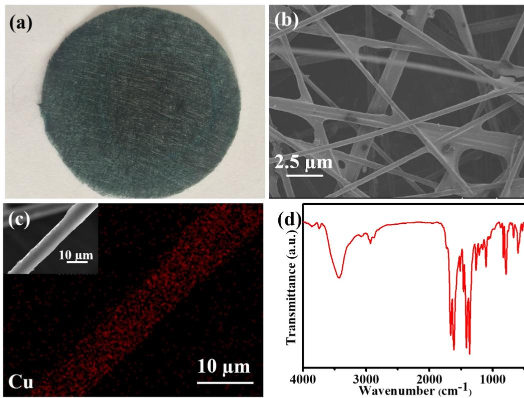
**Figure S8.** The (a) photograph, (b) SEM image, (c) EDS elemental mapping image and corresponding SEM image (insert), (d) FT-IR spectrum of Cu(1,4-NDC)@CF.
