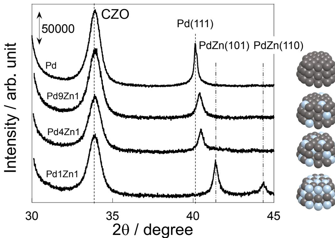
**Figure S1.** XRD patterns of Pd-Zn alloy supported on CZO with various Pd/Zn ratios: Pd loading amount, 5wt%.
