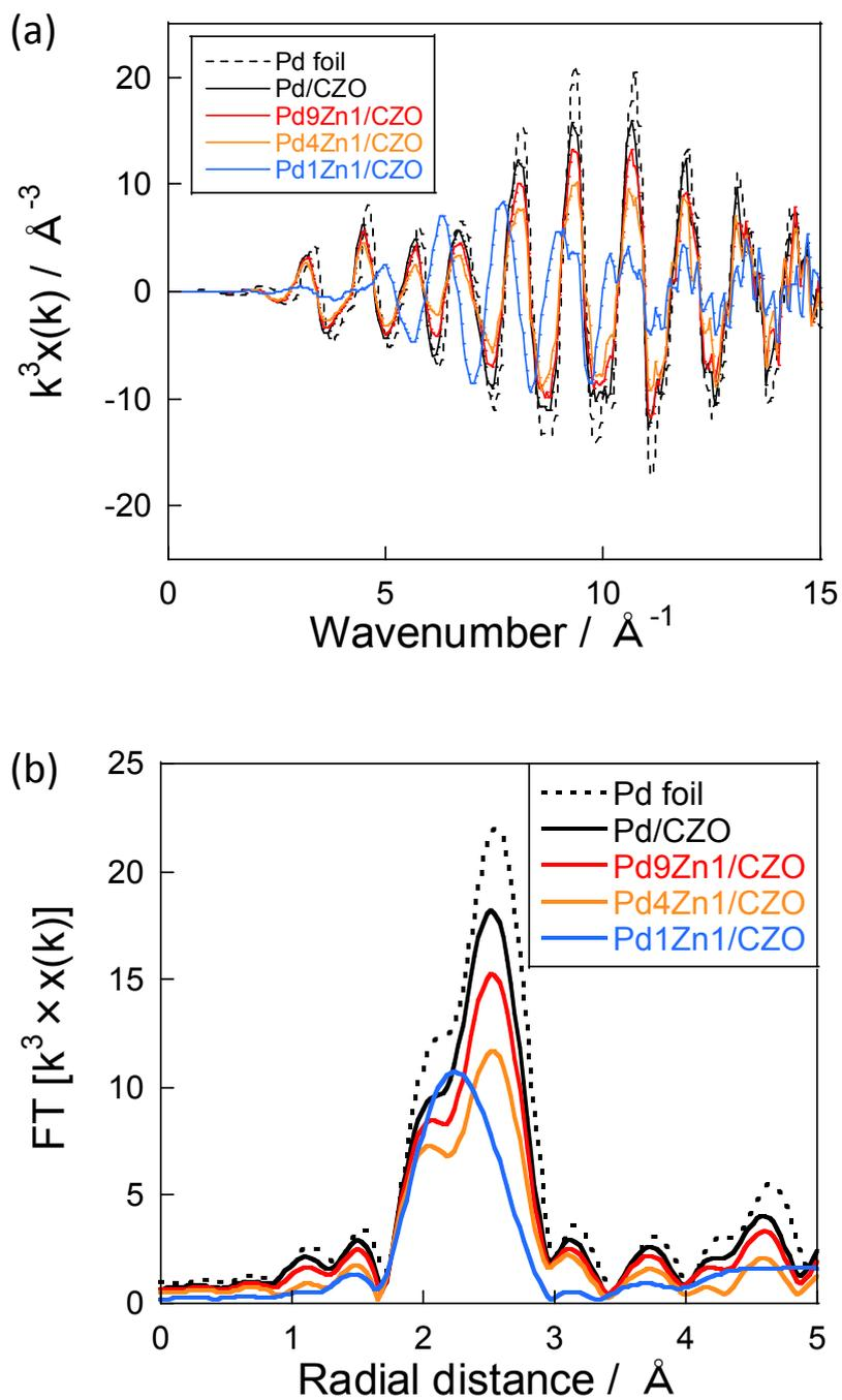
**Figure S2.** (a)  $k^3$ -weighted and (b) Fourier-transformed Pd K-edge EXAFS spectra of Pd-Zn/CZO catalysts: Pd loading amount, 5 wt%.
