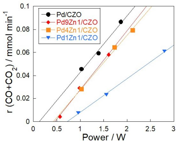
**Figure S5.** Input power dependence of the catalytic activity with an electric field over 5wt%Pd–Zn/CZO with various Zn/Pd ratios: Reactant gas, CH<sub>4</sub>:H<sub>2</sub>O:Ar = 1:2:7, total flow rate 100 SCCM; furnace temperature, 423 K; input current, 3-7 mA.
