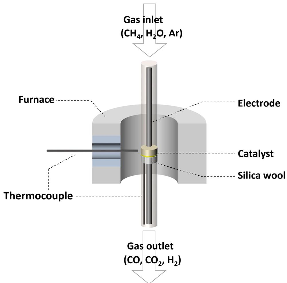
**Figure S3.** Schematic diagram of reactor.
