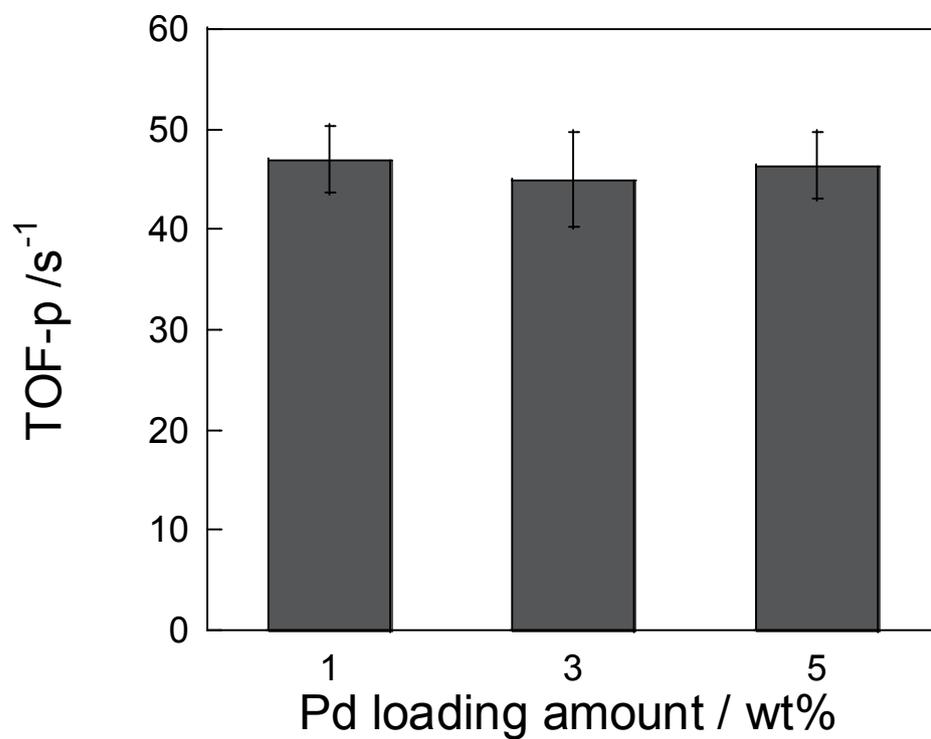
**Figure S4** Effects of Pd loading amount of Pd1Zn1/CZO on turnover frequency calculated based on Pd perimeter (TOF-p) in an electric field: Reactant gas, CH<sub>4</sub>:H<sub>2</sub>O:Ar = 1:2:7, total flow rate 100 SCCM; furnace temperature, 423 K; input power, 1.5 W.
