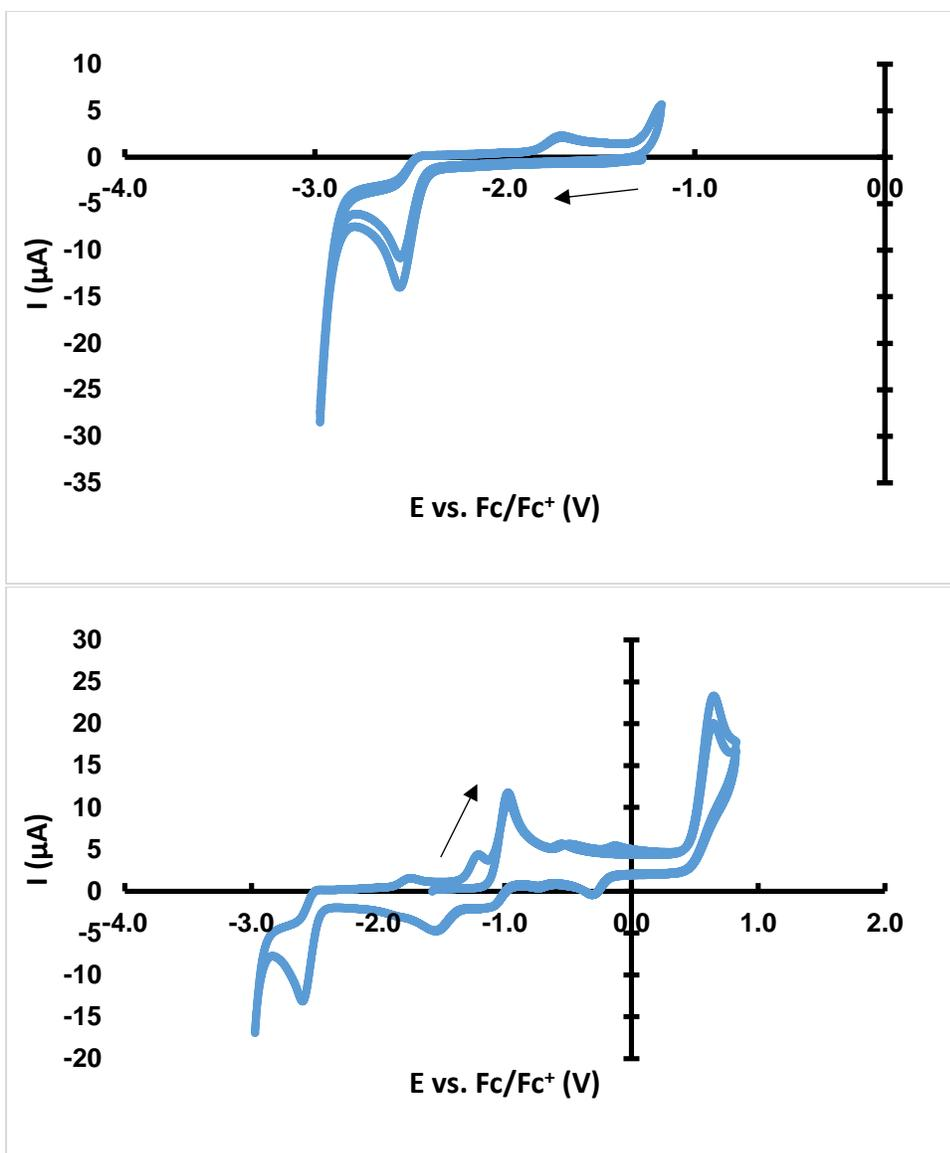
**Details:** The arrow indicates the initial potential and scanning direction. The scan rate was 100 mV/s, and two complete cycles are displayed on each voltammogram. They show two irreversible oxidations at -0.952 and 0.667 V. There is also one irreversible reduction at -2.55 V. The oxidations give rise to reductions at -0.289 and -1.51 V.
