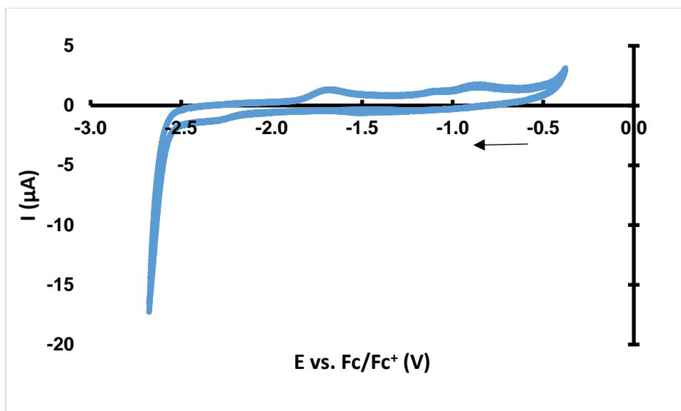
**Details:** The arrow indicates the initial potential and scanning direction. The scan rate was 100 mV/s, and two complete cycles are displayed on each voltammogram. They show two irreversible oxidations at -0.32 and 0.60 V. No reduction events are observed. The oxidations give rise to reductions at 0.90, -1.50, and -2.41 V.
