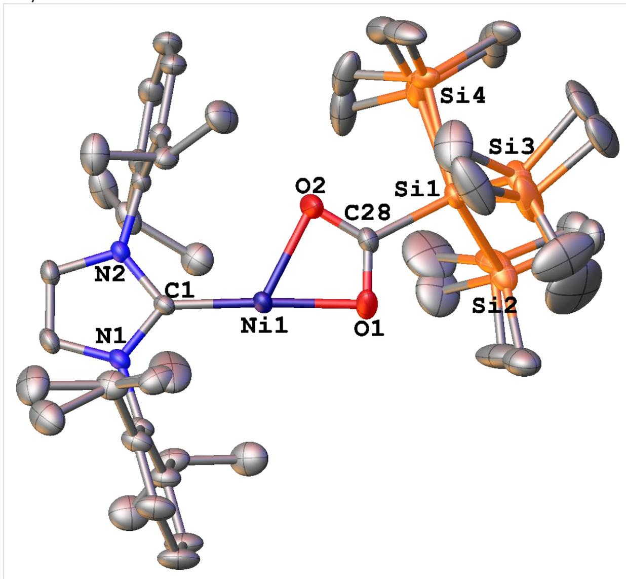
**Details:** Hydrogens have been eliminated for clarity and ellipsoids were set at 50% probability. The rotational disorder about  $-\text{Si}(\text{SiMe}_3)_3$  and an isopropyl group have been modelled appropriately. Selected bond lengths [Å] and angles [°]: Ni1—O1 = 1.978(1), Ni1—O2 = 2.078(1), Ni1—C28 = 2.361(1), Ni1—C1 = 1.872(1), C28—O1 = 1.263(1), C28—O2 = 1.252(2), C28—Si1 = 1.931(1), C1—Ni1—O1 = 174.2(1), C1—Ni1—O2 = 117.4(1), O1—Ni1—O2 = 64.1(1), O1—C28—O2 = 117.8(1).
