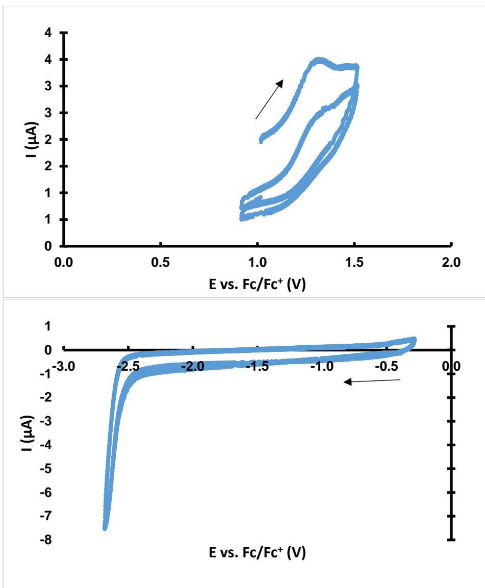
**Details:** The arrow indicates the initial potential and scanning direction. The scan rate was 100 mV/s, and two complete cycles are displayed on each voltammogram. They show two irreversible oxidations at -0.089 and 1.22 V. No reduction events are observed. The oxidations give rise to reductions at -0.040, -1.24, and -2.05 V.
