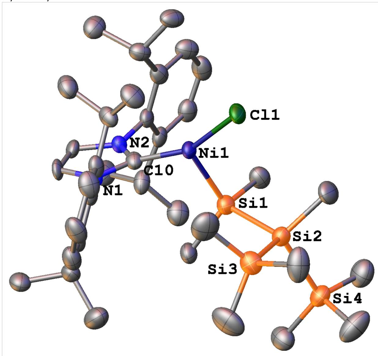
**Details:** Hydrogens have been eliminated for clarity and ellipsoids were set at 50% probability. Selected bond lengths [Å] and angles [°]: Ni1—C10 = 1.850(7), Ni1—Si1 = 2.231(3), Ni1—Cl1 = 2.129(1), C10—Ni1—Si1 = 94.5(3), Si1—Ni1—Cl1 = 107.9(1), Cl1—Ni1—C10 = 156.8(3).
