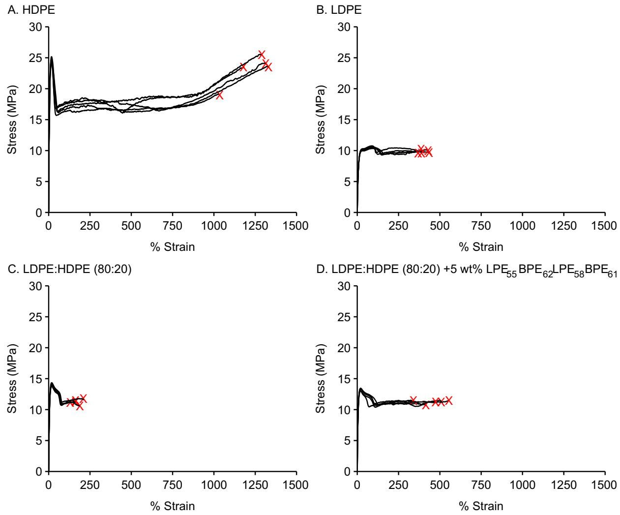
Figure S16. Compiled uniaxial tensile elongation of (A) HDPE, (B) LDPE, and (C) LDPE/HDPE blend (80:20, LDPE:HDPE). (D) Compiled tests of LDPE/HDPE blend (80:20, LDPE:HDPE) with the addition of 5 wt% tetra-block copolymer. The samples were strained at a rate of 100 % min<sup>-1</sup> at 25 °C.
