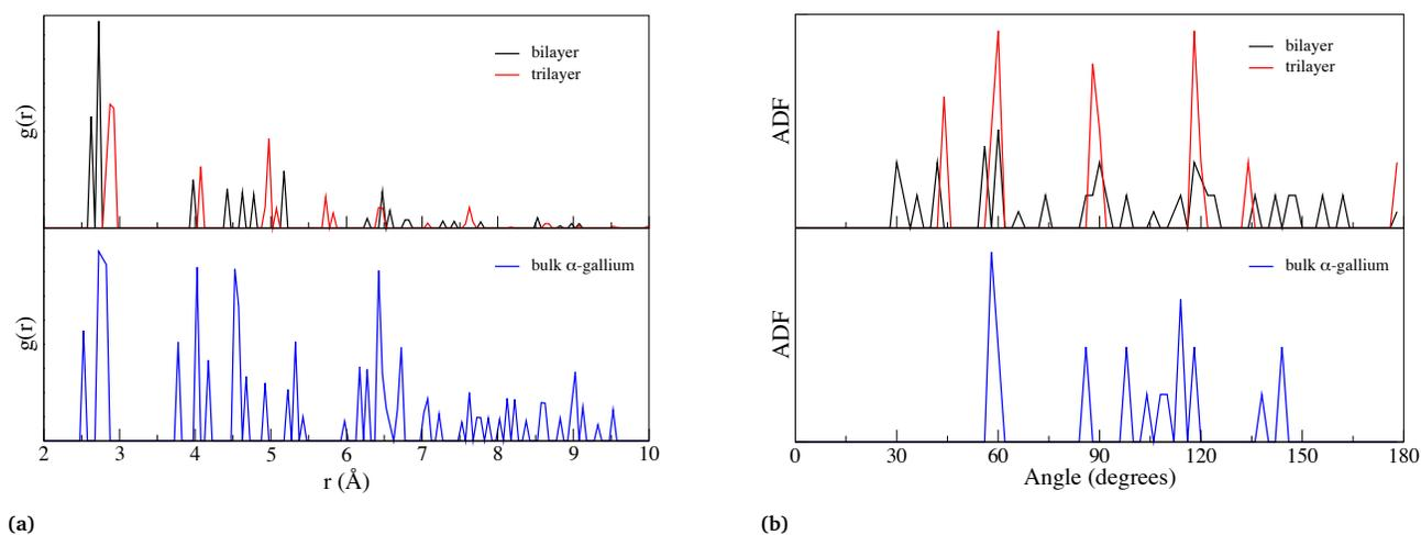
**Fig. S3** (a) Radial distribution function,  $g(r)$ , and (b) angular distribution function (ADF) for the lowest energy, optimised bilayer and trilayer structures. For the ADF, we include only the angles between atoms within the first coordination shell. For both the radial distribution function and ADF, we include an analysis of bulk  $\alpha$ -gallium optimised with the same computational settings (PBEsol, PAW) for comparison.
