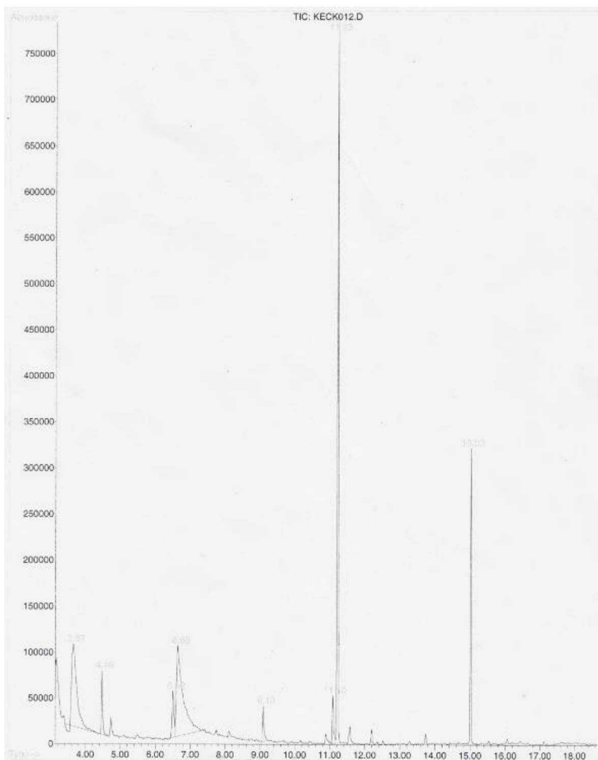
Fig S25. GC-MS measurement of compound 8 after irradiation at \lambda = 254 nm for 40 minutes in DCM.
