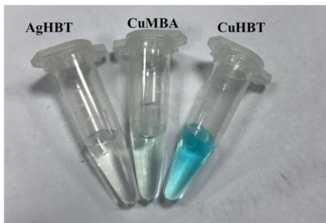
**Fig. S8.** Photographs of the compared colorimetric reactions of CuHBT, CuMBA and AgHBT.
