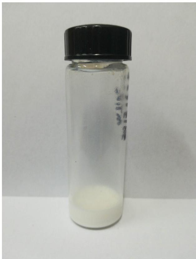
**Fig. S10.** Photograph of  $\text{TiO}_2\text{-C}_{18}\text{-PEG}$  aqueous dispersion (30 wt%) stored for 3 years.
