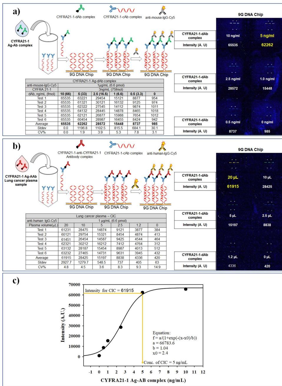
**Figure S1:** (a) CYFRA 21-1 and mouse origin anti-CYFRA 21-1 detection antibody complex detection, (b) Plasma CIC detection, (c) Standard curve using CYFRA 21-1 and mouse origin anti-CYFRA 21-1 detection antibody complex detection.
