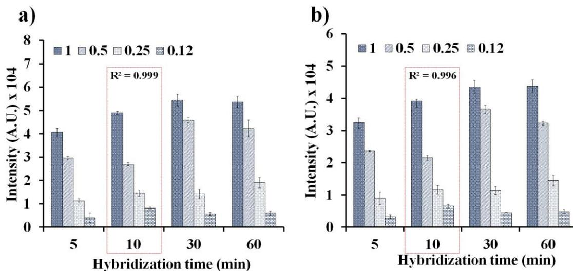
**Figure S3:** Optimization of the hybridization time required for the detection of (a) CIC and (b) CYFRA 21-1. The optimum hybridization time was considered as 10 min for both CIC and CYFRA 21-1 detection because the linearity coefficient ( $R^2$ ) for serial dilution study (dilution factors: 1.0, 0.5, 0.25, and 0.12) were 0.999 and 0.996, respectively. The original concentrations of CIC and CYFRA 21-1 were 2.7 ng/mL and 2.5 ng/mL, respectively.
