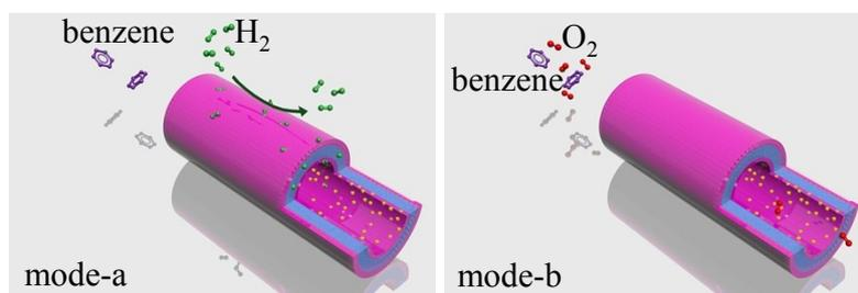
**Fig. S9** Modes of reaction scheme with Pd-TSH composite membrane.
