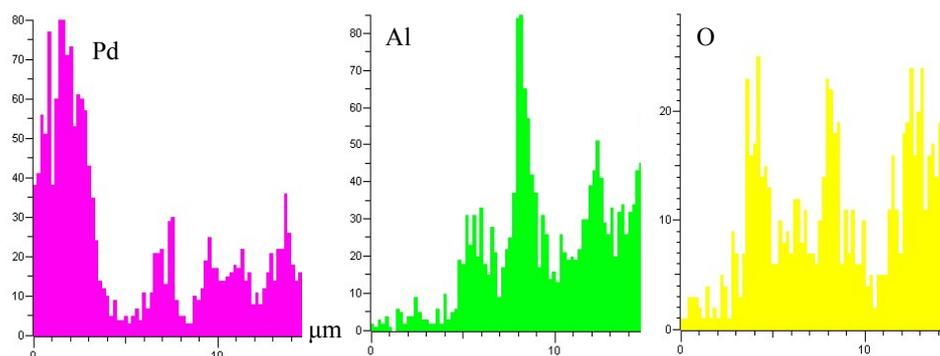
**Fig. S3** EDX analysis of Pd, Al and O.
