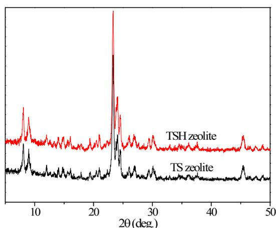
**Fig. S4** XRD patterns of TS and TSH zeolite.
