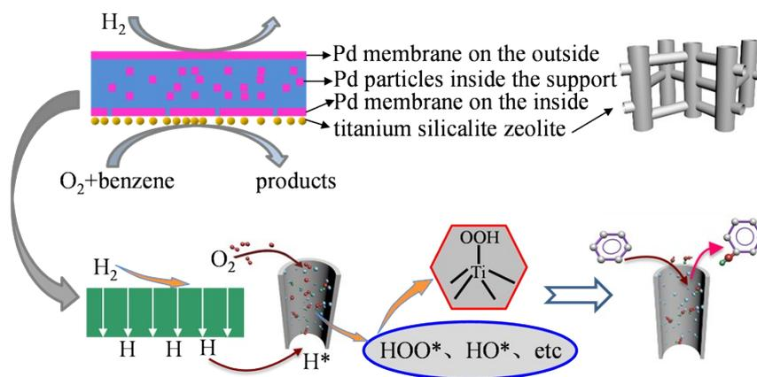
**Fig. S8** The reaction pathway in Pd-TSH composite membrane.
