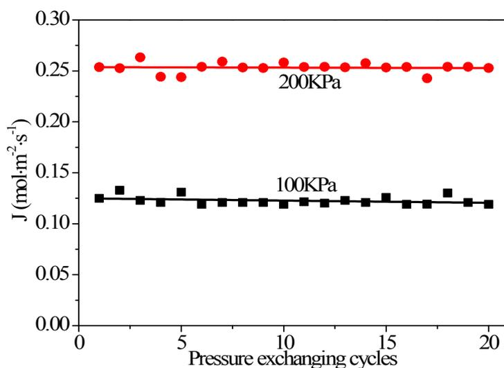
**Fig. S6** Stability of Pd-TSH membrane for the pressure changing test at 473K.
