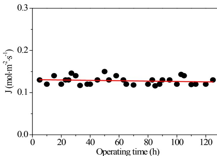
**Fig. S7** Long-term operation for H<sub>2</sub> flux at 473 K and 100 kPa.
