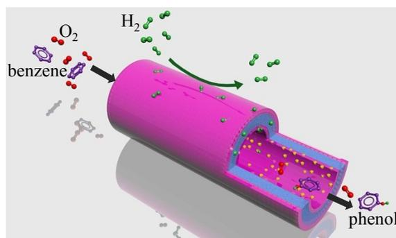
**Fig. S2** Reaction scheme of Pd-TSH composite membrane reactor.
