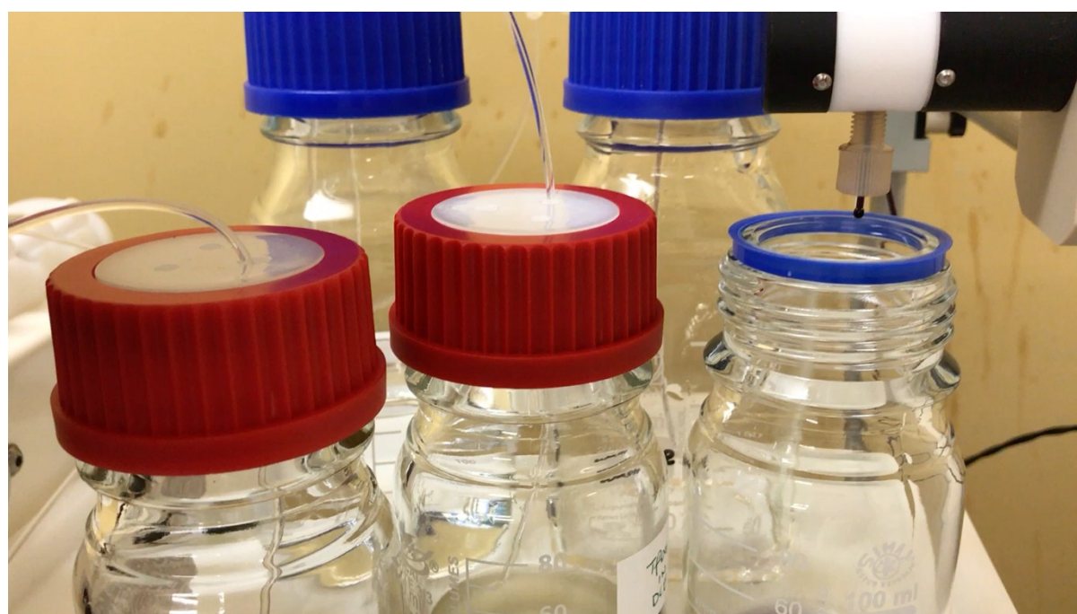
A video showing the black product of HCPs eluted from a commercial flow synthesis reactor set-up from Vapourtec. The red-capped Schott bottles contain transparent chloroformic solutions of the substrate and catalyst (left) and crosslinker (right).
