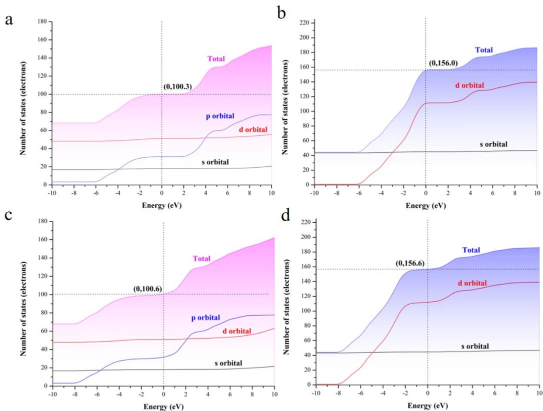
Figure S8 The integrated densities of states of MoO<sub>3</sub> and Ni<sub>0.125</sub>MoO<sub>3</sub>. Mo atom (a) and O atom (b) in MoO<sub>3</sub>, and Mo atom (c) and O atom (d) in Ni<sub>0.125</sub>MoO<sub>3</sub>. The integrated densities of states indicates that the inserted Ni atoms transfer electrons to MoO<sub>3</sub>, and all Mo atoms and O atoms have obtained some electrons.
