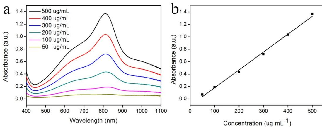
Figure S6 a) UV-Vis-NIR absorption spectra and b) fitting curve of the absorption values at 808 nm of the  $\text{Ni}_{0.125}\text{MoO}_3$  nanodots of dispersions at different concentrations in water.
