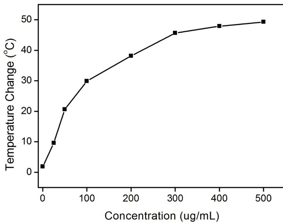
Figure S10. Plot of temperature variation upon the 8-min irradiation *versus* the different concentration suspension of Ni<sub>0.125</sub>MoO<sub>3</sub> nanodots.
