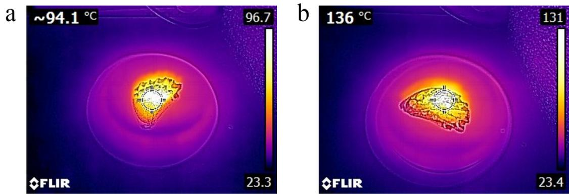
Figure S12. The IR photographs of natural butterfly wing(a) and (b) the  $\text{Ni}_{0.125}\text{MoO}_3$  nanodot- butterfly wing composite under simulated solar irradiation ( $0.3\text{kW m}^{-2}$ )
