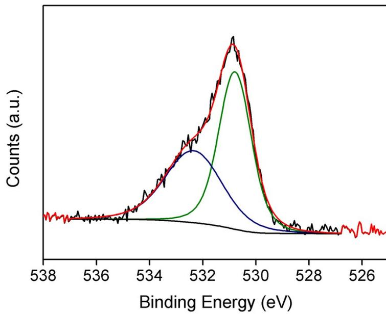
Figure S4. XPS of O 1s spectra of the  $\text{Ni}_x\text{MoO}_3$  sample
