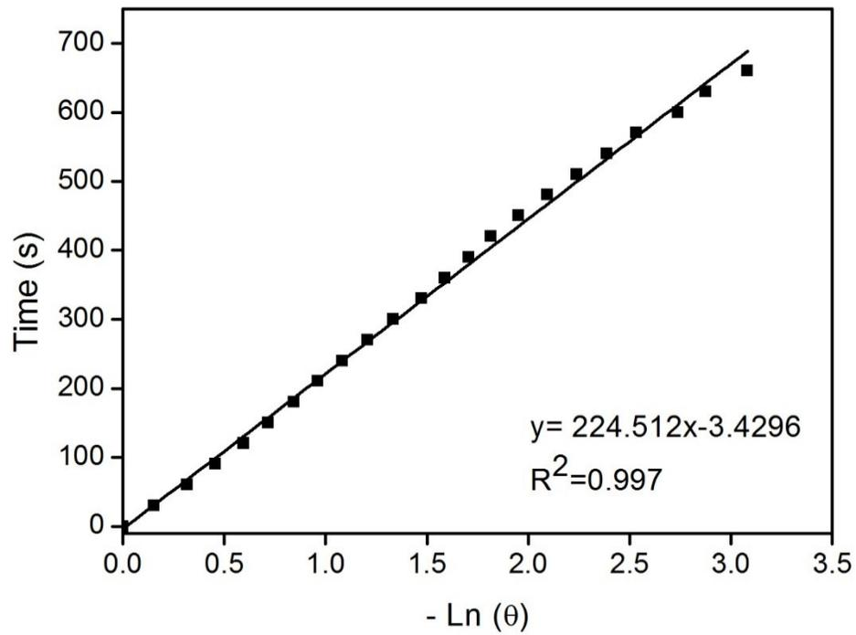
Figure S11. The determination of the time constant for heat transfer of the system using linear regression of the cooling profile of  $\text{Ni}_{0.125}\text{MoO}_3$  nanodots.
