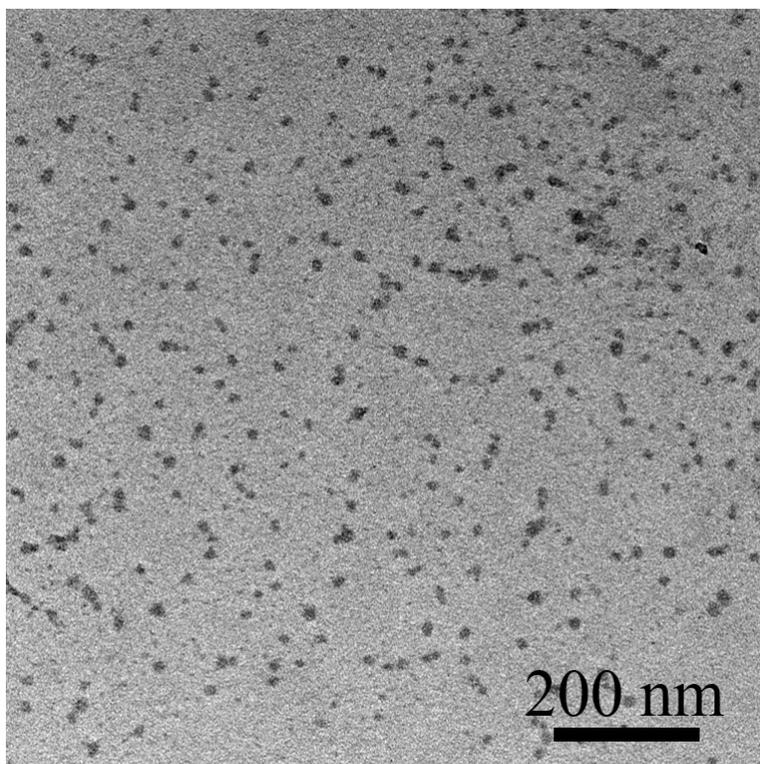
Figure S3. TEM image of the as-prepared  $\text{Ni}_x\text{MoO}_3$  nanodots.
