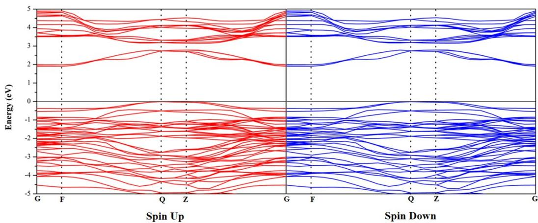
Figure S7 The band structure of bulk MoO<sub>3</sub>. The band gap value is 1.9eV.
