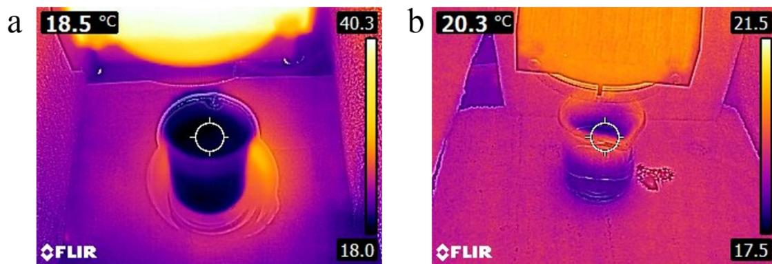
Figure S13. IR photographs of 50mL beakers without the  $\text{Ni}_{0.125}\text{MoO}_3$  nanodot- butterfly wing composite on top of the water surface before the solar irradiation(a) and after the solar irradiation for 3 hours(b).
