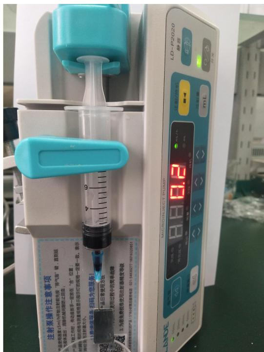
**Fig. S1** The digital device diagram for preparing gradient polymer brushes.
