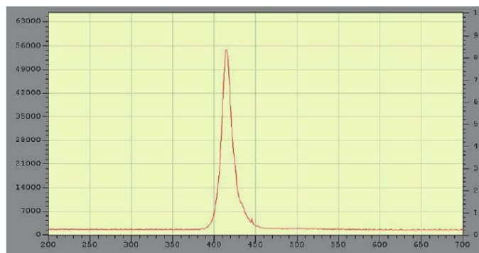
Figure S26. Emission of the blue LED (420 nm) (spectrum is taken from the producer's specification).
