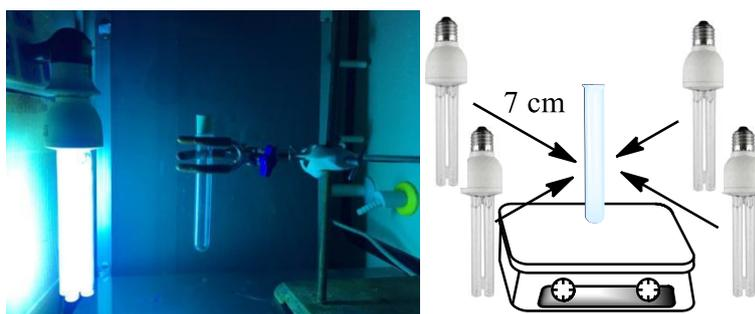
**Figure S1 Placement of CFL around quartz test tube.** Four 25 W UVC compact fluorescent light bulbs were placed around the quartz test tube and the distance was about 7 cm. A cardboard box lined with tin foil was placed over the lamps and stir plate. In one side of the cardboard box, part of the side was cut out, and a high-speed fan was set up into for dissipating heat.
