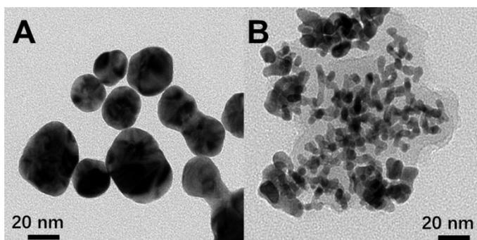
**Figure S2.** TEM images of (A) Au NPs and (B) Au-PDA.
