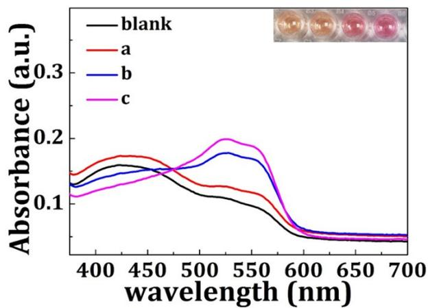
**Figure S4.** The UV-vis spectra of methyl red in Au nanozyme (a, Au-PDA; b, Au hydrogel-HCl; c, Au hydrogel)-glucose systems.
