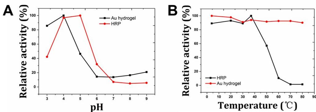
**Figure S7.** The effect of pH and incubation temperature on peroxidase-like activity of Au hydrogel.
