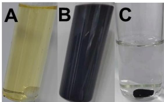
**Figure S1.** Digital pictures of Au hydrogel formation at different stages: (A)  $\text{HAuCl}_4$  solution, (B) initial step after the addition of reducing agent, and (C) formation of Au hydrogel.
