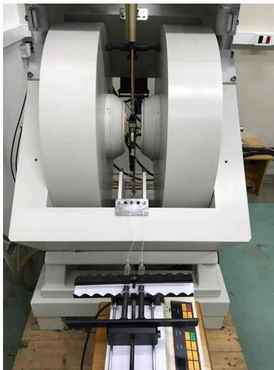
Figure S1. EPR spectrometer with mixing cell resonator for continuous flow measurements. (Photograph taken by coauthor D. R. Truzzi)
