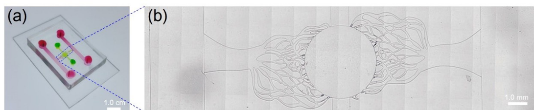
Figure S1 Microfluidic device for cell co-culture, metabolite analysis and cytotoxicity assay. (a) An image of the microfluidic device filled with green and red dye in the HeLa cell culture and HUVEC cell culture part, (b) Microscopic images of the spatial microstructure of the vessel network chip model.
