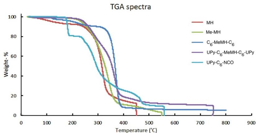
**Fig. S12:** The TGA spectra of maltoheptaose (MH) and its derivatives (MeMH, C<sub>6</sub>-MeMH-C<sub>6</sub>, UPy-C<sub>6</sub>-MeMH-C<sub>6</sub>-UPy) and UPy-C<sub>6</sub>-NCO
