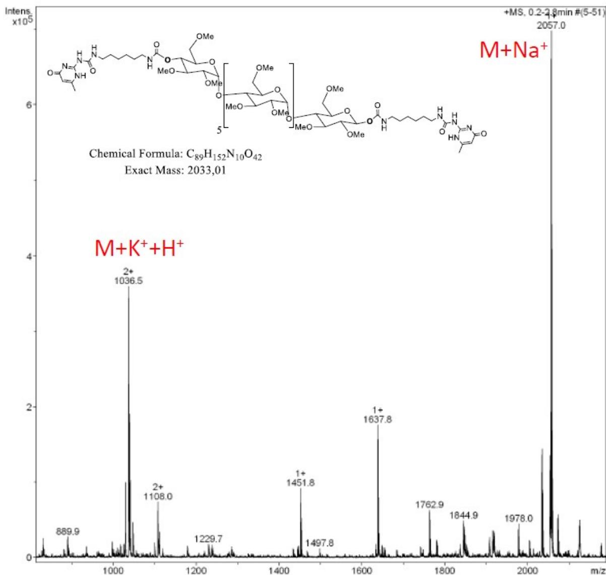
**Fig. S10:** ESI-MS spectra of the methylated maltoheptaose, where both ends have been appended with UPy (UPy-C<sub>6</sub>-MeMH-C<sub>6</sub>-UPy).
