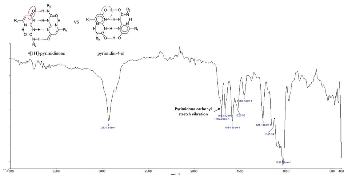
**Fig. S11:** FTIR spectra of the UPy-C<sub>6</sub>-MeMH-C<sub>6</sub>-UPy showing no isocyanate band at  $\nu = 2268 \text{ cm}^{-1}$  and characteristic band at  $\nu = 1700 \text{ cm}^{-1}$  of the pyrimidinone carbonyl stretch vibration, which is absent in the enol tautomer (UPy functionalities remain dimerized in the solid-state under the keto tautomer form).
