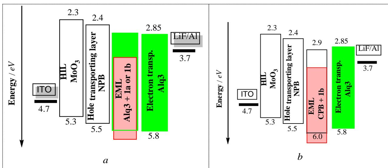
**Fig. 2** Energy-level diagram of devices **1a:Alq<sub>3</sub>** and **1b:Alq<sub>3</sub>** (a), **1b:CBP** (b).
