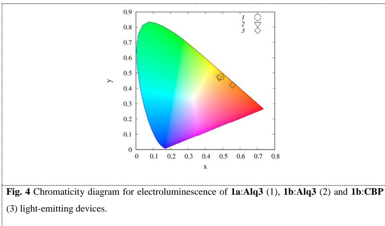
**Fig. 4** Chromaticity diagram for electroluminescence of **1a:Alq<sub>3</sub>** (1), **1b:Alq<sub>3</sub>** (2) and **1b:CBP** (3) light-emitting devices.
