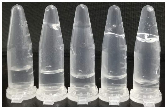
Figure S1. Effects of \text{Cu}^{2+} with different concentrations on the gelation of alginate.
