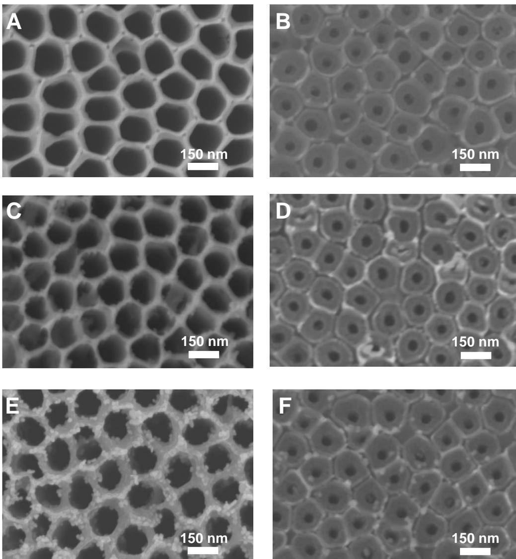
**Fig. S10** Top-view and bottom-view SEM images of TiNMs with AuNPs amplified with silver after the contact with urine samples from the healthy individuals (sample II - A and B) and patients with bladder cancer (sample III - C and D, sample IV - E and F).
