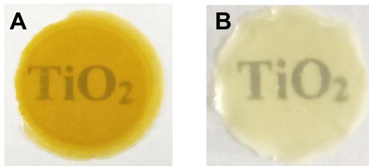
**Fig. S1** Images of self-standing TiNMs: (A) before and (B) after annealing at 450 °C for 2 h in air.
