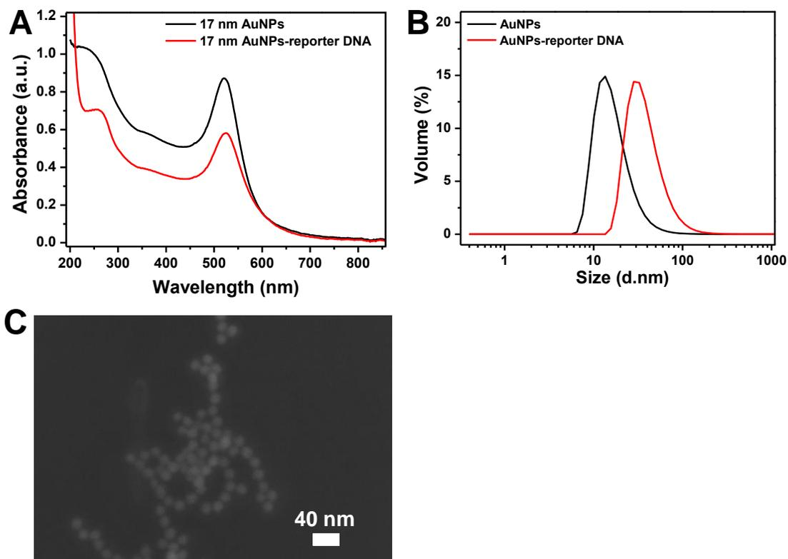
**Fig. S6** UV-vis absorption spectra (A) and size (B) of ~17 nm AuNPs determined by dynamic light scattering before and after modification with the reporter DNA. (C) SEM image of ~17 nm AuNPs.
