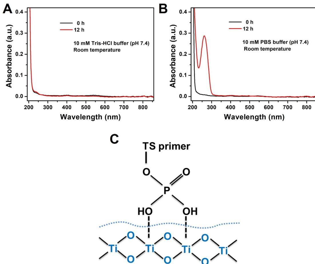
**Fig. S3** UV-vis absorption spectra of TS primer solution after incubation treatment with TiNM/TS primer in (A) 10 mM Tris-HCl buffer (pH 7.4) and (B) 10 mM PBS buffer (pH 7.4). (C) Bidentate interaction of the TS primer with TiNM.
