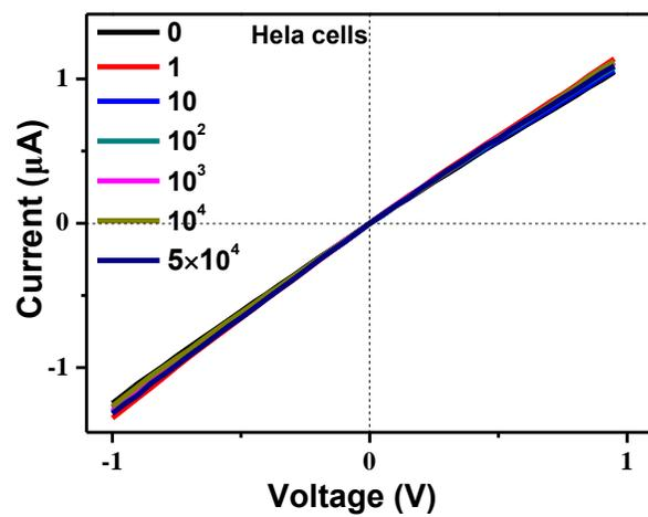
**Fig. S8** *I-V* curves of TiNMs modified with AuNPs in the presence of different concentrations of telomerase.
