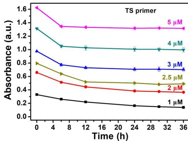
**Fig. S4** TS primer absorption capacity of TiNM as a function of incubation time (0-36 h) and TS primer concentrations (1-5  $\mu\text{M}$ ) at room temperature. The absorbance value of the TS primer solution was recorded at 260 nm.
