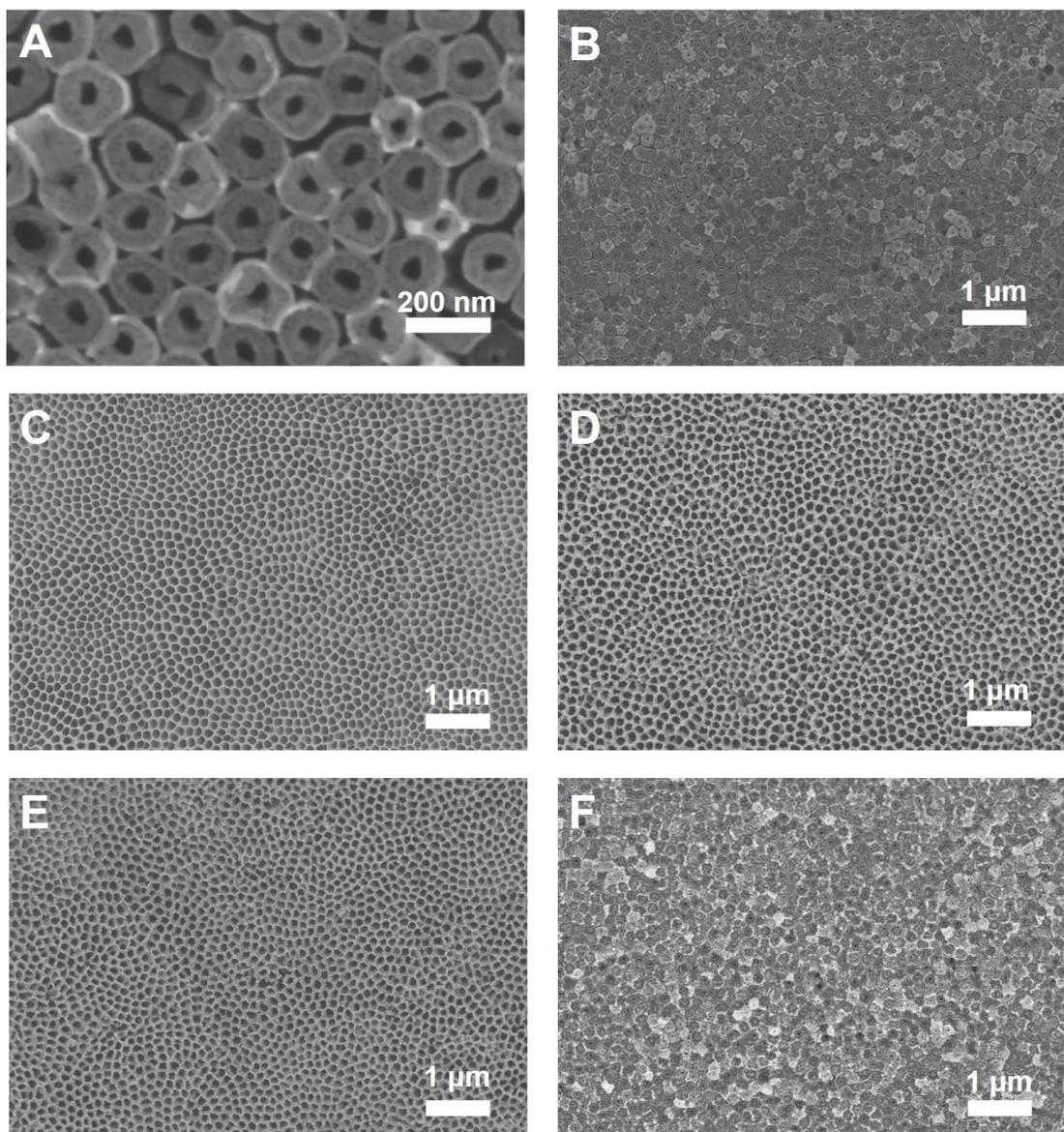
**Fig. S2** Bottom-view SEM images of TiNMs (A and B). Top-view SEM images of TiNMs before (C) and after (D) hybridization with AuNPs-reporter DNA. Top-view (E) and bottom-view (F) SEM images of TiNMs with AuNPs amplified with silver.
