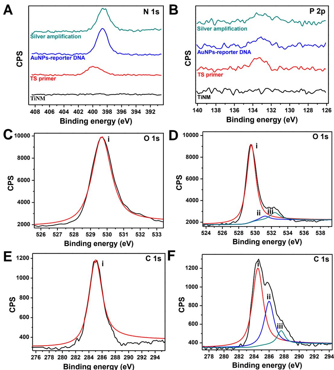
**Fig. S5** High-resolution (A) N 1s and (B) P 2p spectra. High-resolution O 1s spectra of TiNM before (C) and (D) after adsorption of TS primer. High-resolution C 1s spectra of TiNM before (E) and (F) after modification of TS primer. CPS = counts per second.
