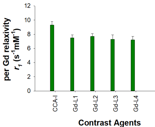
Fig. S5. Per Gd relaxivity comparison of CCA-I with the modified AAZTA chelates, Gd-L1 , Gd-L2 , Gd-L3 and Gd-L4 . Clearly, the close packing of individual chelates in CCA-I further restricts their internal rotation and consequently there is an resultant increase of two units in the per-Gd relaxivity of CCA-I as compared to the individual chelates. r_1 values are measured at 7 T and 25°C.
