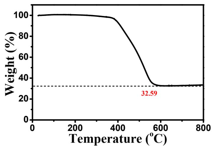
Fig. S5 The TG curve of Co-N-CNTs obtained at air atmosphere.
