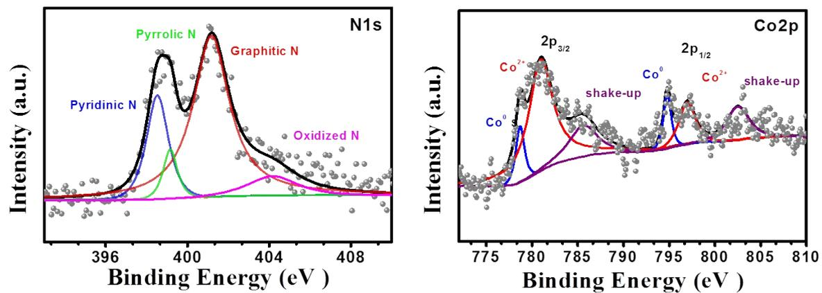
Fig. S4 High resolution XPS spectra of (a) N 1s and (b) Co 2p of Co-N-CNTs.
