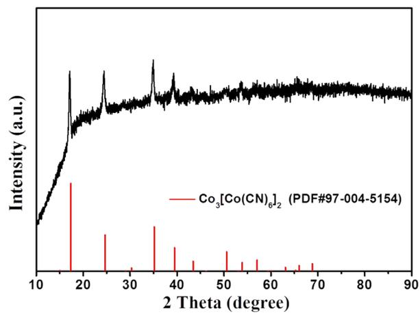
**Fig. S2** XRD pattern of the precursor cobaltic Prussian blue analogue  $\text{Co}_3[\text{Co}(\text{CN})_6]_2$ .
