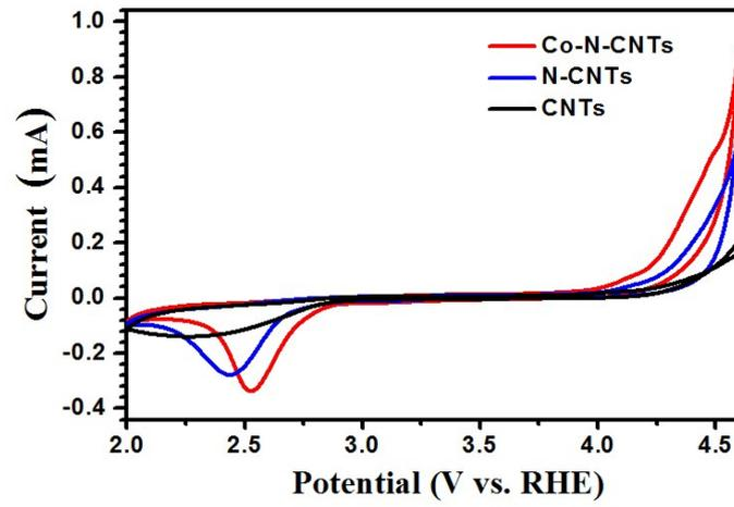
**Fig. S7** CV curves of the Li-CO<sub>2</sub> batteries using the Co-N-CNTs, N-CNTs and commercial CNTs catalysts at a scanning rate of 0.2 mV s<sup>-1</sup>.
