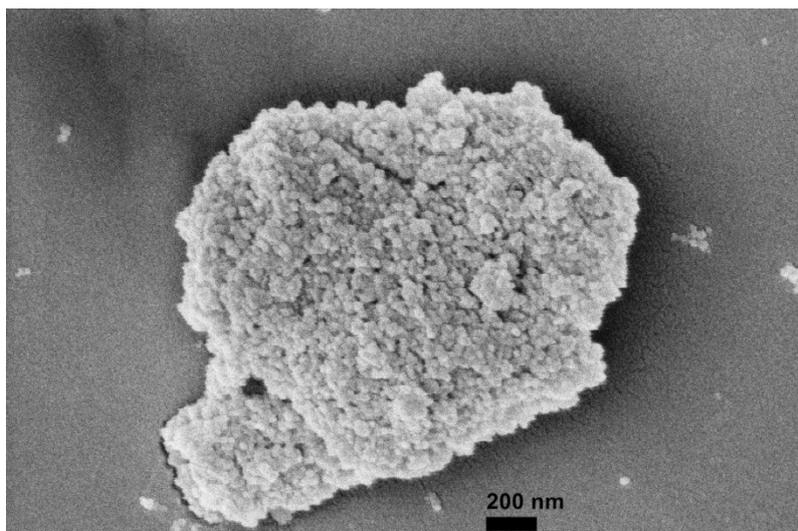
**Fig. S1** SEM image of the precursor cobaltic Prussian blue analogue  $\text{Co}_3[\text{Co}(\text{CN})_6]_2$ .
