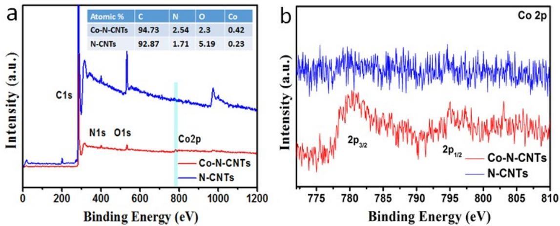
**Fig. S3** (a) XPS survey spectrum and (b) Co 2p spectrum of the Co-N-CNTs and N-CNTs.
