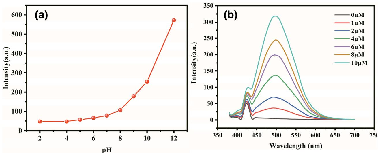
**Figure S3.** (a) Fluorescence intensity of 10 μM OTC under different pH conditions (excitation wavelength: 370nm, emission wavelength: 495nm), (b) Fluorescence emission spectra of different concentrations of OTC in 0.025M NaHCO<sub>3</sub>-NaOH buffer (excitation wavelength: 370nm, pH=9.8).
