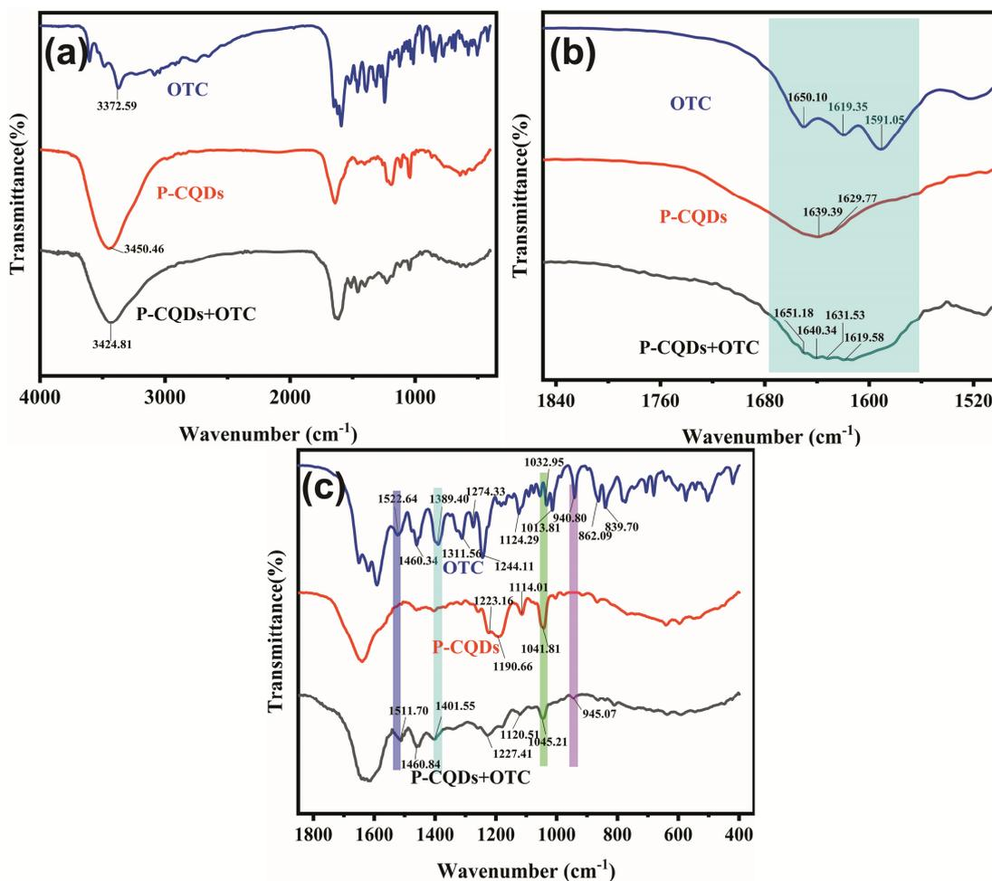
**Figure S10.** The FTIR of OTC, P-CQDs and mixture of OTC and P-CQDs (all samples were dissolved with KBr in mixture of ethanol and water (1:1) in advance, the products were measured using KBr tablet method after freeze-drying for 24h, the mass ratio of P-CQDs and OTC was 2).
