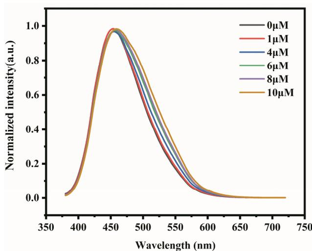
**Figure S4.** Fluorescence emission spectra of CQDs in the presence of different concentrations of OTC in 0.025M NaHCO<sub>3</sub>-NaOH buffer (CQDs concentration: 5mg/L, excitation wavelength: 370nm, pH=9.8).
