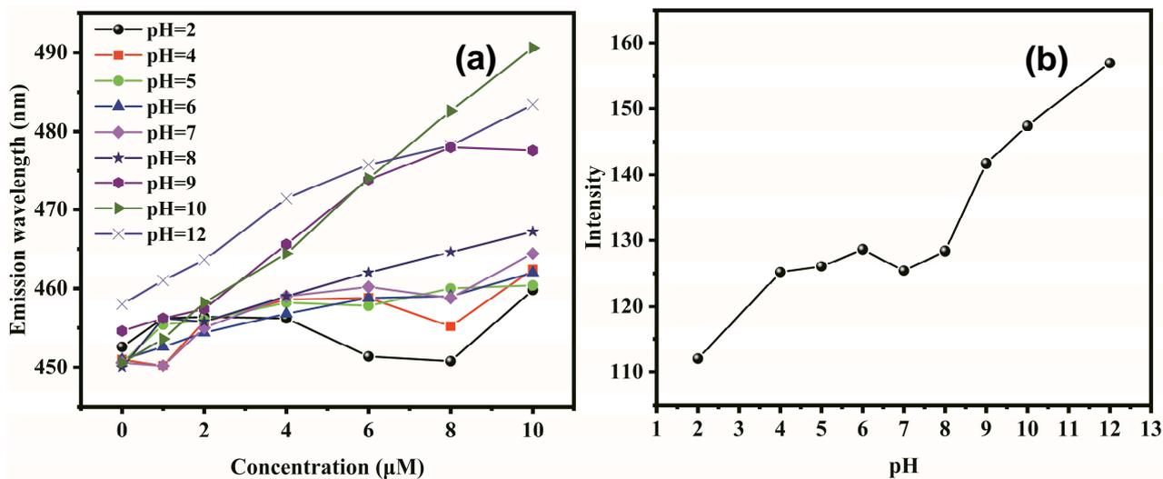
**Figure S11.** (a) The maximum fluorescence emission wavelength of P-CQDs in the presence of different concentrations of OTC under a wide range of pH conditions, (b) The fluorescence intensity of 1mg/L P-CQDs under different pH conditions (excitation wavelength: 370nm, emission wavelength: 457nm, the pH of solutions was adjusted by dropping a certain volume of 1M HCl or 1M NaOH into PBS buffers).
