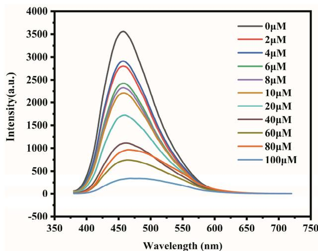
**Figure S15.** Fluorescence emission spectra of P-CQDs in the presence of different concentrations of TC in 0.025M NaHCO<sub>3</sub>-NaOH buffer (P-CQDs concentration: 5 μg/ml, excitation wavelength: 370nm, pH=9.8).
