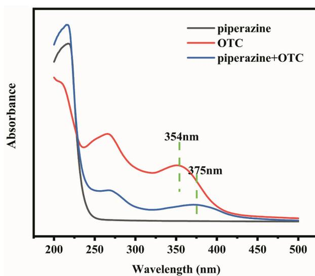
**Figure S6.** UV/Vis absorption spectra of piperazine (0.02M), OTC (10 $\mu$ M) and mixture of piperazine (0.01M) and OTC (2 $\mu$ M).
