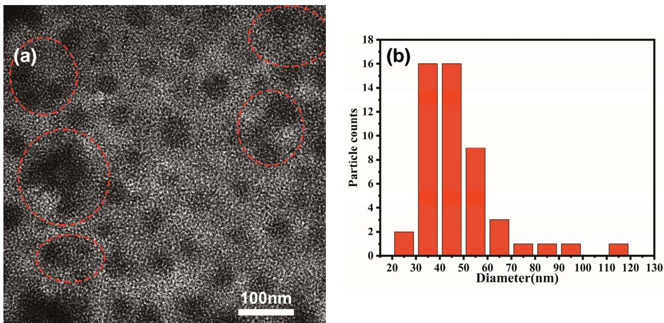
**Figure S8.** TEM image (a) and size distribution (b) of P-CQDs in the presence of OTC (OTC: 10μM, the particle size distribution was calculated by measuring 50 particles).
