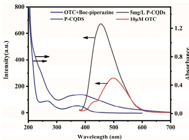
**Figure S16.** Fluorescence emission intensity of P-CQDs and OTC, and UV-vis absorption spectra of P-CQDs and mixture of OTC and Boc-piperazine (pH=9.8, excitation wavelength: 370nm, the concentration of Boc-piperazine was 10 μM).
