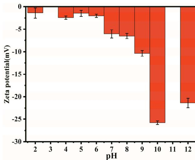
**Figure S12.** The zeta potential of P-CQDs under different pH conditions (P-CQDs concentrations: 5mg/L, the number of parallel samples was three).
