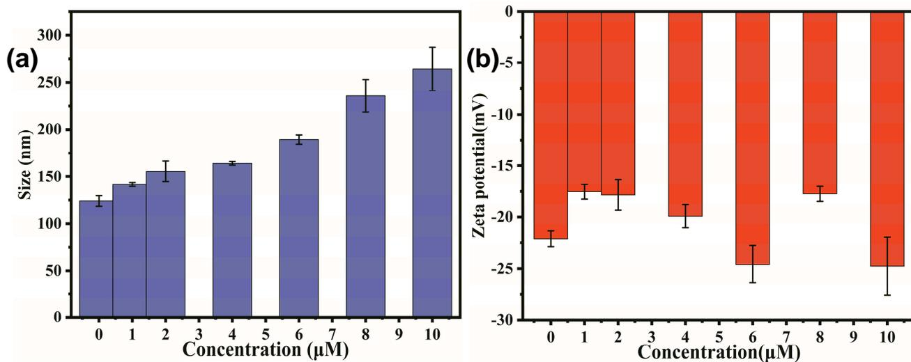
**Figure S7.** The particle size (a) and zeta potential (b) of P-CQDs in the presence of different concentrations of OTC (P-CQDs concentrations: 5mg/L, pH=9.8, the number of parallel samples was three).
