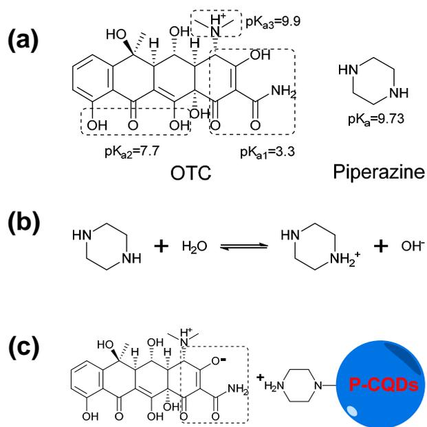
**Figure S9.** (a) The structure and pKa of OTC and piperazine molecule, (b) the dissociation equation of piperazine when pH is 9.8, and (c) the possible electrostatic interaction between P-CQDs and OTC.
