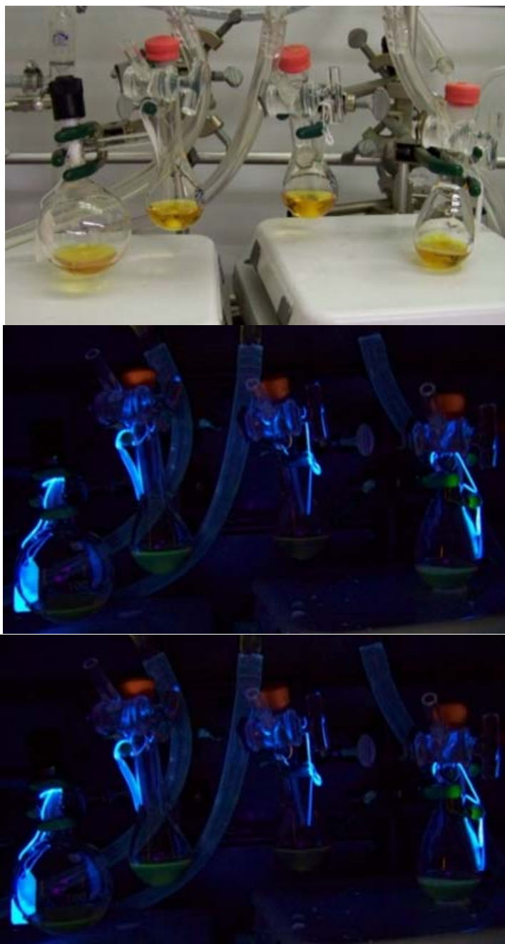
Figure S11. Photograph of the catalytic reactions with 1.5 mol % [(COD)Rh(BoPNP)]BF 4 in THF for the (far left) hydrogenation of limonene, (left middle) hydrosilylations of limonene, (right middle) hydroboration of limonene, and (far right) hydroacylation of 2,2-dimethyl-4-penal under (top) ambient light, (middle) UV light 20 minutes after the additon of [(COD)Rh(BoPNP)]BF 4 , and (bottom) UV light after 24 hours.
