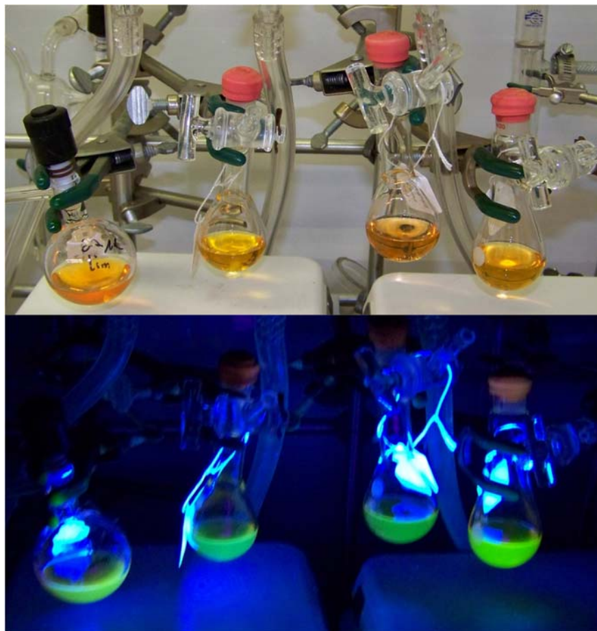
Figure S9. Photograph of the catalytic reactions with 1.5 mol % [(\text{COD})\text{Rh}(\text{BoPNP})]\text{BF}_4 in \text{CH}_2\text{Cl}_2 for the (far left) hydrogenation of limonene, (left middle) hydrosilylations of limonene, (right middle) hydroboration of limonene, and (far right) hydroacylation of 2,2-dimethyl-4-penal under (top) ambient light and (bottom) UV light five minutes after the addition of [(\text{COD})\text{Rh}(\text{BoPNP})]\text{BF}_4 .
