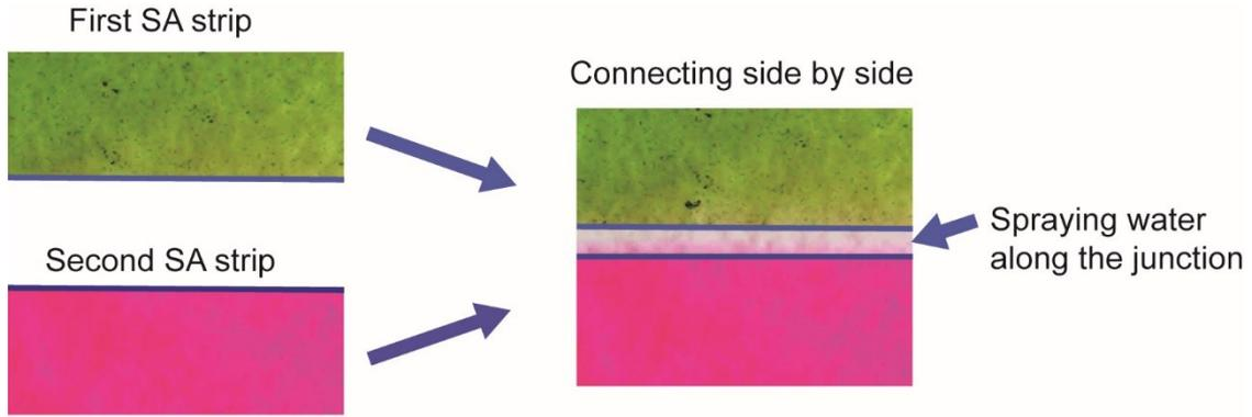
**Fig. S3 Schematics** showing how two SA strips were assembled together side by side. The assembled two strips self-healed into an integral piece through water-induced molecular diffusion.
