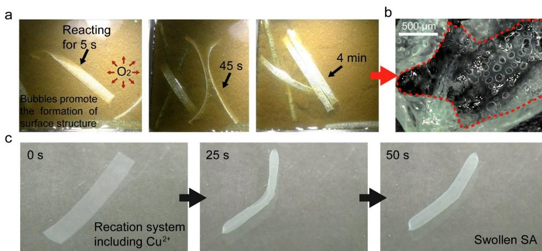
**Fig. S2 Evolutionary process of a solid SA strip to a hollow hydrogel tube.** (a) Snapshots showing that the SA strips were converted to hydrogel tube in 4 min. (b) A image revealing the structure of inner wall of hydrogel tube. The gas bubbles released and left many holes in the tube wall. (c) The SA strip swelled only if there was no H<sub>2</sub>O<sub>2</sub> element in the reaction solution.
