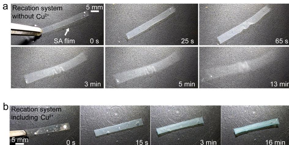
**Fig. S1 Cu<sup>2+</sup>-induced crosslinking.** (a) An SA strip was immersed in water without Cu<sup>2+</sup>, and it dissolved in 13 min. (b) As it was immersed in Cu<sup>2+</sup>-containing water solution, it swelled with sorption of water, but did not dissolve owing to Cu<sup>2+</sup>-induced crosslinking with carboxyl groups of SA molecules.
