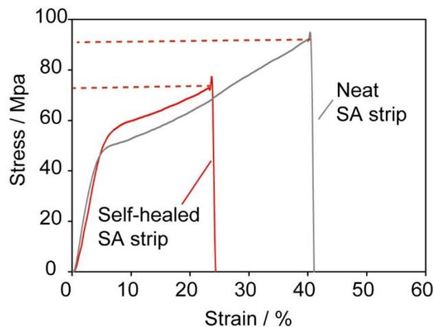
**Fig. S5 Tensile curves of self-healed SA strip and the neat SA strip.** The self-healing ratio was calculated based on their maximum stress values as indicated by red broken line.
