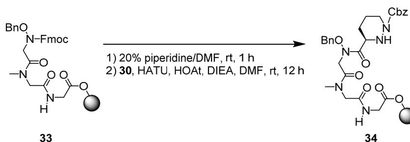
**Tetrapeptide 34:** 20% piperidine in DMF was added to the reaction tube containing the above resin **33** (0.116 mmol) and the mixture was shaken for 1 h at room temperature. The resin was washed with DMF three times. In another flask, piperazic acid **30** (93.7 mg, 0.355 mmol) was activated with HATU (134.9 mg, 0.355 mmol), HOAt (47.9 mg, 0.355 mmol), DIEA (123.4  $\mu$ L, 0.710 mmol) in DMF and resultant mixture was
