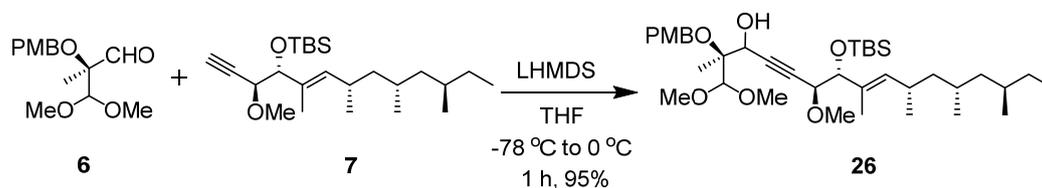
**Alcohol 26:** To a stirred solution of alkyne **7** (22.0 mg, 0.056 mmol) in dry THF (0.6 mL) was added LHMDS (1.04 M in hexane, 0.21 mL, 0.218 mmol) at -78 °C under N<sub>2</sub> atmosphere. After stirring for 30 min at 0 °C, the reaction mixture was cooled to -78 °C
