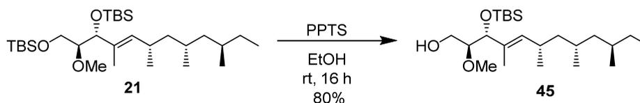
**Alcohol 45:** To a stirred solution of **21** (25.0 mg, 0.048 mmol) in EtOH (0.56 mL) was added PPTS (1.2 mg, 4.78  $\mu\text{mol}$ ) at  $0^\circ\text{C}$ . After stirring for 16 h at room temperature, the reaction mixture was evaporated and the residue was purified by silica gel flash column chromatography (ethyl acetate/*n*-hexane = 5:95) to afford 15.4 mg (80%) of **45** as a
