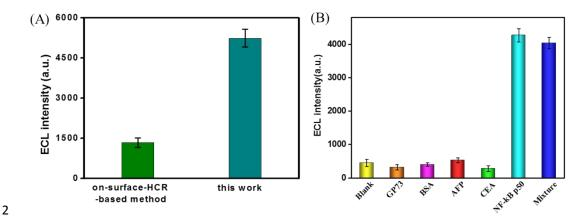
Fig.S2 (A) Comparison of ECL intensity between the on-surface-HCR-based method and the proposed method in the presence of 500 pM NF-κB p50. (B) ECL response in the presence of 100 pM NF-κB p50 or 10 nM of other analytes. All the detection was performed in 6.7 mM phosphate buffer (pH 7.4) containing 20 mM TPA. Scan range: 0.2 to 1.6 V. Scan rate: 50 mV/s.
