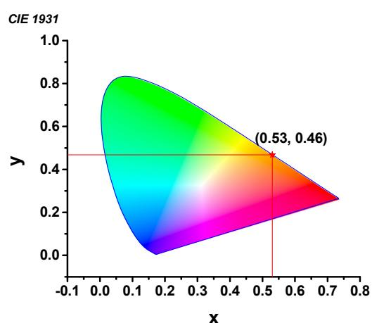
**Fig. S6.** CIE coordinates of the emissions of solid SBF3.
