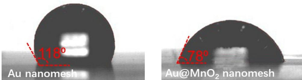
**Figure S3.** Photographs of water droplet on Au nanomesh and the Au@MnO<sub>2</sub> nanomesh, using PDMS as the substrate.
