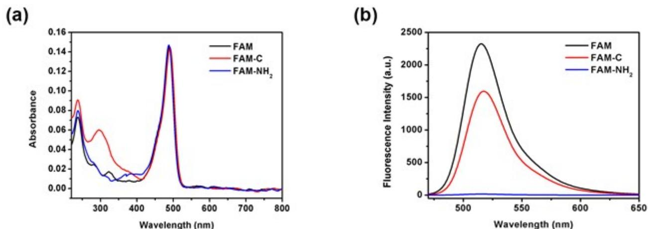
**Figure S9.** Absorption (a) and fluorescence spectra (b) of 2  $\mu\text{M}$  fluorescein (FAM), FAM-C and FAM-NH<sub>2</sub>. FAM-C showed strong fluorescence enhancement over FAM-NH<sub>2</sub>.
