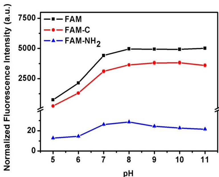
**Figure S10.** The pH-dependent fluorescence emission ( $\lambda_{\text{ex}} = 490 \text{ nm}$ ,  $\lambda_{\text{em}} = 520 \text{ nm}$ ) of both 1.1  $\mu\text{M}$  FAM-NH<sub>2</sub> and FAM-C in the range of pH 5~11 (100 mM sodium phosphate buffer). In any situation, FAM-C has
