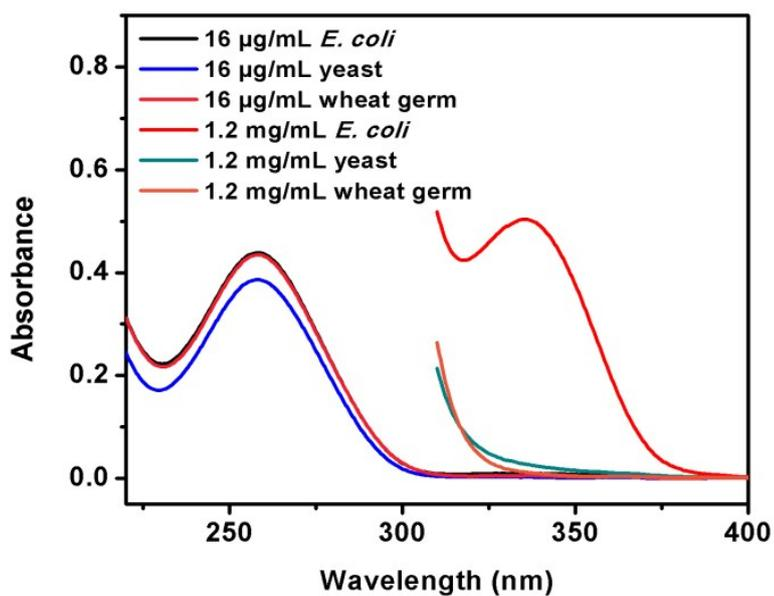
**Figure S12.** Absorption spectra of 16 µg/mL and 1.2 mg/mL different tRNA samples. *E. coli* tRNA exhibited an absorption peak near 330 nm belonging to s<sup>4</sup>U.
