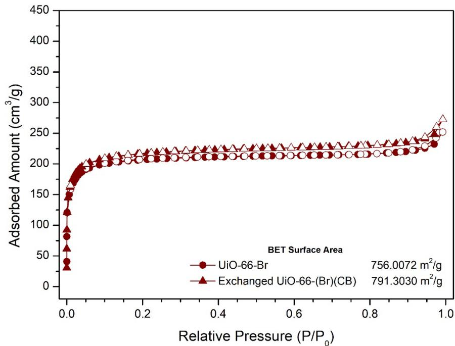
**Fig. S13** N<sub>2</sub> full isotherm (at 77K) and BET surface area for UiO-66-Br and exchanged UiO-66-(Br)(CB).
