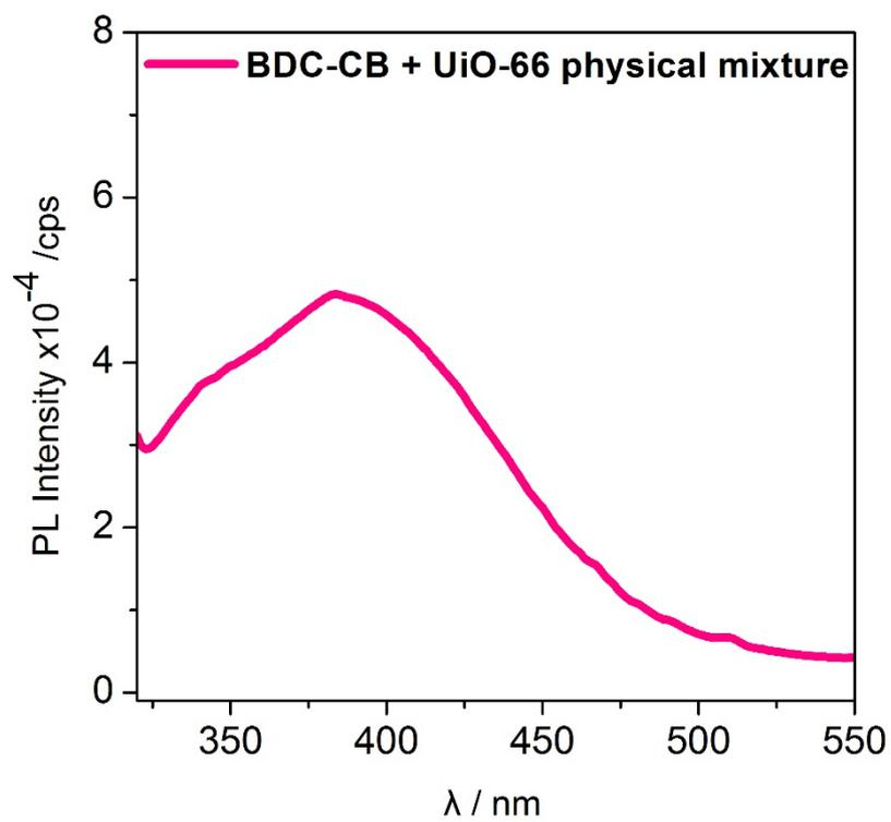
**Fig. S17** Photoluminescence (PL) spectra of the physical mixture of BDC-CB and UiO-66 (10 mol% of BDC-CB to UiO-66).
