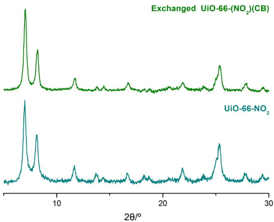
**Fig. S6** PXR of UiO-66-NO<sub>2</sub> and exchanged UiO-66-(NO<sub>2</sub>)(CB).
