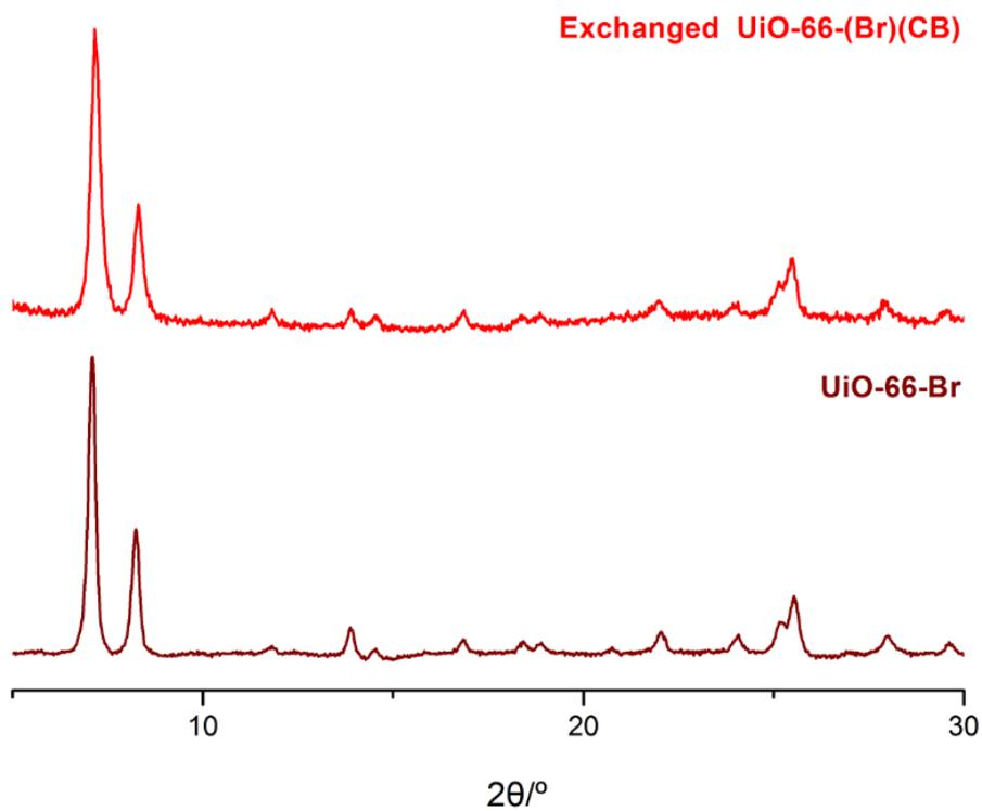
**Fig. S5** PXR of UiO-66-Br and exchanged UiO-66-(Br)(CB).
