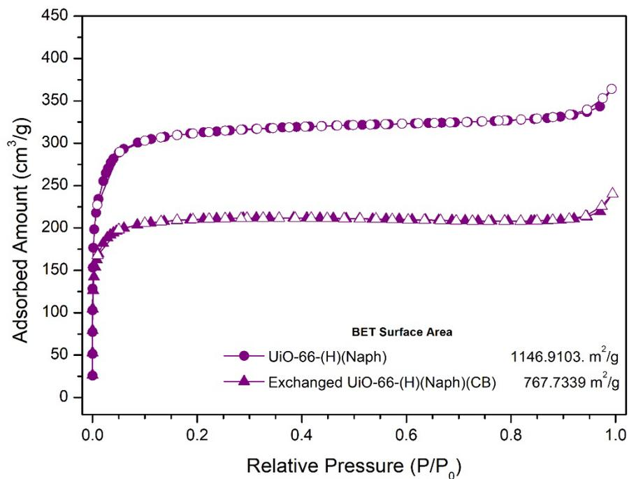
**Fig. S15**  $N_2$  full isotherm (at 77K) and BET surface area for UiO-66-(H)(Naph) and exchanged UiO-66-(H)(Naph)(CB).
