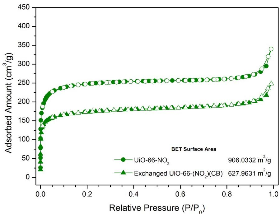
**Fig. S14** N<sub>2</sub> full isotherm (at 77K) and BET surface area for UiO-66-NO<sub>2</sub> and exchanged UiO-66-(NO<sub>2</sub>)(CB).
