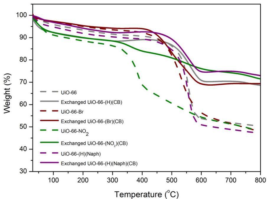
**Fig. S16.** Thermogravimetric analysis (TGA) of UiO-66 and exchanged UiO-66-Rs with carborane functionalities.
