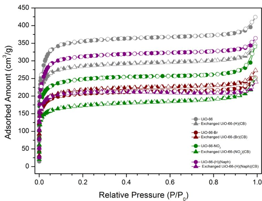
**Fig. S11** N<sub>2</sub> full isotherm (at 77K) for UiO-66s and exchanged UiO-66-(R)(CB)s.
