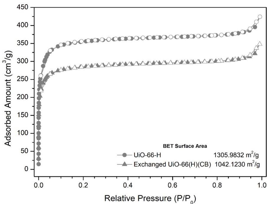
**Fig. S12** N<sub>2</sub> full isotherm (at 77K) and BET surface area for UiO-66 and exchanged UiO-66-(H)(CB).
