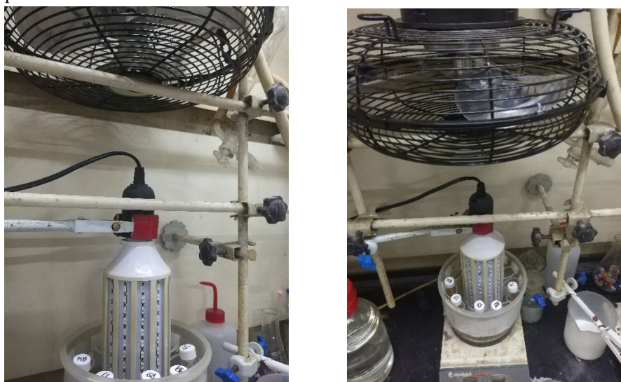
Figure S1. Photograph of the photocatalytic reactor used for reactions conducted under blue LED irradiation.
