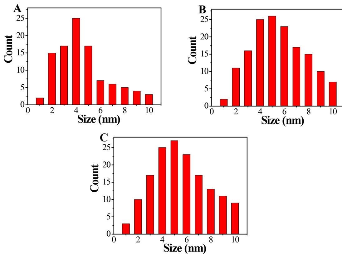
**Figure S2.** The size distribution of Pd NPs in (A) Pd/ZnO catalyst, the size distribution of PdZn intermetallic alloy NPs in (B) PdZn/ZnO catalyst, (C) PdZn@C/ZnO catalyst.
