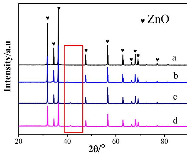
**Figure S3.** XRD patterns of (a) ZnO, (b) Pd/ZnO, (c) PdZn/ZnO and (d) PdZn@C/ZnO.
