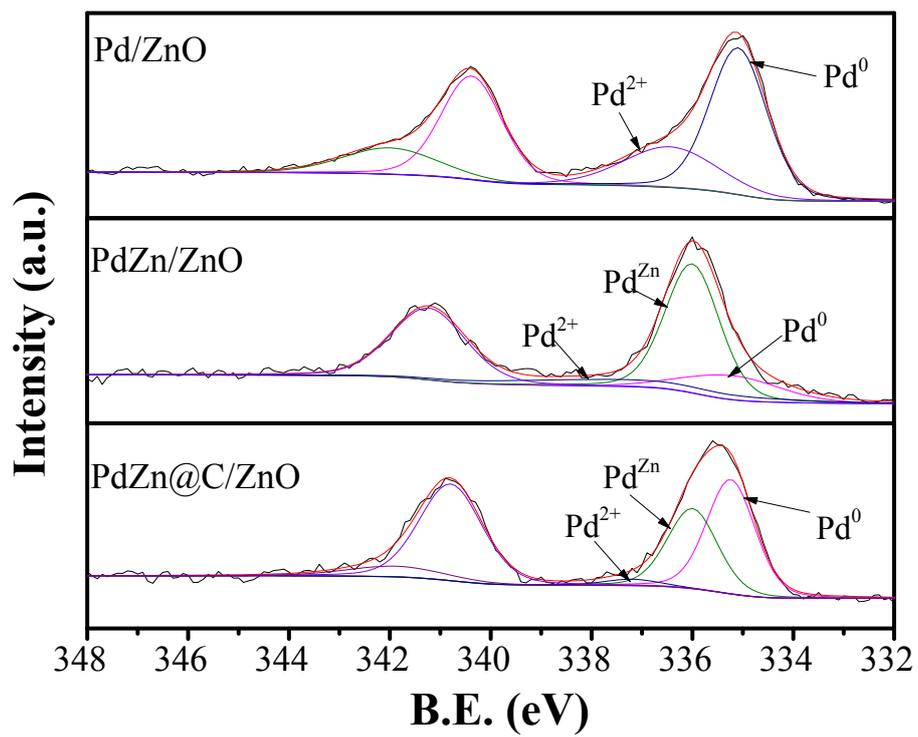
**Figure S4.** XPS spectra of Pd/ZnO, PdZn/ZnO and PdZn@C/ZnO.
