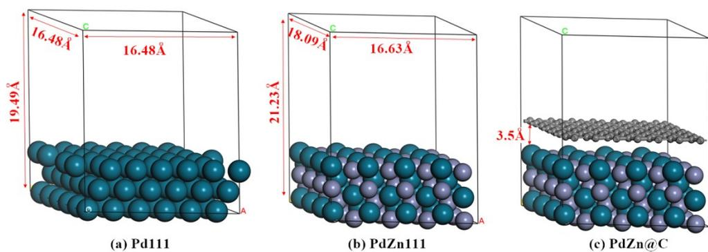
**Figure S6.** Models of Pd (111) (a), PdZn (111) (b) and PdZn@C (c). The blue, purple and gray balls represent Pd, Zn and C atoms, respectively. The structure of PdZn@C is an ideal model, and the distance of 3.5 Å is an approximated average value. After the adsorption of intermediates, the distance will have a fluctuation, as shown in Fig.S7.
