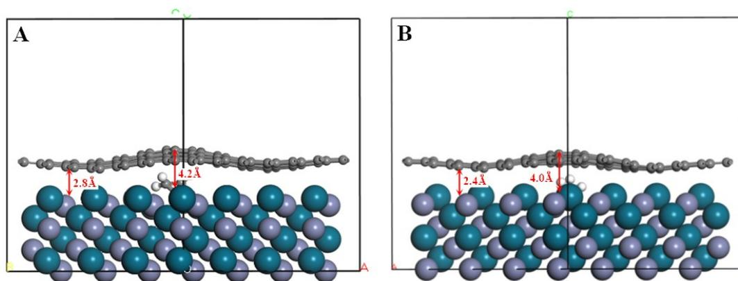
**Figure S7.** The adsorption structures of  $C_2H_4$  (A) and  $CH_3$  (B) on PdZn@Gr.
