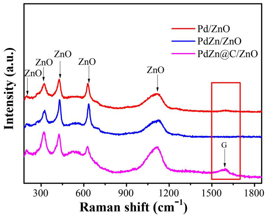
**Figure S5.** Raman spectra of the Pd/ZnO, PdZn/ZnO and PdZn@C/ZnO catalysts.
