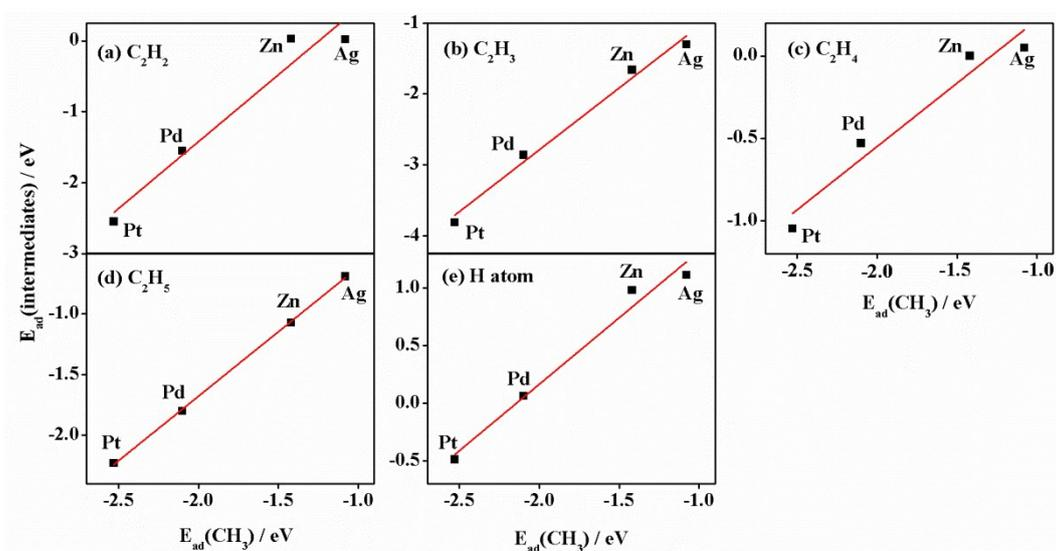
**Figure S8.** Scaling relation between the adsorption energy of CH<sub>3</sub> and that of intermediates in hydrogenation of acetylene
