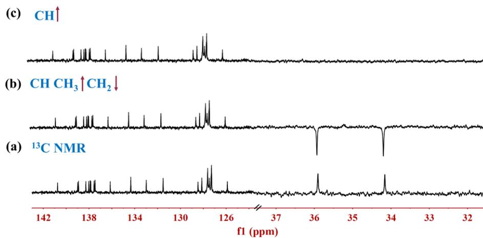
**Figure S6.** (a) <sup>13</sup>C NMR, (b) DEPT-135° NMR, and (c) DEPT-90° NMR spectra of PCMC in CDCl<sub>3</sub>.
