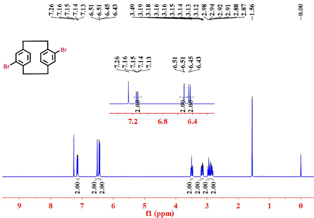
**Figure S24.**  $^1\text{H}$  NMR spectrum of 4,16-dibromo[2.2]paracyclophane (**6**) in  $\text{CDCl}_3$ .
