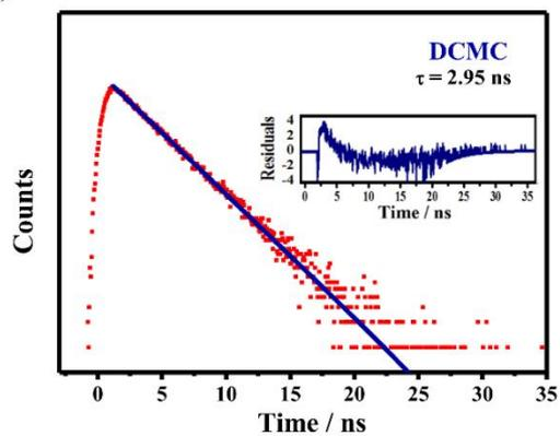
**Figure S15.** (a) Solid powder of **DCMC** (i) and **PCMC** (ii), fluorescent photographs of **DCMC** (iii) and **PCMC** (iiii) solid under UV irradiation at  $\lambda = 365 \text{ nm}$ . (b) Emission lifetime decay for **DCMC** in  $\text{CH}_2\text{Cl}_2$  measured at  $\lambda = 458 \text{ nm}$ . Insert: curve fitting residuals for **DCMC**.
