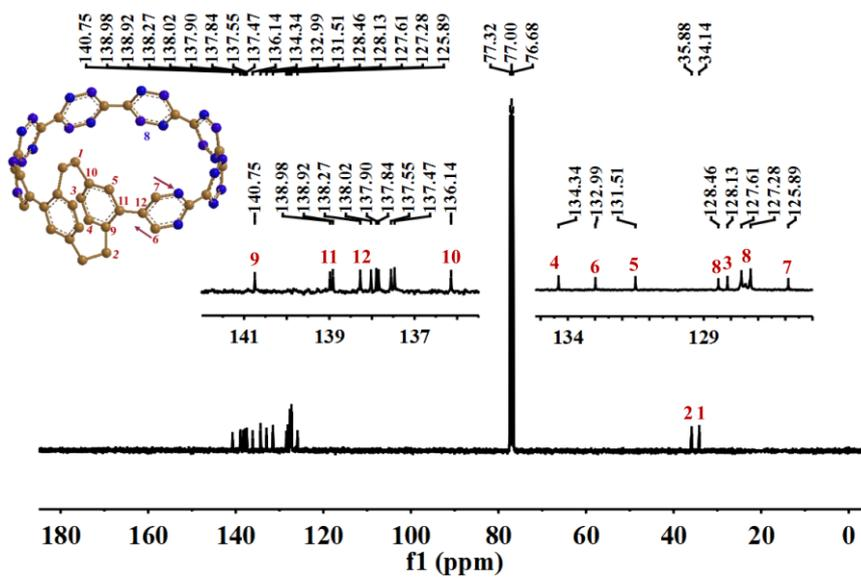
**Figure S12.**  $^{13}\text{C}$  NMR spectrum of PCMC in  $\text{CDCl}_3$ .
