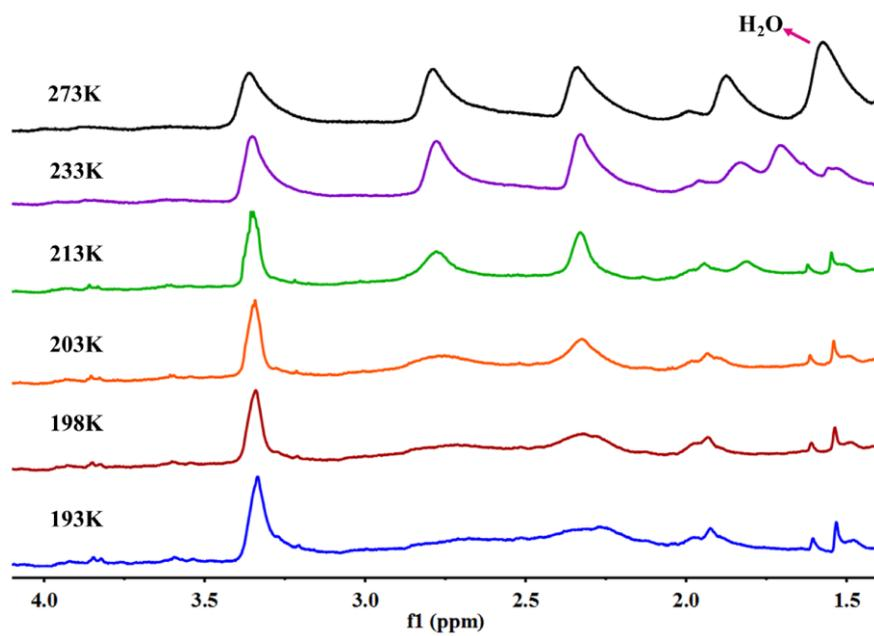
**Figure S16.** VT-NMR spectra of **PCMC** in the range of 1.4-4.1 ppm in CD<sub>2</sub>Cl<sub>2</sub>.
