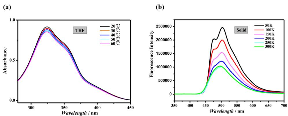
**Figure S17.** Variable-temperature UV-vis spectra in THF (a) and fluorescence spectra in solid form (b) of **PCMC**.
