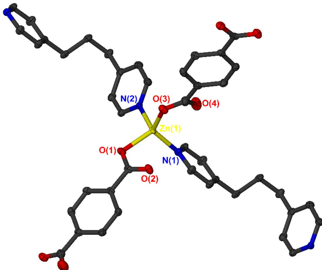
**Figure S1.** View of the coordination environment of  $Zn^{2+}$  in **1** (50% probability thermal ellipsoids; hydrogen atoms omitted for clarity).
