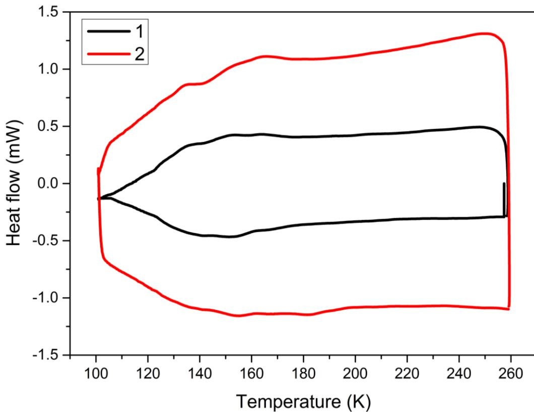
**Figure S6.** Differential scanning calorimetry (DSC) of **1** (black) and **2** (red).
