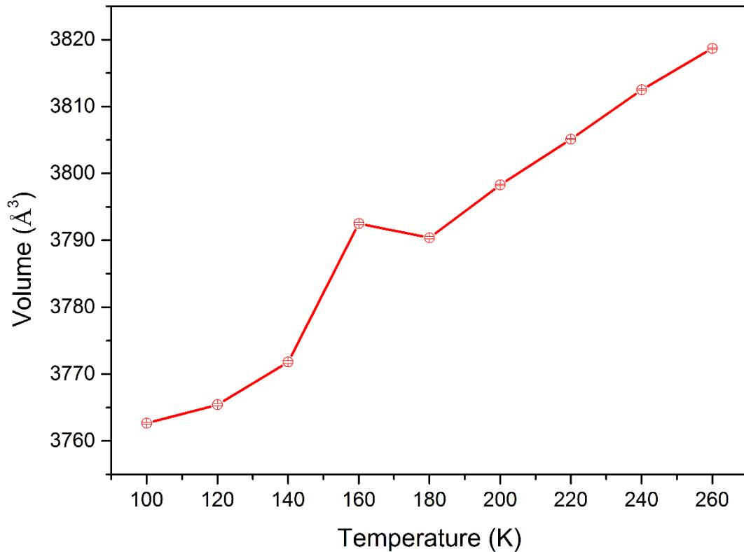
**Figure S5.** Variation of unit cell volume of **1** with temperature .
