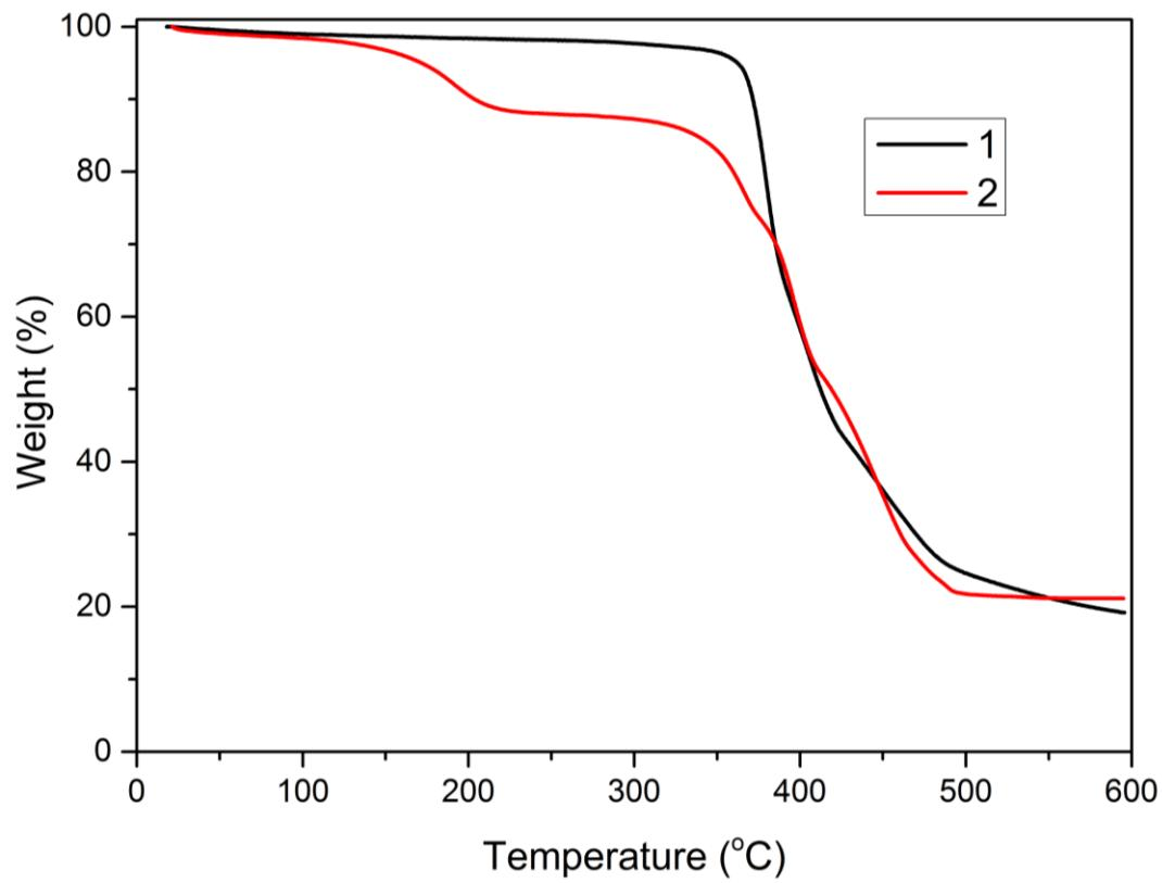
**Figure S7.** Thermogravimetric analysis (TGA) of **1** (black) and **2** (red).
