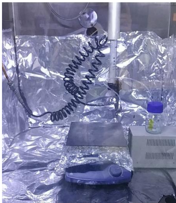
Figure S7. The homemade electronic-controlled spraying device
