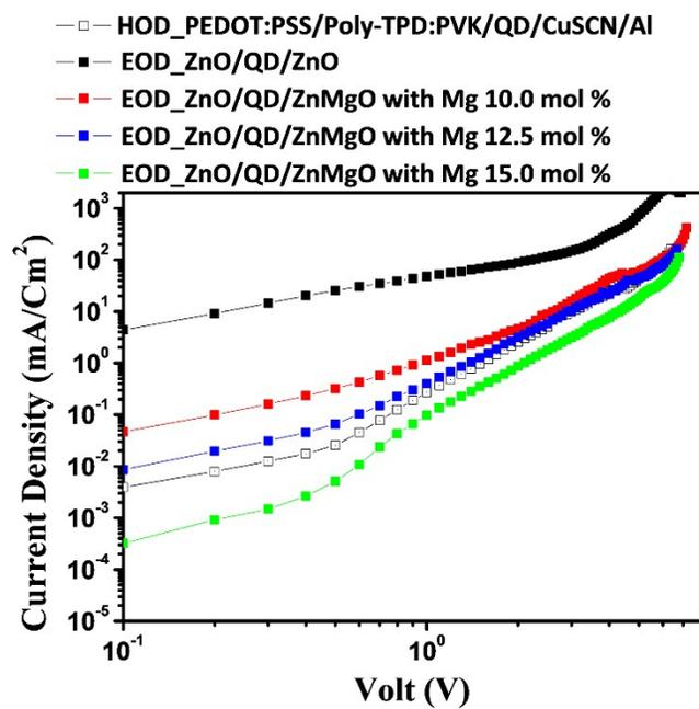
**Figure S3.** Current density-voltage curves of a HOD and EODs. ZnMgO with Mg 12.5 mol% demonstrated current density of the EOD that is closest to that of the HOD. ZnMgO with Mg 15.0 mol% demonstrated lowest current density.
