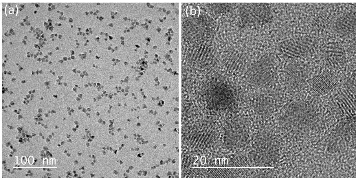
**Figure S4.** TEM images of InP-based non-Cd QDs with magnification of (a) x50000 and (b) x300000.
