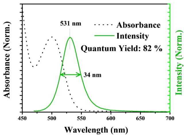
**Figure S1.** Absorption and emission spectra of InP-based QDs. Inset values are emission wavelength, FWHM, and quantum yield. Quantum yield of InP-based QDs in solution phase is measured by spectro-photometer with integration hemi-sphere.
