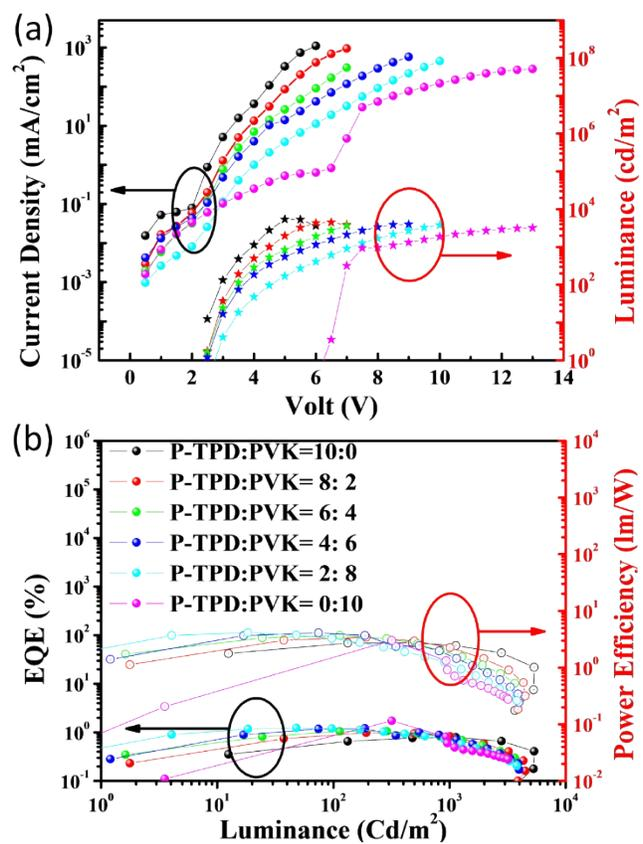
**Figure S2.** (a) J-V-L characteristics of QLEDs with ZnO ETL according to different P-TPD:PVK ratio and (b) EQE and power efficiency of QLEDs as a function of luminance.
