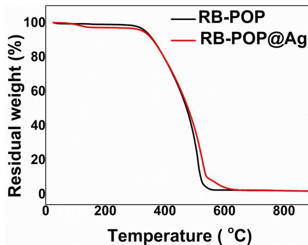
**Figure S3** TGA analysis on **RB-POP** and **Ag@RB-POP** in air, with a ramping rate of 10  $^{\circ}\text{C}$  min.
