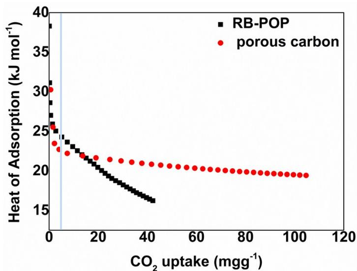
**Figure S10** Isosteric heats of adsorption ( $Q_{st}$ ) for CO<sub>2</sub> adsorption by RB-POP and porous carbon. The isosteric heats of adsorption ( $Q_{st}$ ) are calculated by fitting the CO<sub>2</sub> adsorption isotherms at 273 K and 298 K and applying of the Clausius-Clapeyron equation.
