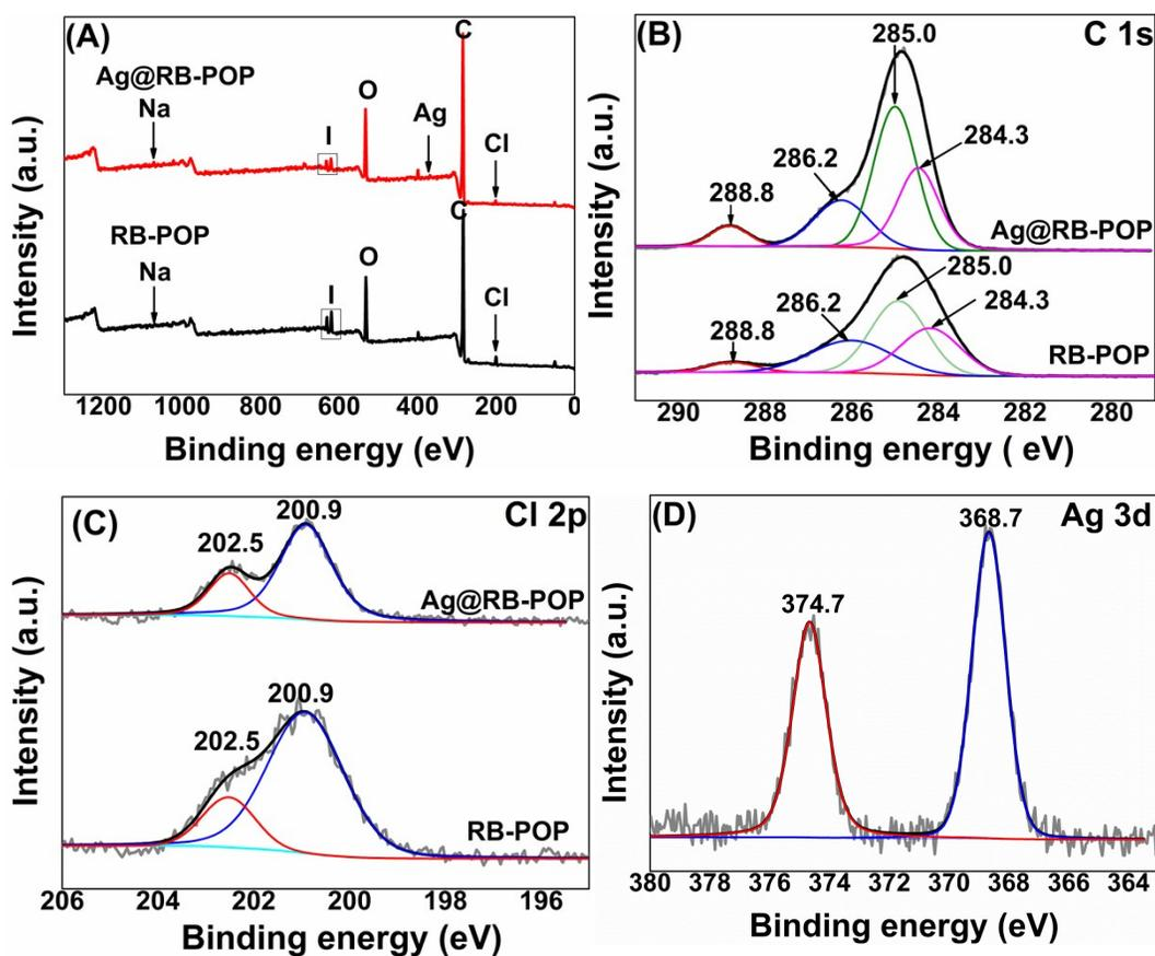
**Figure S9.** XPS spectra: (A) survey spectra, (B) C1s, (C) Cl1s for RB-POP and Ag@RB-POP (D) Ag 3d for Ag@RB-POP -After
