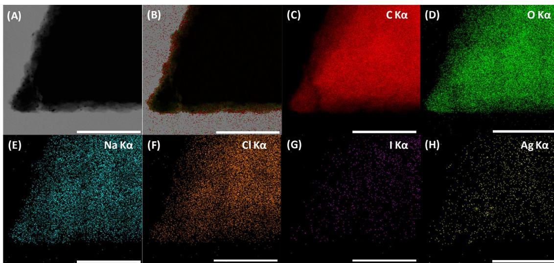
**Figure S8** (A) The(HR)TEM of Ag@RB-POP, Scale bar 200 nm, (B) to (H) are the compositional EDS mapping of Ag@RB-POP using scanning transmission electron microscopy. Scale bar 200 nm.
