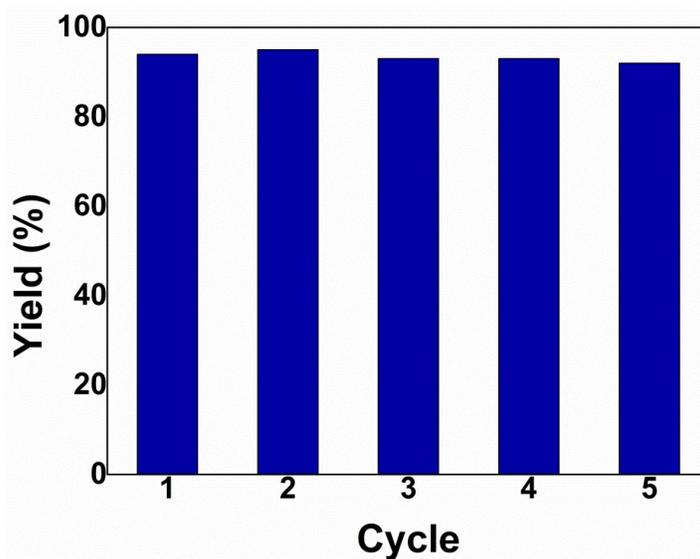
**Figure S11** Recyclability test of Ag@RB-POP. Reaction conditions: **1a**, 0.5 mmol; Ag@RB-POP, 20 mg (Ag was 0.01 mol% based on **1a**); DBU, 0.5 mmol; CO<sub>2</sub> 1 MPa; CH<sub>3</sub>CN, 2 mL; 30 °C, 12 h. <sup>b</sup> Determined by <sup>1</sup>H NMR (CDCl<sub>3</sub>, 400 MHz) using mesitylene as an internal standard.
