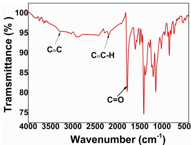
**Figure S1** FTIR spectrum of **RB-POP**. The spectrum was recorded as KBr pellets.
