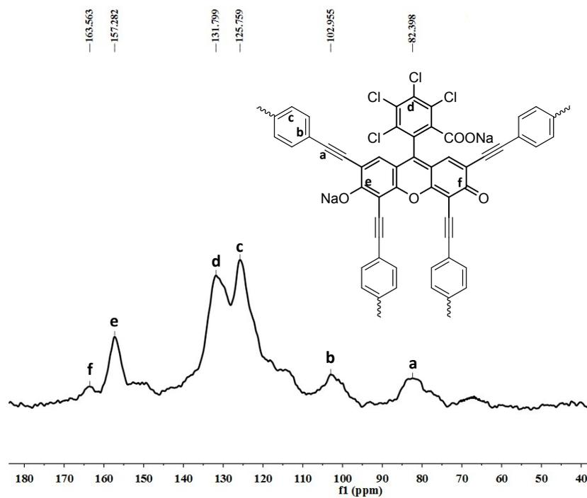
**Figure S2** CP/MAS  $^{13}\text{C}$  NMR spectrum for **RB-POP**.
