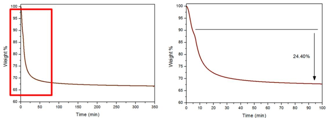
**Figure S27.** Isothermal Thermogravimetric Analysis of NBoc-RhMOP at 150 °C, highlighting the stability of the material after the weight loss attributed to the thermolabile deprotection of 24 Boc groups.
