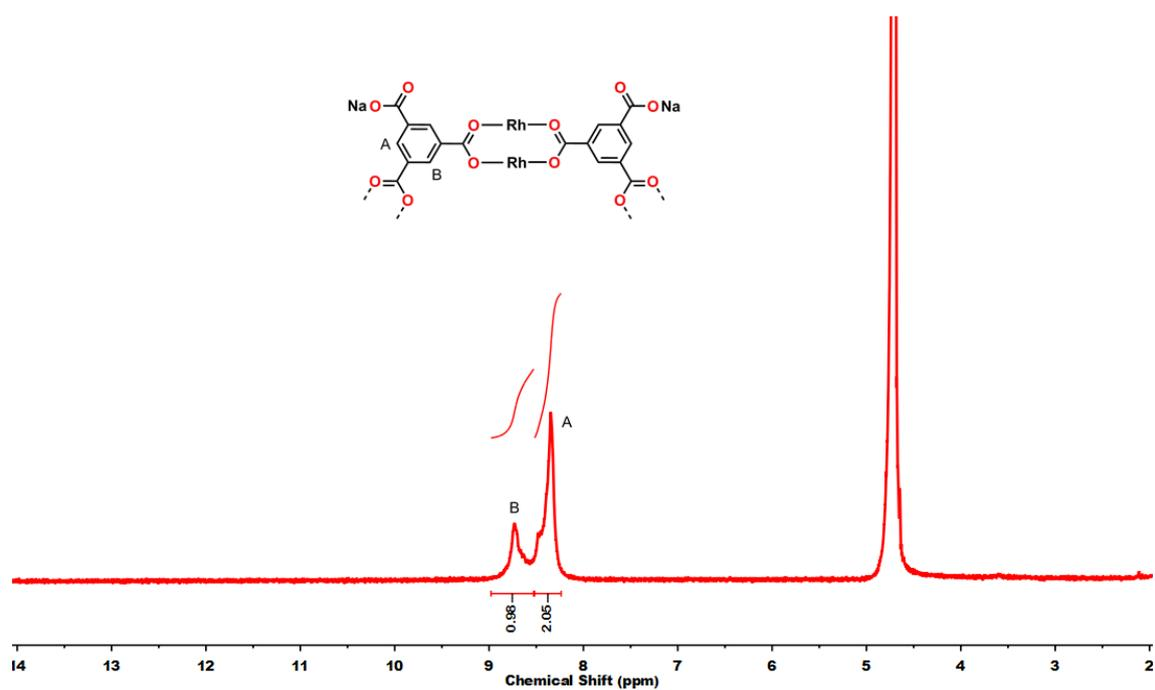
**Figure S16.**  $^1\text{H}$  NMR spectrum of COONa-RhMOP in  $\text{D}_2\text{O}/\text{NaOD}$  (24 mol. eq. vs MOP) dissolved for 7 days.
