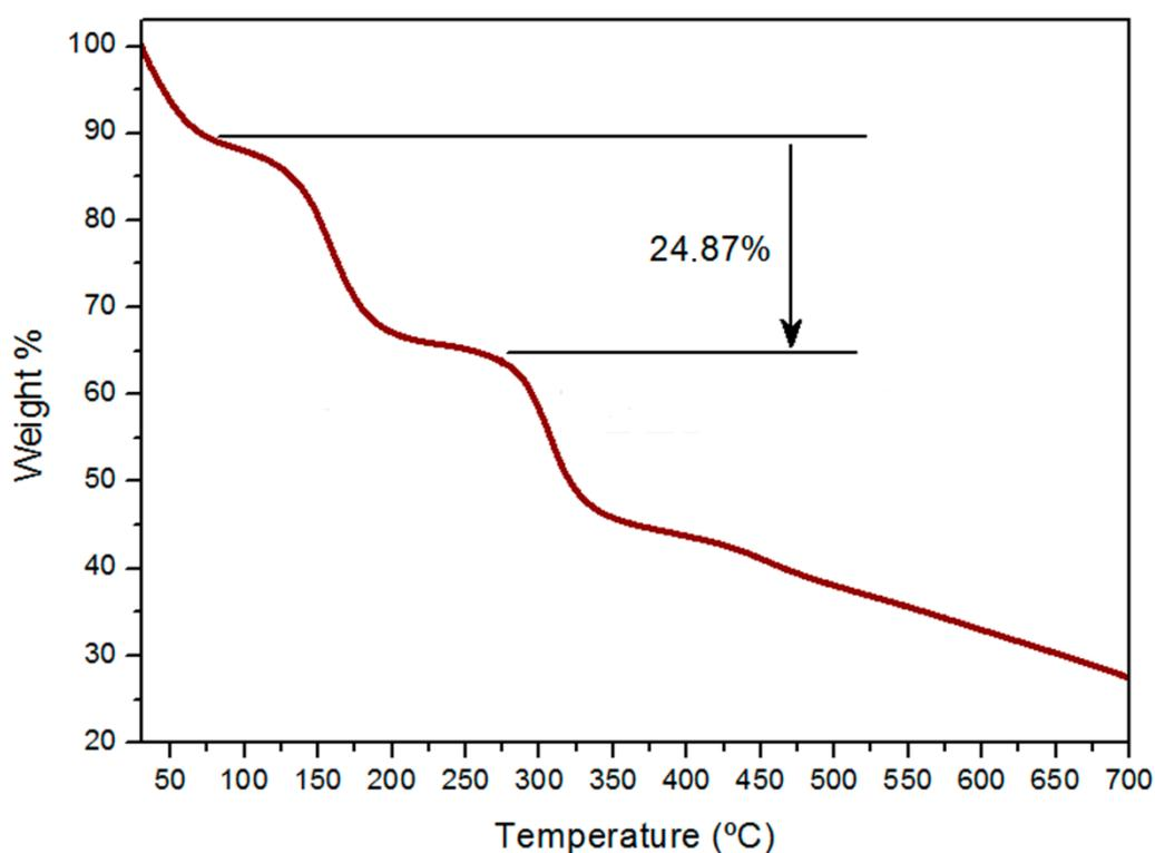
**Figure S26.** Thermogravimetric Analysis of NBoc-RhMOP, highlighting the 24.87% weight loss attributed to the thermolabile deprotection of 24 Boc groups (Calculated weight loss 25.1%).
