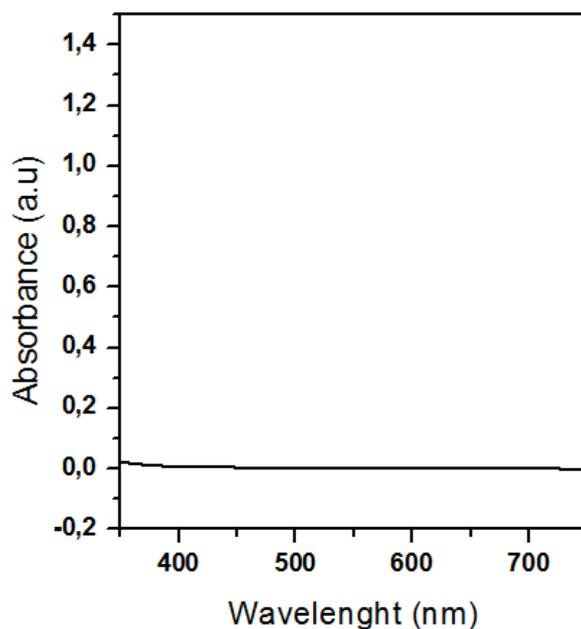
**Figure S23.** UV-Vis spectrum of the DCM:TFA supernatant after the deprotection step. The absence of absorption bands at the Rh-Rh expected region (594 nm) confirms that no  $\text{Rh}_2(\text{TFA})_4$  byproduct is being formed.
