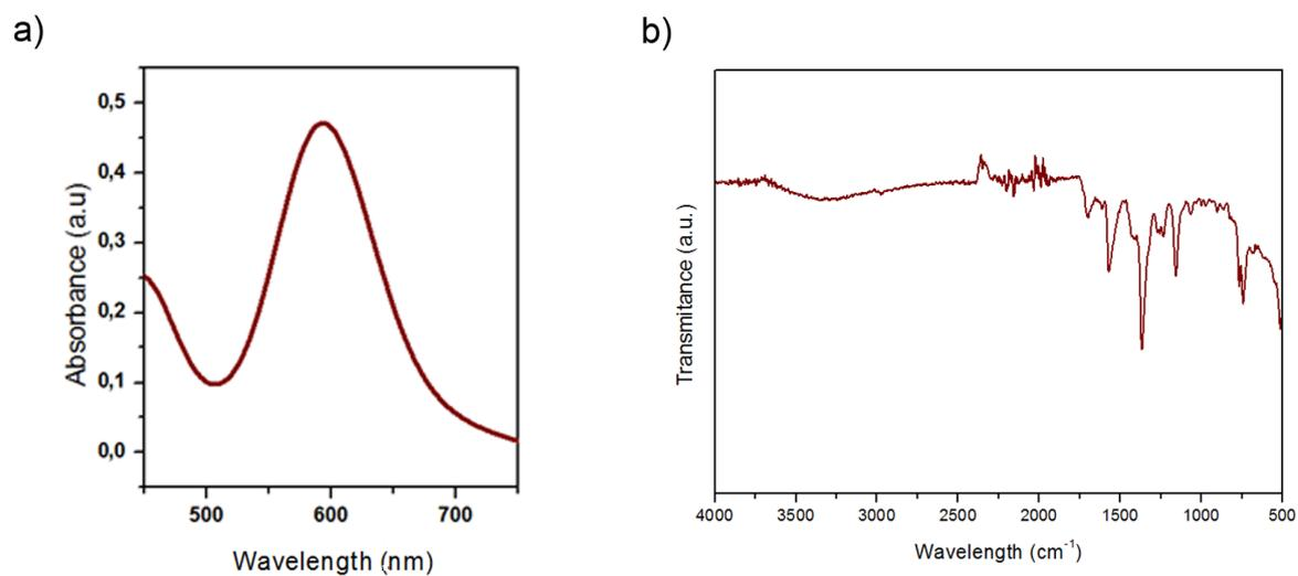
**Figure S21.** a) UV-Vis spectrum of NBoc-RhMOP in Acetone (0.30 mM).  $\lambda_{\text{max}}$  is centered at 594 nm. b) FTIR spectrum of NBoc-RhMOP.
