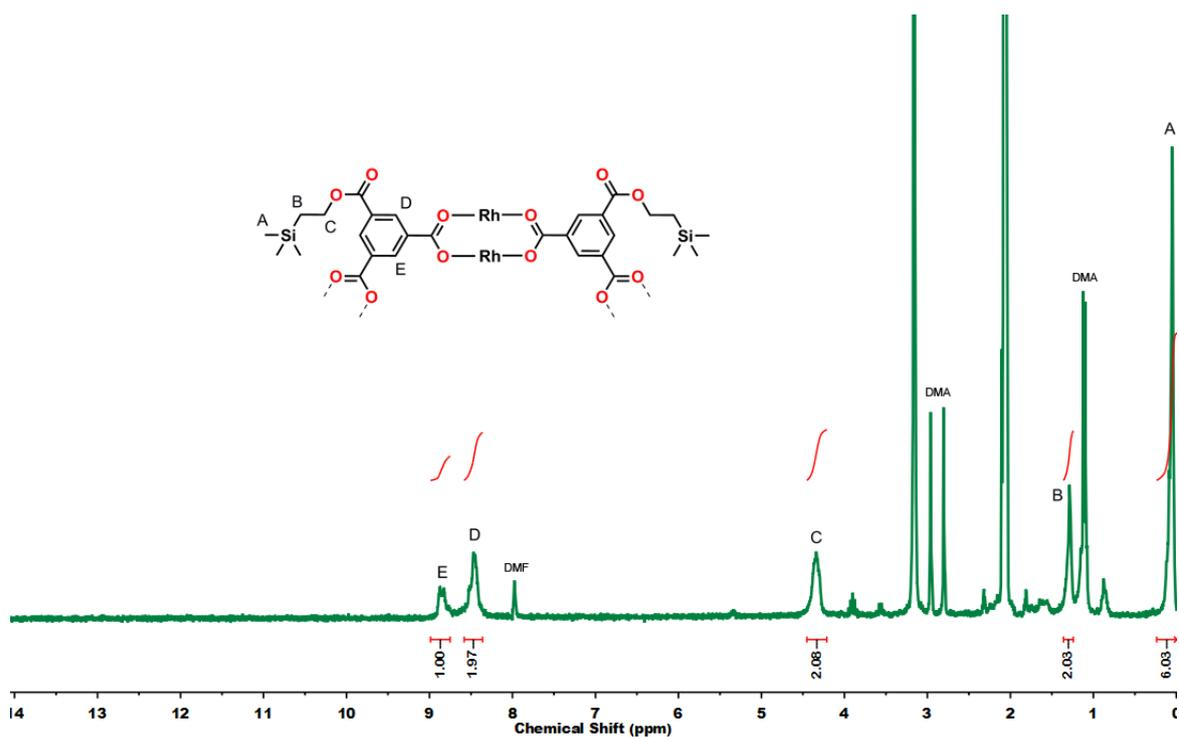
**Figure S7.**  $^1\text{H}$  NMR spectrum of COOTSE-RhMOP in acetone- $d_6$ . TMS signal (A) is not fully integrable due to the presence of TMS as an internal reference in deuterated solvents. The chemical shift of the signals is shifted compared with the free linker. No residual  $\text{H}_2\text{btc}$ -COOTSE peaks are observed.
