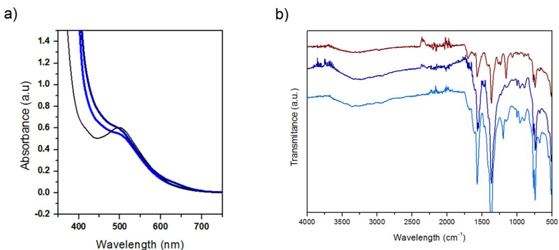
**Figure S28.** a) UV-Vis spectrum of NH<sub>2</sub>-RhMOP deprotected by thermolabile (navy) or TFA (blue) in DMSO (0.30 mM).  $\lambda_{\text{max}}$  is centered at 501 nm. Rh<sub>2</sub>(Acetate)<sub>4</sub> in DMSO (0.3 mM) added for reference (Black) to show the strong coordination of DMSO molecules in the axial positions of the paddlewheel.<sup>2,3</sup> b) FTIR spectra of NH<sub>2</sub>-RhMOP, deprotected by thermolabile (navy) or TFA (blue) in comparison with NBoc-RhMOP (wine).
