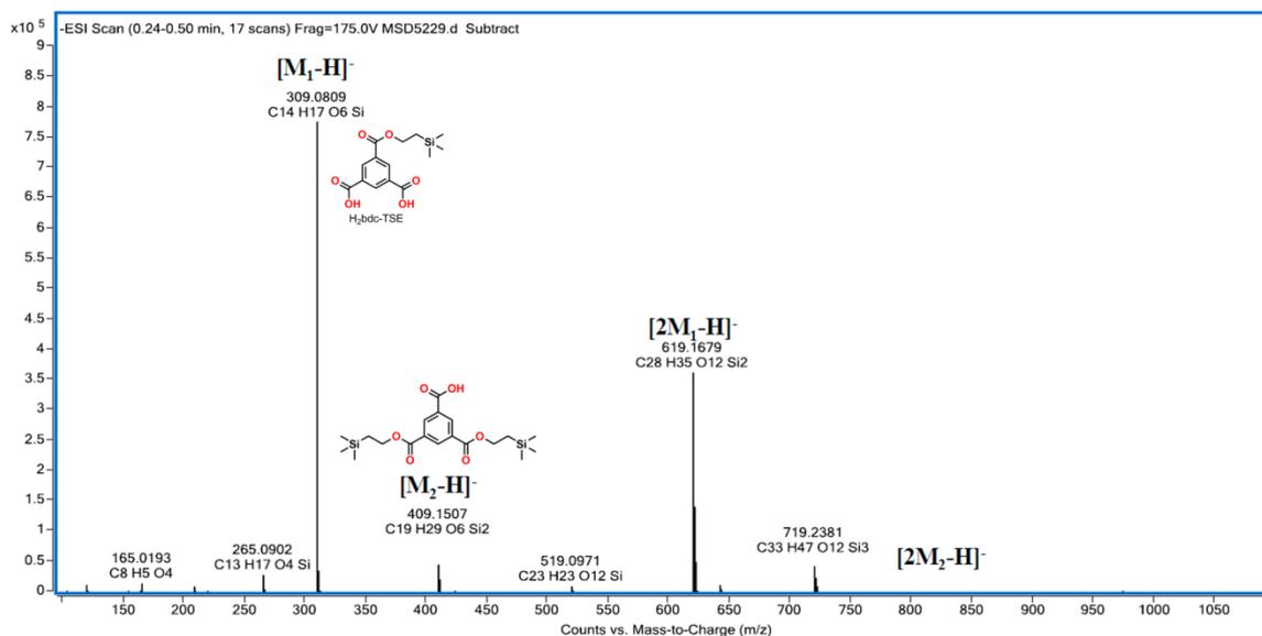
**Figure S5.** ESI-MS spectrum of H<sub>2</sub>btc-COOTSE. Residual traces (<5%) of mono-protected linker can be observed.
