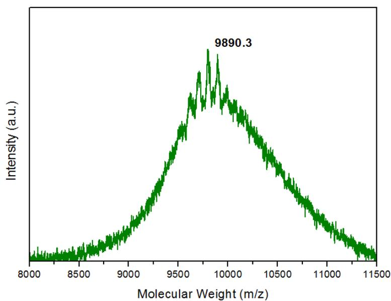
**Figure S6.** MALDI-TOF spectra of COOTSE-RhMOP in acetone. The weight corresponding to the formula [Rh<sub>24</sub>(TSE-bdc)<sub>24</sub> + H<sup>+</sup>]<sup>+</sup> has been highlighted: expected = 9891.5; found = 9890.3.
