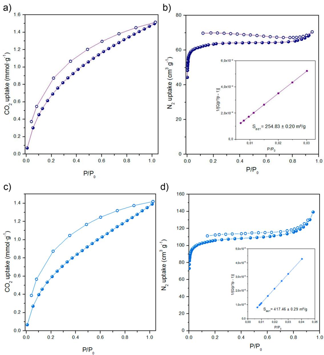
**Figure S30.** a,c) CO<sub>2</sub> adsorption isotherm at 295 K and b,d) N<sub>2</sub> adsorption isotherm at 77 K with BET linear fit of Thermolabile-deprotected NH<sub>2</sub>-RhMOP (navy) and TFA-deprotected NH<sub>2</sub>-RhMOP (blue).
