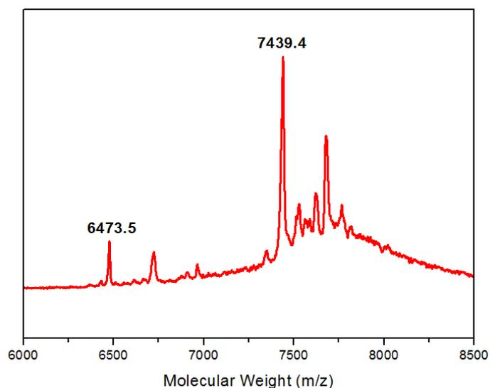
**Figure S10.** MALDI-TOF spectra of COOH-RhMOP in DMF. The weight corresponding to the formula  $[\text{Rh}_{24}(\text{COOH-bdc})_{24} + \text{H}^+]^+$  has been highlighted: expected = 7441.5; found = 7439.4. The weight corresponding to the formula  $[\text{Rh}_{24}(\text{COOH-bdc})_{24} - 22\text{CO}_2 + \text{H}^+]^+$  has been highlighted: expected = 6473.3; found = 6473.5.
