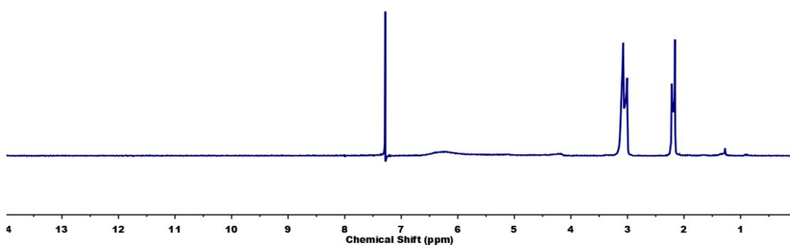
**Figure S22.**  $^1\text{H}$  NMR of the evaporated DCM:TFA supernatant in  $\text{DMSO-}d_6$  after the deprotection step. No  $\text{H}_2\text{bdc-NH}_2$  signals can be observed, discarding any linker exchange process or partial degradation of the scaffold. DMA signals, coming from the MOP inner solvation, can be observed.
