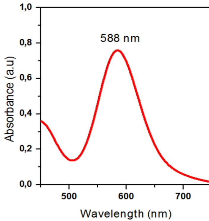
Figure S17. UV-Vis spectrum of COONa-RhMOP in H<sub>2</sub>O (0.30 mM).  $\lambda_{\text{max}}$  is centered at 588 nm.
