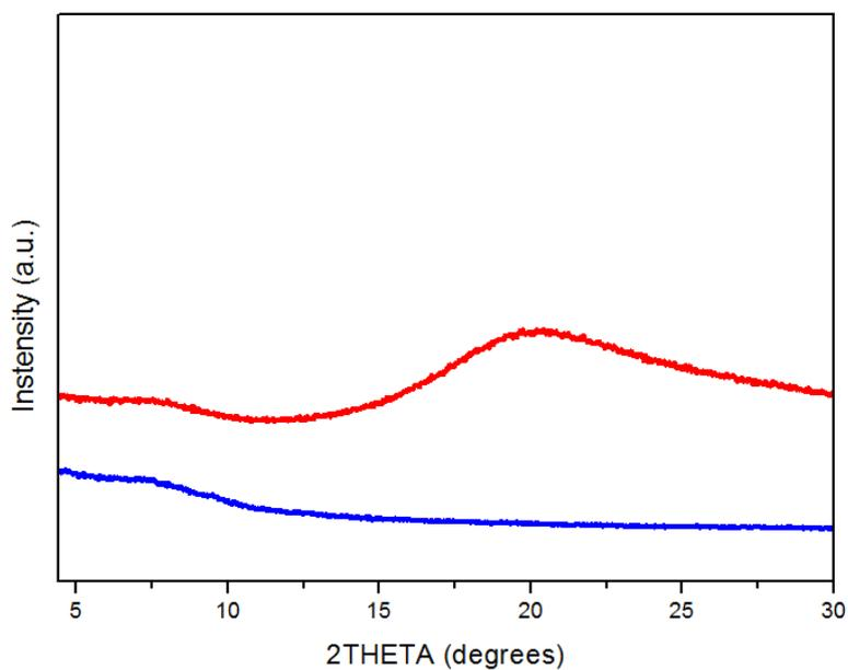
**Figure S1.** PXRD patterns of BT\_Rh-NH<sub>2</sub>bdc (blue) and BT\_Rhbtc (red).
