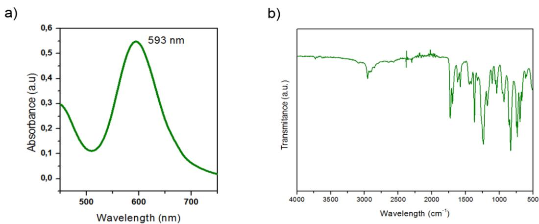
**Figure S8.** a) UV-Vis spectrum of COOTSE-RhMOP in acetone (0.30 mM).  $\lambda_{\text{max}}$  is centered at 593 nm. b) FTIR spectrum of COOTSE-RhMOP.
