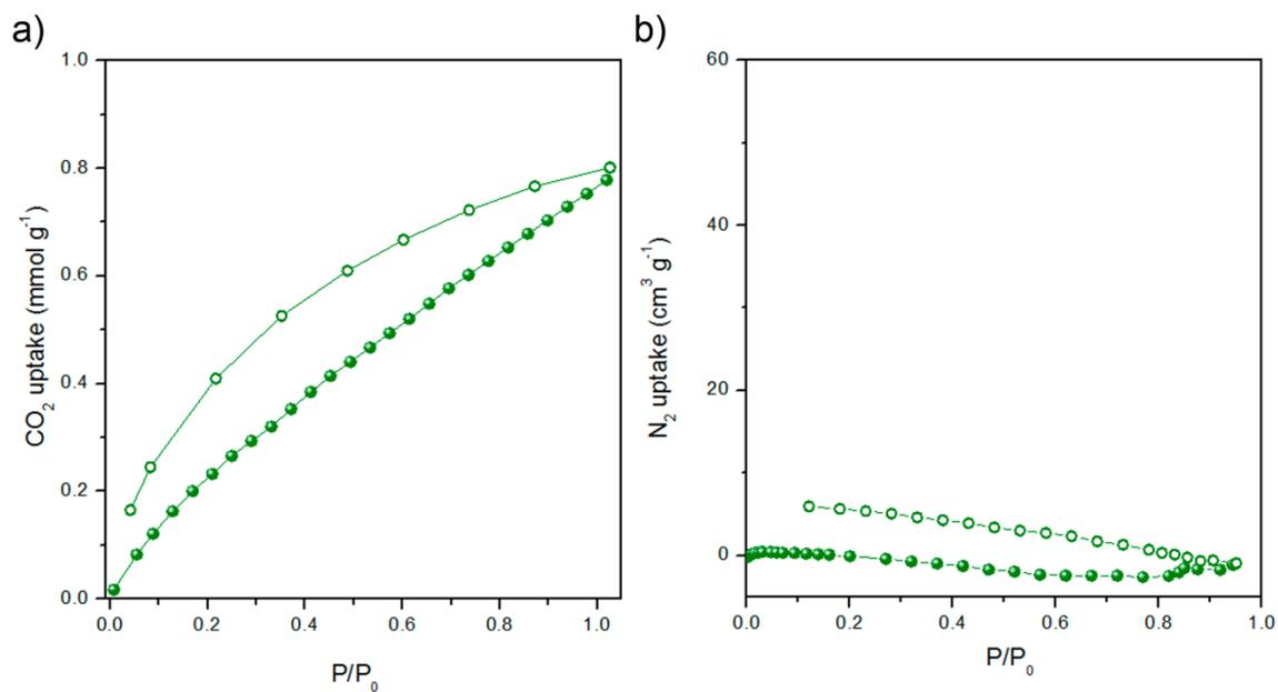
**Figure S11.** a) CO<sub>2</sub> adsorption isotherm at 295 K and b) N<sub>2</sub> adsorption isotherm at 77 K with BET linear fit of COOTSE-RhMOP
