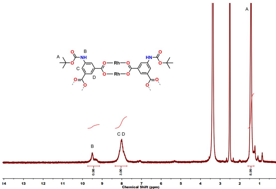
**Figure S20.**  $^1\text{H}$  NMR spectrum of NBoc-RhMOP in  $\text{DMSO-}d_6$ . The chemical shift of the signals is shifted compared with the free linker. No residual  $\text{H}_2\text{bdc-NBoc}$  peaks are observed.
