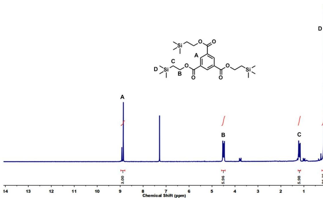
**Figure S3.**  $^1\text{H}$  NMR spectrum of the tri-protected intermediate  $\text{btc-COOTSE}_3$  in  $\text{CDCl}_3$ . TMS signal (D) is not fully integrable due to the presence of TMS as an internal reference in deuterated solvents.
