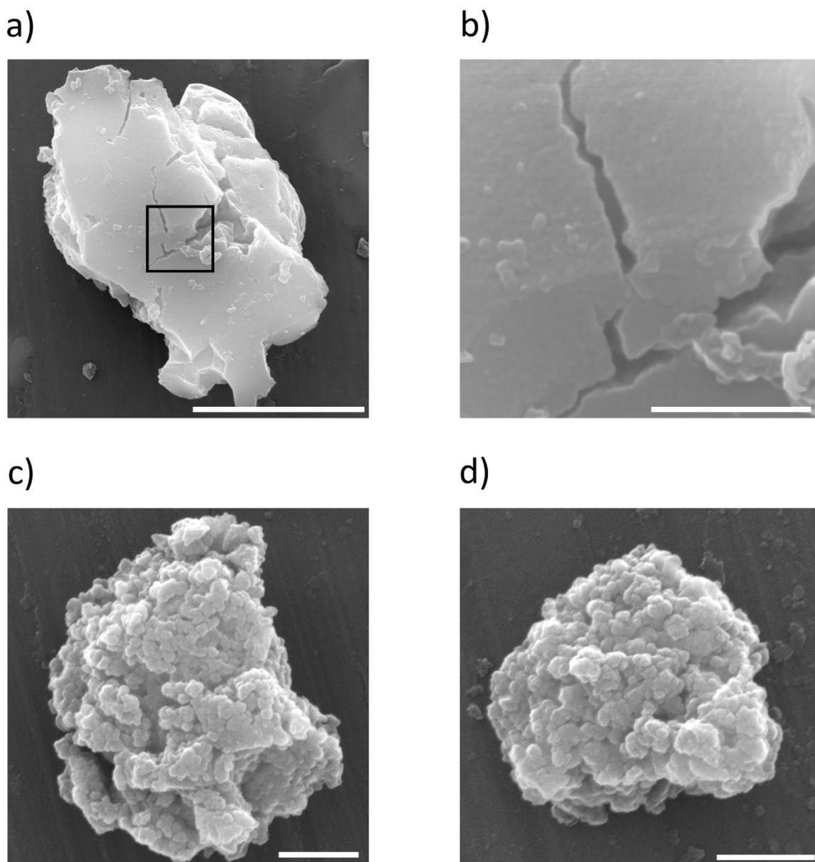
**Figure S31.** a,b) FESEM images of the NH<sub>2</sub>-RhMOP obtained by the thermal treatment of the NBoc-RhMOP. b) High magnification image of the highlighted area in a). c,d) FESEM images of the NH<sub>2</sub>-MOP obtained after deprotecting the NBoc-RhMOP with TFA. Scale bars = 5 μm (a), 1 μm (b), and 500 nm (c, d).
