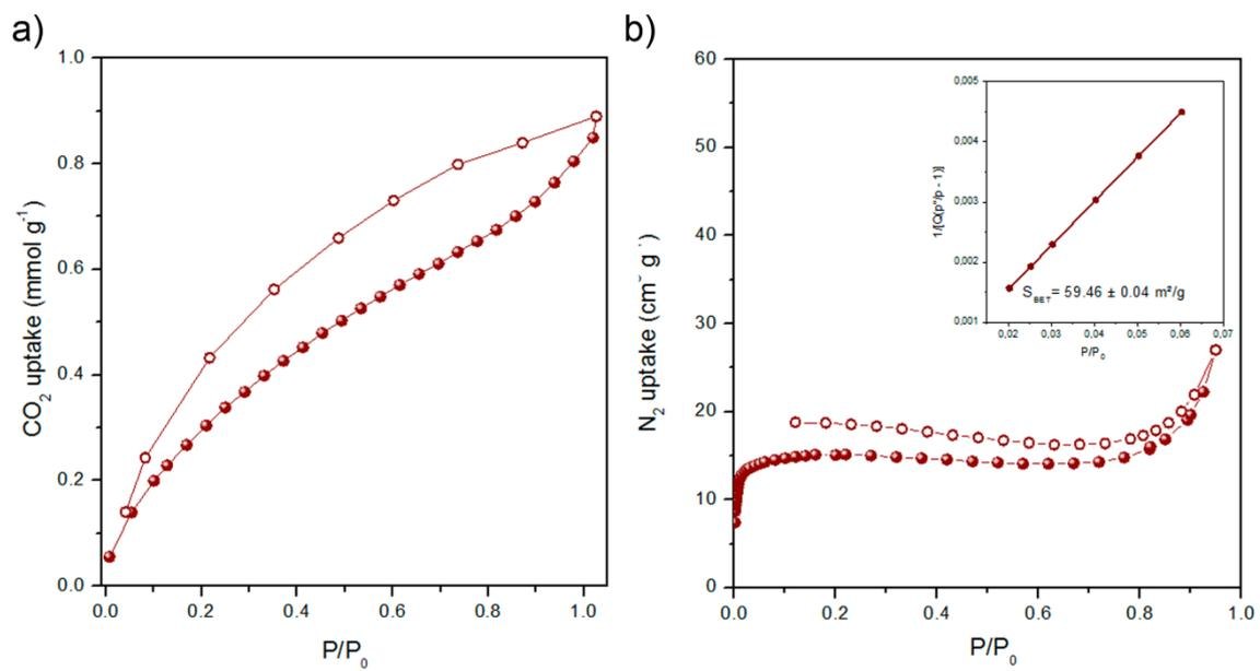
**Figure S29.** a) CO<sub>2</sub> adsorption isotherm at 295 K and b) N<sub>2</sub> adsorption isotherm at 77 K with BET linear fit of NBoc-RhMOP
