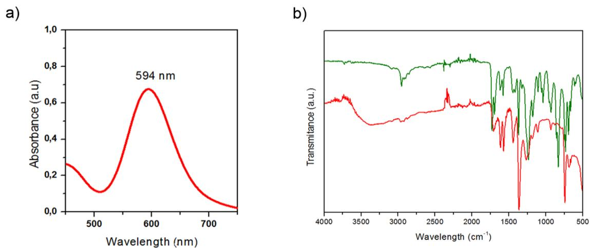
**Figure S13.** a) UV-Vis spectrum of COOH-RhMOP in DMF (0.30 mM).  $\lambda_{\text{max}}$  is centered at 594 nm. b) FTIR spectra of COOH-RhMOP (red) in comparison with COOTSE-RhMOP (green).
