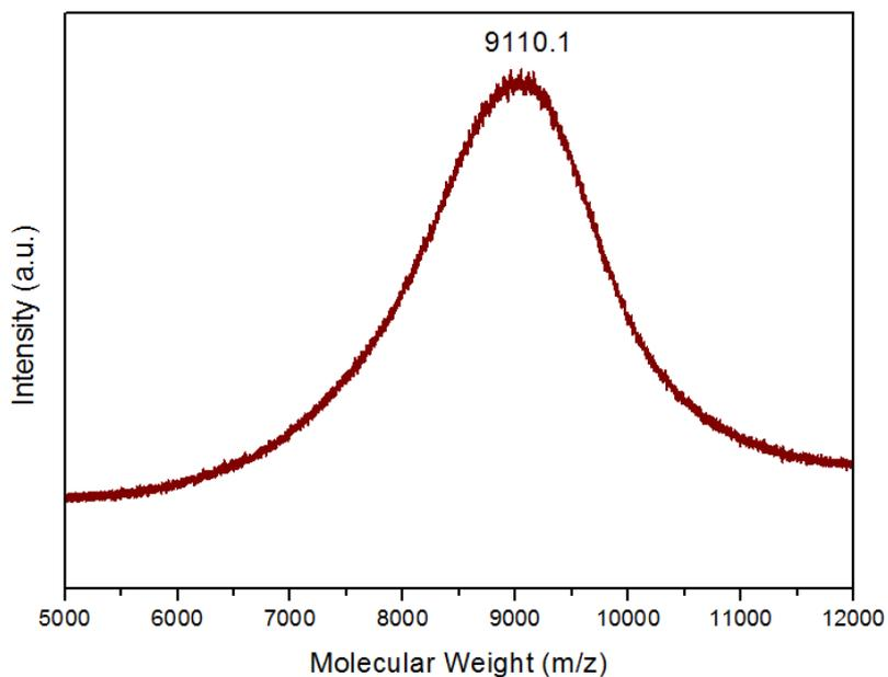
**Figure S19.** MALDI-TOF spectra of NBoc-RhMOP in Acetone. The weight corresponding to the formula  $[\text{Rh}_{24}(\text{NBoc-bdc})_{24} - \text{Nbc} + \text{H}^+]^+ + 2\text{H}_2\text{O}$  has been highlighted: expected = 9105.4; found = 9110.1.
