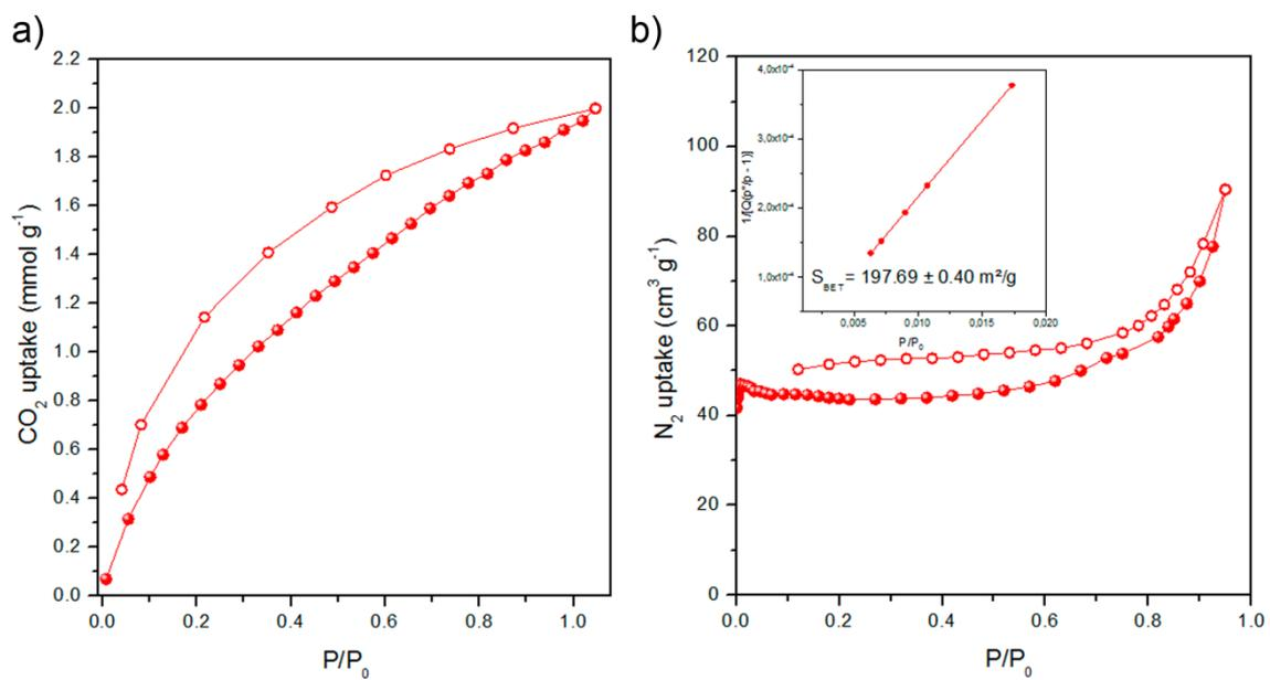
**Figure S12.** a) CO<sub>2</sub> adsorption isotherm at 295 K and b) N<sub>2</sub> adsorption isotherm at 77 K with BET linear fit of COOH-RhMOP
