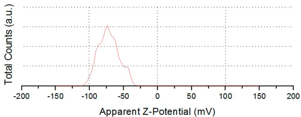
**Figure S14.** Z-Potential measurements of COONa-RhMOP in basic H<sub>2</sub>O, confirming a charged specie.
