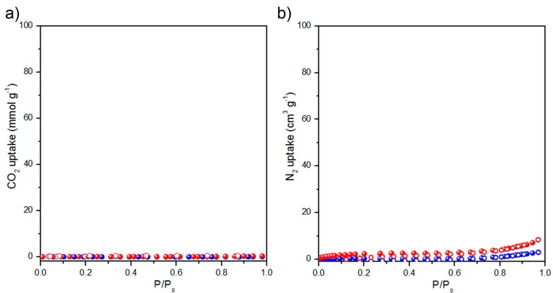
**Figure S2.** a) CO<sub>2</sub> adsorption isotherm at 295 K and b) N<sub>2</sub> adsorption isotherm at 77 K with BET linear fit of BT\_Rh-NH<sub>2</sub>bdc (blue) and BT\_Rhbtc (red).
