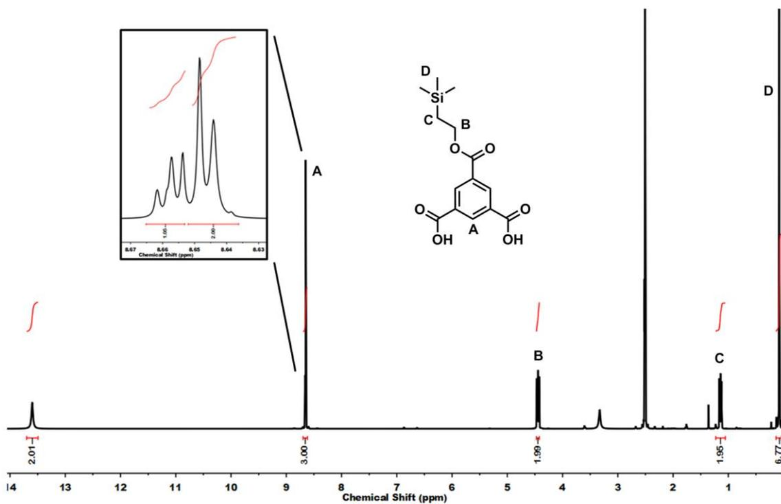
**Figure S4.**  $^1\text{H}$  NMR spectrum of the mono-protected linker  $\text{H}_2\text{btc-COOTSE}$  in  $\text{DMSO-}d_6$ . TMS signal (D) is not fully integrable due to the presence of TMS as an internal reference in deuterated solvents.
