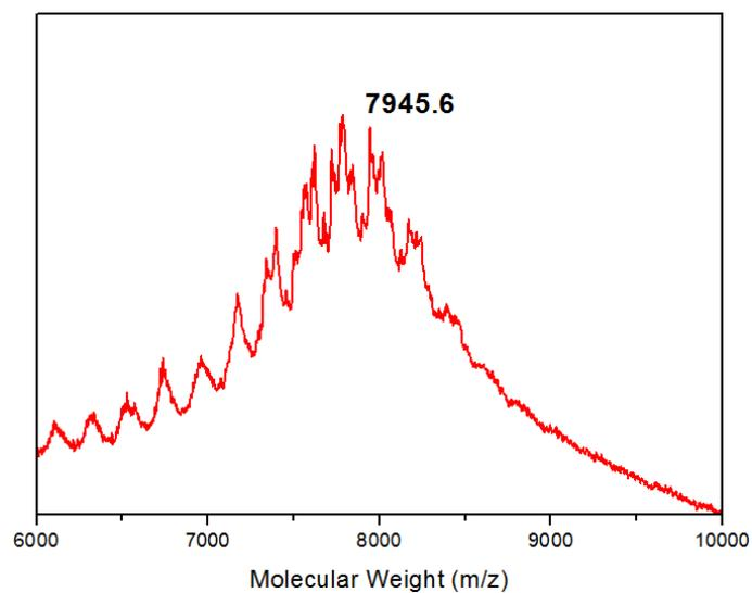
**Figure S15.** MALDI-TOF spectrum of COONa-RhMOP. The weight corresponding to the formula  $[\text{Rh}_{24}(\text{COONa-bdc})_{24} - 2\text{Na}^+ + \text{H}^+]^-$  has been highlighted: expected = 7947; found = 7945.6.
