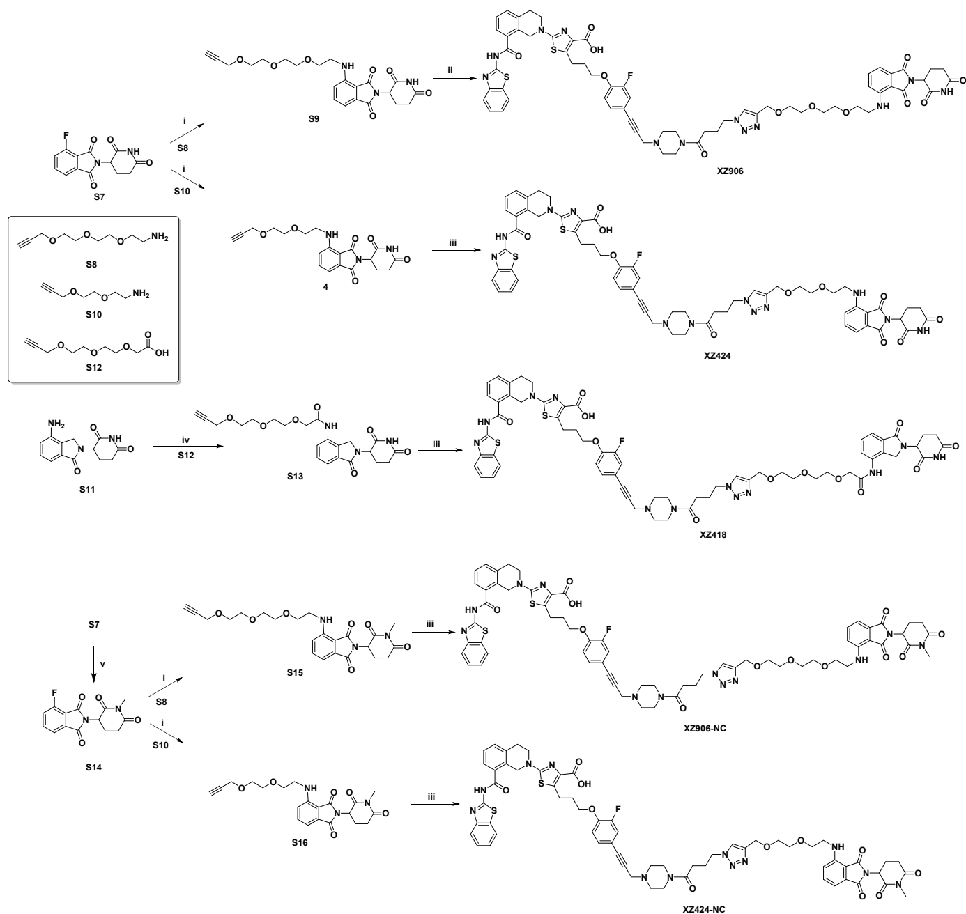
Scheme S2. Synthetic route for BCL-X L PROTACs. Reagents and conditions: (i) DIPEA, DMF, 90 °C. (ii) 3 , CuSO 4 ·5H 2 O, sodium L-ascorbate, t BuOH, H 2 O, 65 °C. (iii) a) 6 , CuSO 4 ·5H 2 O, sodium L-ascorbate, t BuOH, THF, H 2 O, 55 °C; b) HCl in 1,4-dioxane, DCM, MeOH. (iv) HATU, DIPEA, DCM. (v) Iodomethane, t BuOK, DMSO.
