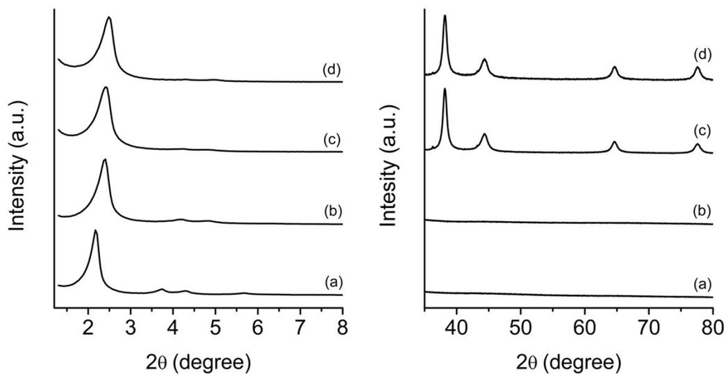
**Figure SI-2.** PXRD patterns at low angles (left) and at high angles (right) of: (a) as-synthesized MSNPs, (b) calcined MSNPs, (c) starting Janus Au-MSNPs (**S0**) and (d) gated nanoparticles (**S1**).
