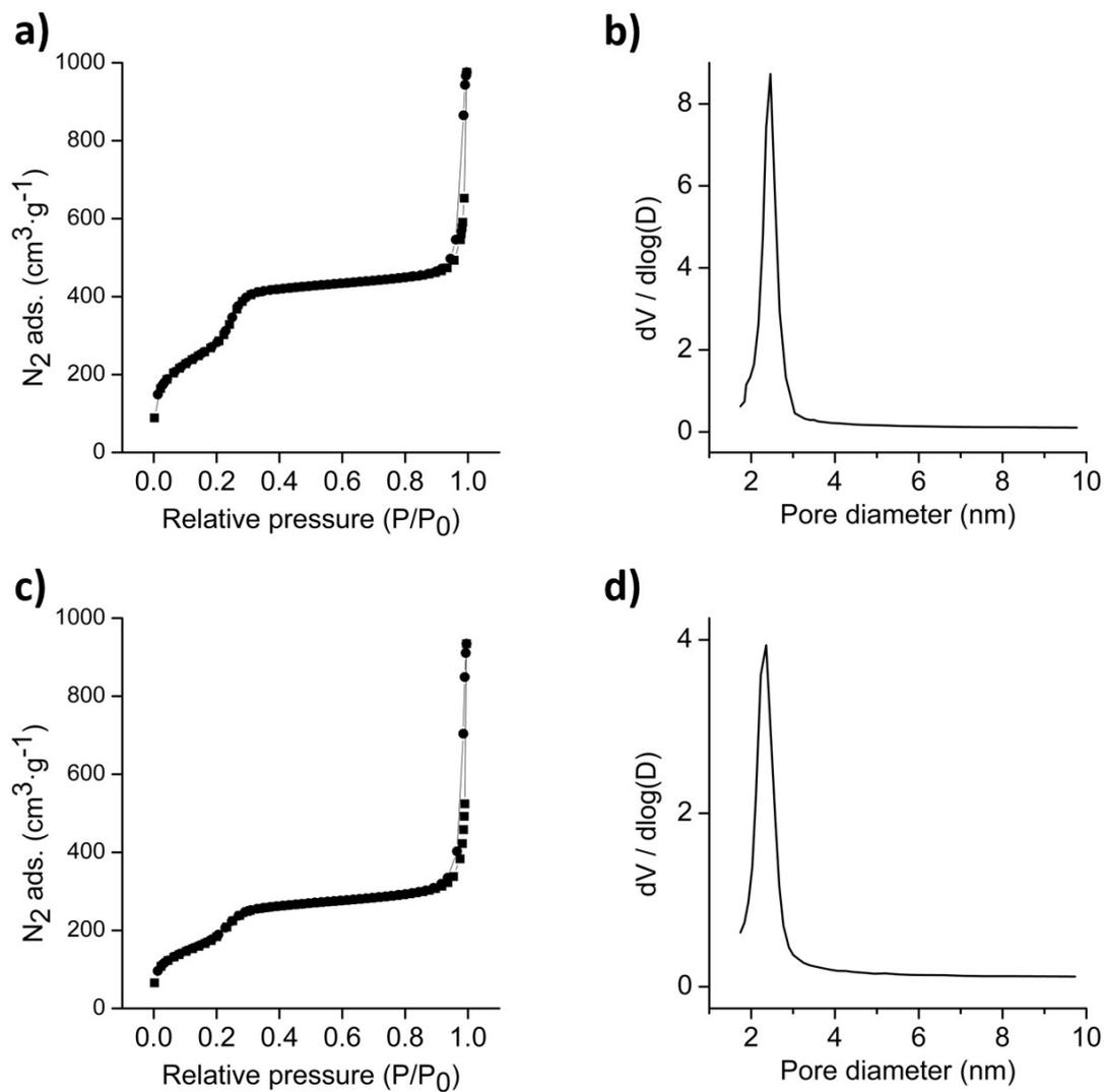
**Figure SI-4.** a) N<sub>2</sub> adsorption-desorption isotherms for the calcined **MSNPs** and (b) corresponding pore diameter distribution. c) N<sub>2</sub> adsorption-desorption isotherms for the Janus Au-MSNPs (**S0**) and (d) corresponding pore diameter distribution. Pore diameter distributions were determined by applying the BJH model on the adsorption branch of the isotherm for P/P<sub>0</sub> < 0.8, which is associated with the surfactant generated mesopores.
