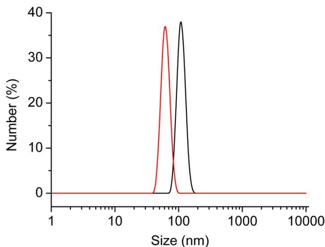
**Figure SI-6.** Apparent hydrodynamic size distribution of nanobots (**S1<sub>cat</sub>**) before (black) and after the addition (red) of fuel (0.3% v/v H<sub>2</sub>O<sub>2</sub>) as measured by DLS.
