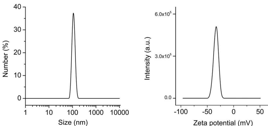
**Figure SI-5.** Hydrodynamic diameter and zeta potential distributions of the nanodevice (**S1<sub>cat</sub>**) determined by DLS.
