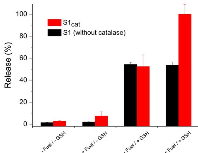
**Figure SI-7.** Cargo release from nanoparticles **S1** (without the catalase) and nanobots **S1<sub>cat</sub>** in phosphate buffer (10 mM, pH 7.5) after 60 min under different conditions: (i) control (no fuel and no GSH), (ii) presence of H<sub>2</sub>O<sub>2</sub> (0.3%), (iii) presence of GSH (10 mM), and (iv) presence of GSH (10 mM) and H<sub>2</sub>O<sub>2</sub> (0.3%). Error bars represent s. d. from three independent experiments.
