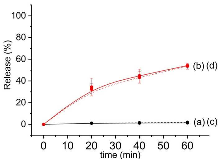
**Figure SI-8.** Cargo release from nanoparticles **S1** (without the catalase) as a function of time in phosphate buffer (pH 7.5) under different conditions: (a, continuous line) control (no fuel and no GSH), (b, continuous line) presence of GSH (10 mM) and no fuel, (c, dashed line) presence of fuel (H<sub>2</sub>O<sub>2</sub> 0.3%) and no SGH, and (d, dashed line) presence of GSH (10 mM) and fuel (H<sub>2</sub>O<sub>2</sub> 0.3%). Error bars represent s. d. from three independent experiments.
