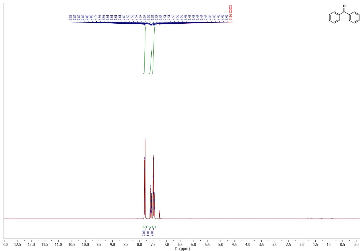
**Figure SI 28.**  $^1\text{H}$ -NMR of benzophenone.
