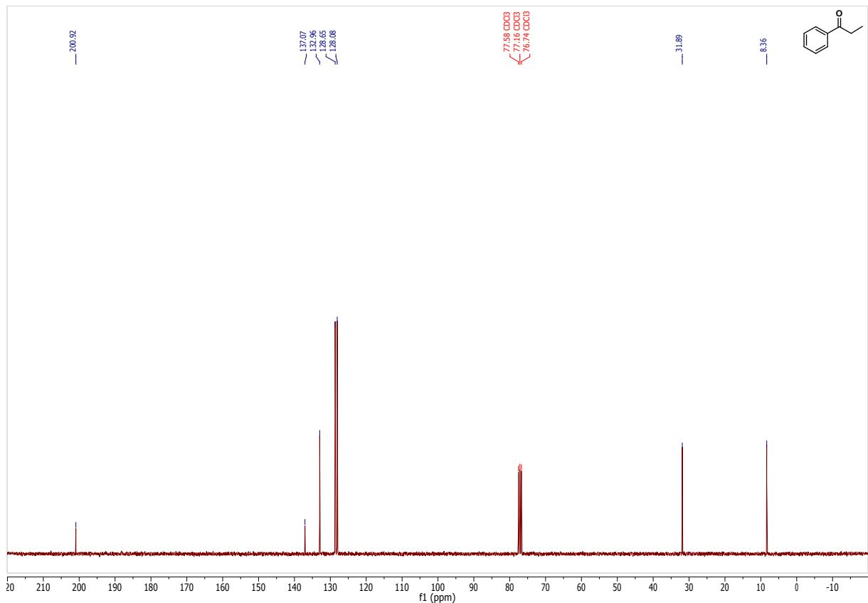
**Figure SI 25.** <sup>13</sup>C-NMR of propiophenone.
