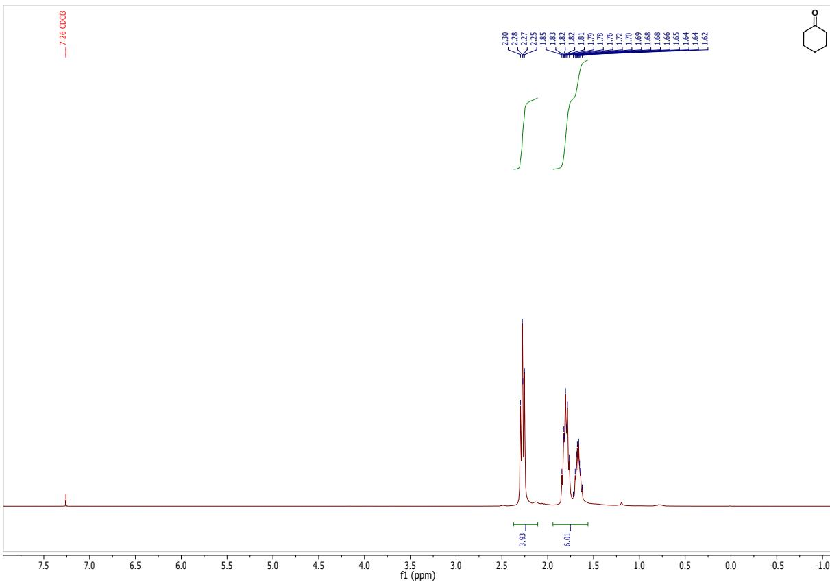
**Figure SI 44.** <sup>1</sup>H-NMR of cyclohexanone.
