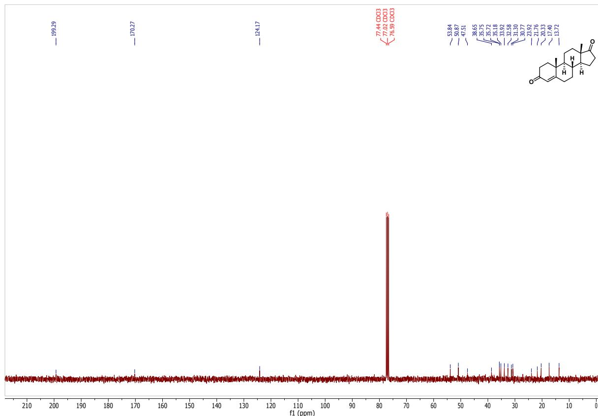
**Figure SI 61.** <sup>13</sup>C-NMR of androstenedione.
