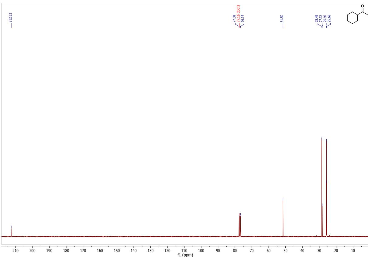
**Figure SI 43.** <sup>13</sup>C-NMR of cyclohexylmethylketone.
