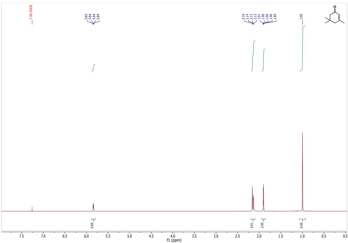
**Figure SI 48.**  $^1\text{H}$ -NMR of 3,5,5-trimethylcyclohex-2-en-1-one.
