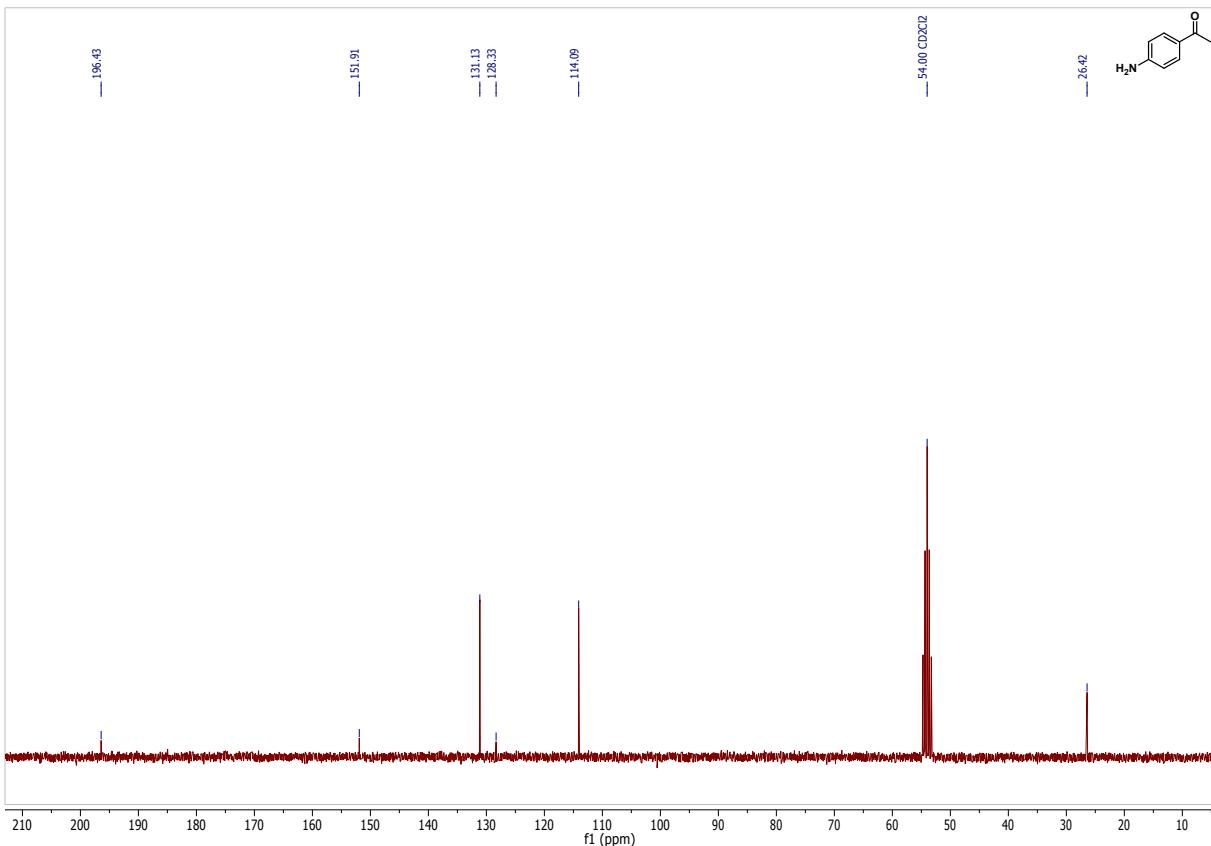
**Figure SI 21.**  $^{13}\text{C}$ -NMR of 1-(4-aminophenyl)ethanone.
