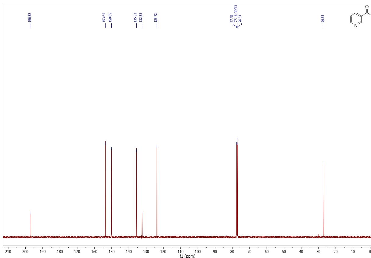
**Figure SI 37.**  $^{13}\text{C}$ -NMR of 1-(pyridine-3-yl)ethan-1-one.
