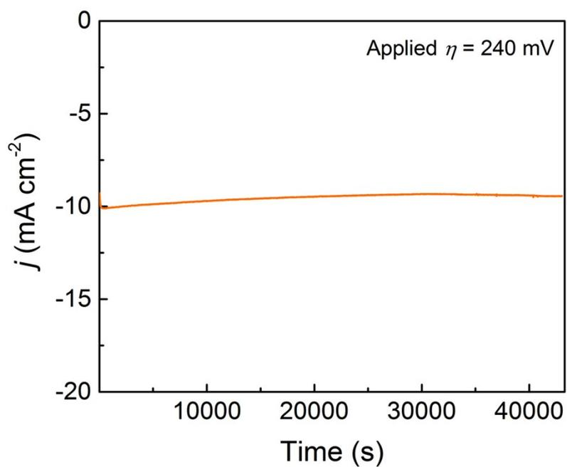
**Figure S5.** The chronoamperometric curve obtained with the NiC-2 drop-casted carbon fiber paper (loading = 0.5 mg cm<sup>-2</sup>) in 1 M PB solution with a constant applied potential of -0.24 V. This test was carried out in a two-compartment electrolytic cell, where the anode and cathode was separated by a piece of glass frit. Pt wire was employed as the counter electrode.
