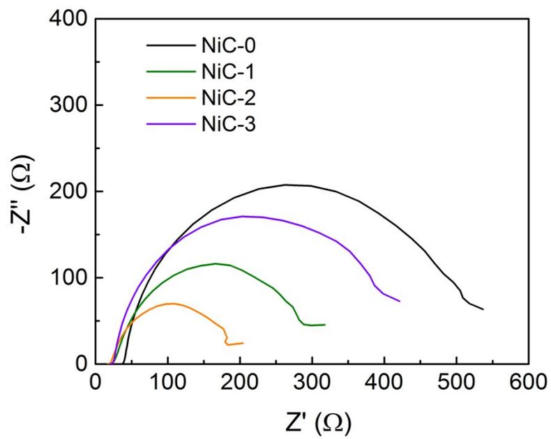
**Figure S4.** EIS spectra of the NiC composites obtained at 150 mV of applied overpotential in the 1 M PB solution.
