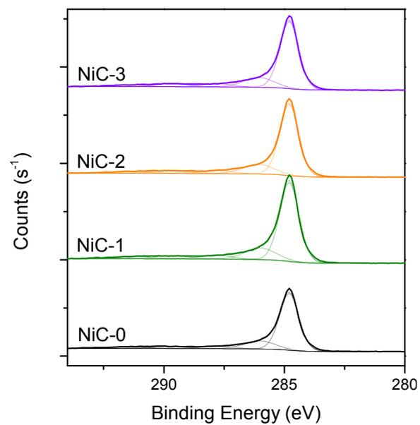
**Figure S3.** C1s XPS results of NiC samples with varying degrees of oxidation (NiC-0 to NiC-3)
