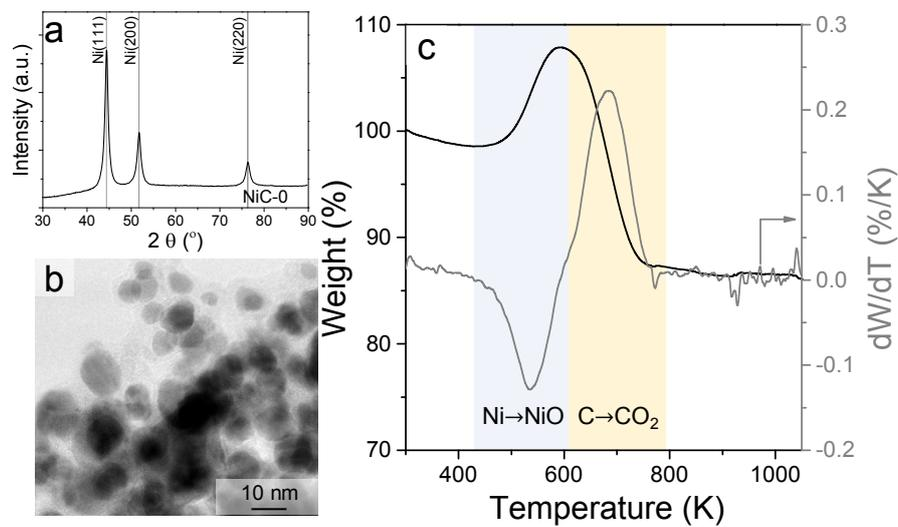
**Figure S1.** (a) XRD, (b) TEM and (c) thermogravimetric analysis (TGA) along with derivative weight ( $dW/dT$ ) curves of the native NiC sample (NiC-0). Shaded regions indicate the zones of weight gain from Ni oxidation and weight loss from C gasification.
