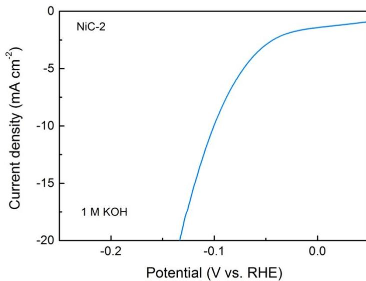
**Figure S7.** HER polarization curve obtained for the NiC-2 composite drop-casted glassy-carbon electrodes in 1 M KOH solution.
