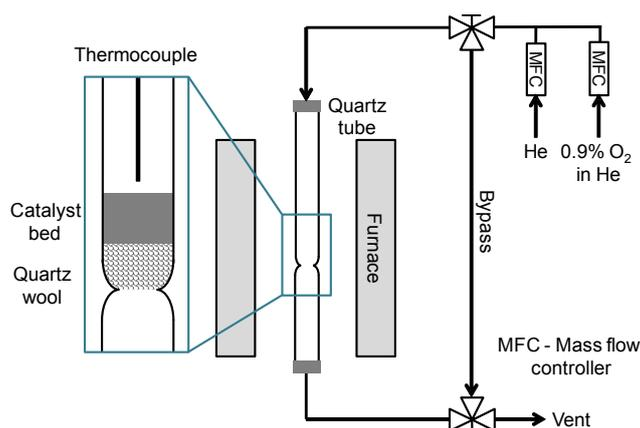
**Scheme S1:** Schematic of thermal oxidation rig utilised to controllably oxidise NiC composites
