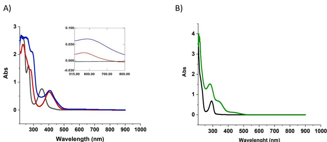
**Figure 1**(A) UV-Vis spectra of salan 1a (black), Cu-salan 8 (red) and VO-salan 9 (Blue). (B) UV-Vis spectra of salan 1b (black) and VO-salan 10 (green)
