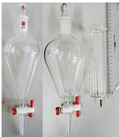
Fig. S4 The original separatory funnel (500 mL), the new separatory funnel (intelligent device, 500 mL), and the glass syringe (from left to right).
