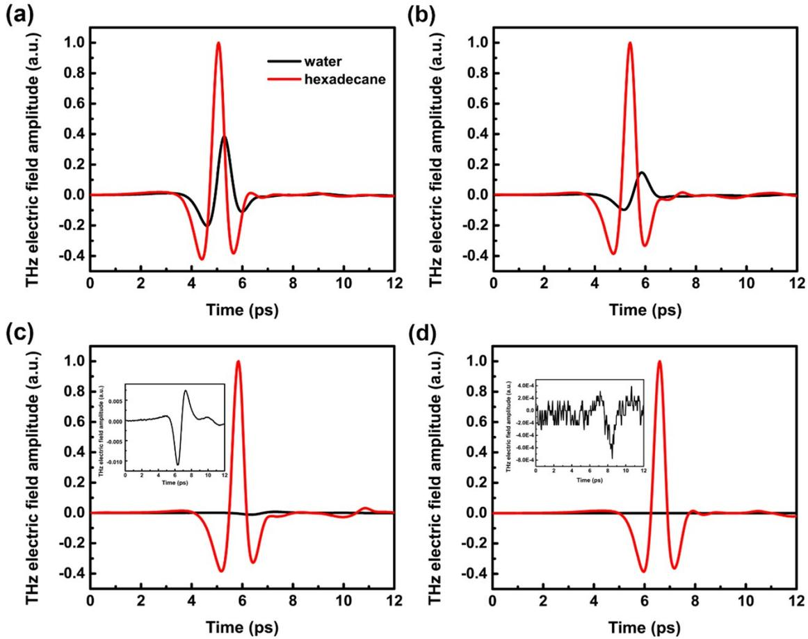
**Figure S2.** The temporal profiles of electric field with Millipore water (black line) and hexadecane (red line) (a) in 0.1 mm cell, (b) in 0.2 mm cell, (c) in 0.5 mm cell, and (d) in 1 mm cell.
