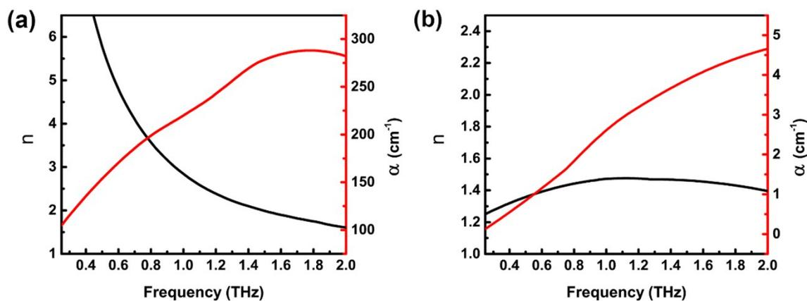
**Figure S4.** Frequency-dependent refractive index (black line) and power absorption coefficient (red line). (a) Millipore water and (b) hexadecane.
