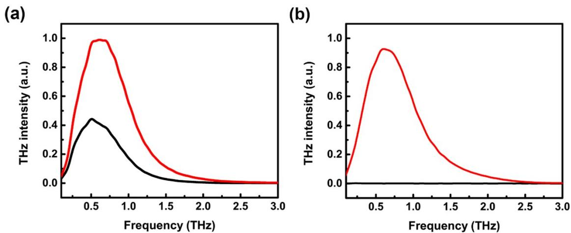
**Figure S3.** Corresponding transmission spectra for the temporal profiles of electric field of Fig. S1(a) and S1(d) with Millipore water (black line) and hexadecane (red line). (a) 0.1 mm cell and (b) 1 mm cell.
