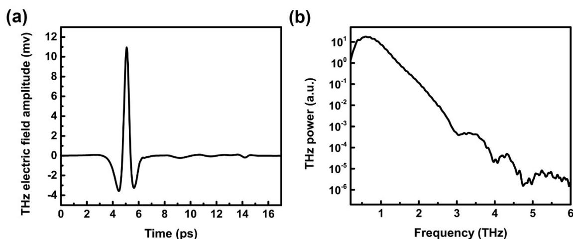
**Figure S1.** (a) Measured wave form of THz pulse under dry air. (b) Power spectrum of the Fourier transform of the pulse shown in (a).
