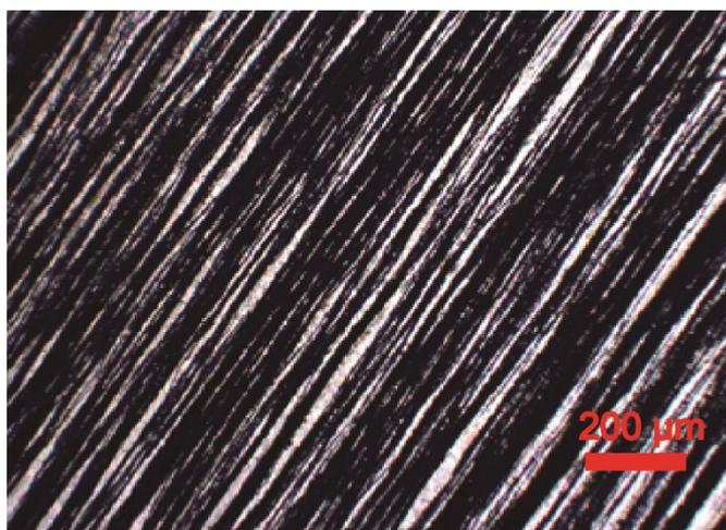
**Fig. S1 Microscopic image of physical-patterning SA/FeP film.** The image indicates that the FeP aligned orderly in SA matrix.
